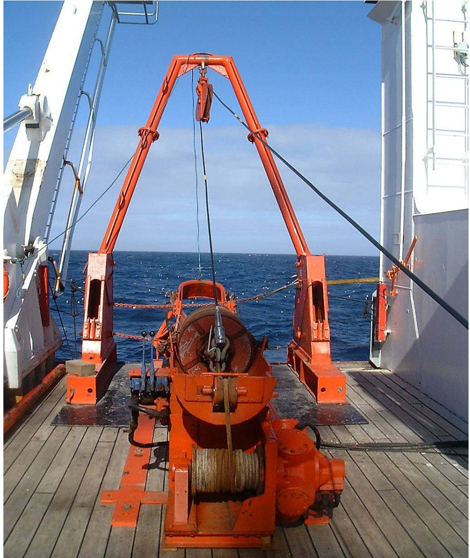
Above Portable 'A' Frame, Launch Chute and launch/recovery winch Below left Freefall Deployment Winch with 5000m Kevlar Cable Below right Deck Layout, Container Workshop, Core Bench, Coring System
