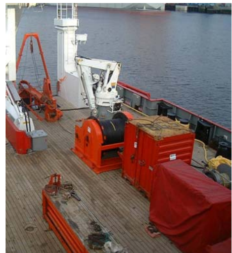
Above Portable 'A' Frame, Launch Chute and launch/recovery winch Below left Freefall Deployment Winch with 5000m Kevlar Cable Below right Deck Layout, Container Workshop, Core Bench, Coring System
