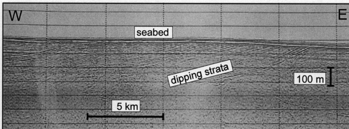
Fig. 7. Part of single-channel seismic line S103 showing dipping strata of the Larsen Basin very near the seabed
