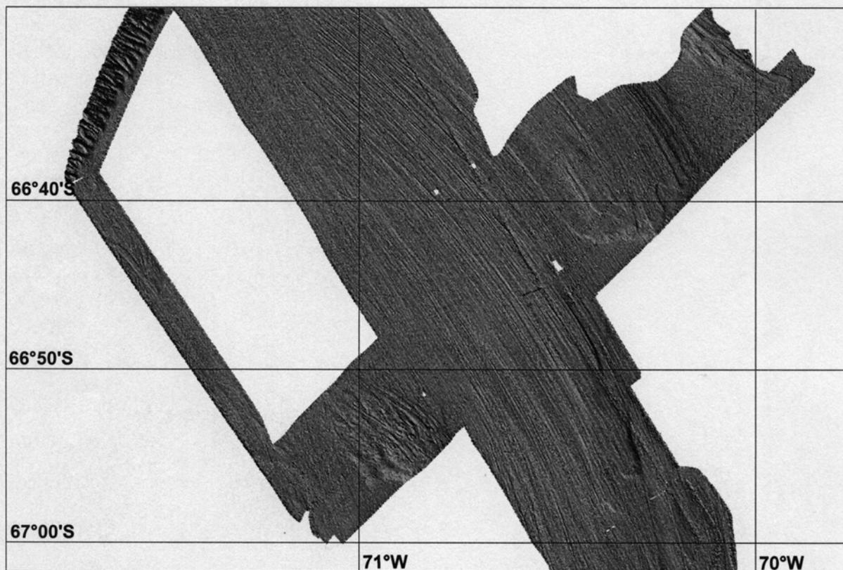
Fig. 11. EM120 sun illumination image of mega-scale glacial lineations in the outer part of Marguerite Trough. Grid cell size 50 m X 50 m.
