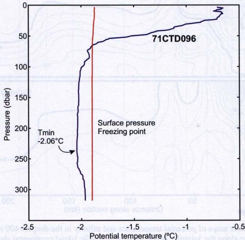
Figure 19. Potential temperature and surface pressure freezing point profiles for station 71CTD096, located at the northern tip of the Larsen C ice front.
