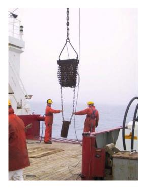
Fig. 9 Dredge deployment from aft deck
