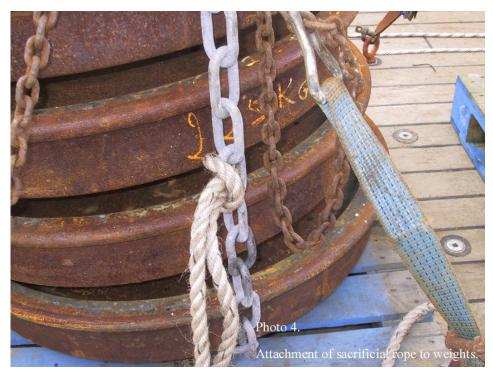
The method of attaching the sacrificial rope, as shown, was used to reduce the risk of the rope being cut by the pressure of the narrow chain link. The long end was threaded through the two deck eyes and over the wood as shown in Photo 5.
