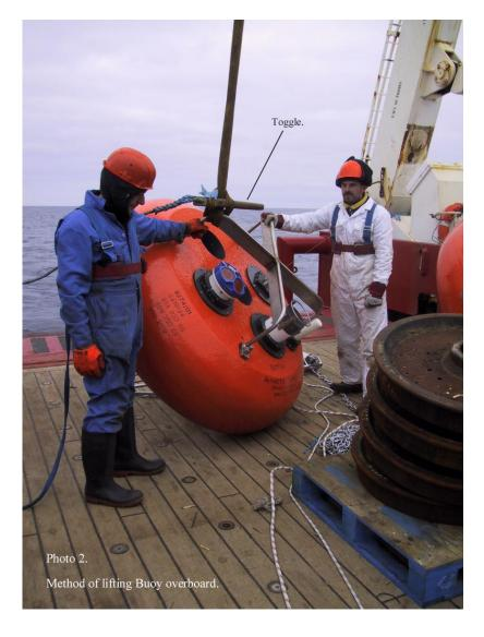
A HEAVING LINE WAS ALSO BE ATTACHED TO THE SHACKLE TO PREVENT THE HEAVY WIRE CRASHING TO THE DECK AS SOON AS THE WEIGHT OF THE BUOY IS RELEASED. Once the buoy was floating the toggle was pulled out, (not all that easy because of the weight of the Gilson wire maintains a tension.)
