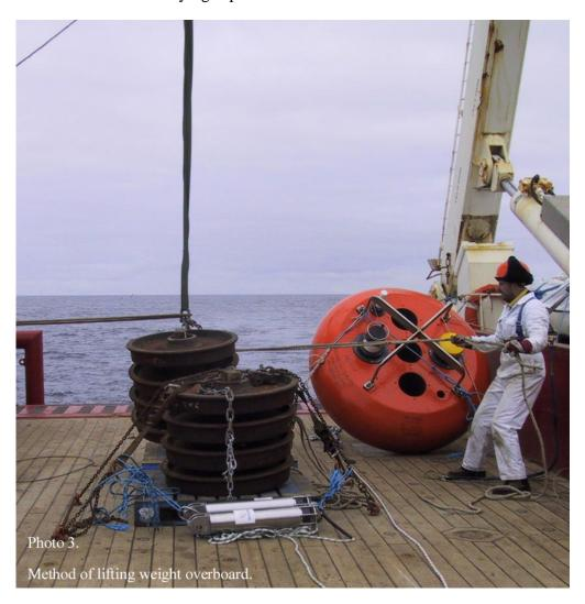
The mooring line was mainly stowed in the plastic crate, having been flaked in bottom end first. The **trimsyn buoys** were on deck outside the crate. When they were reached the **trymsyns** were carried aft and pushed off over the roller.
