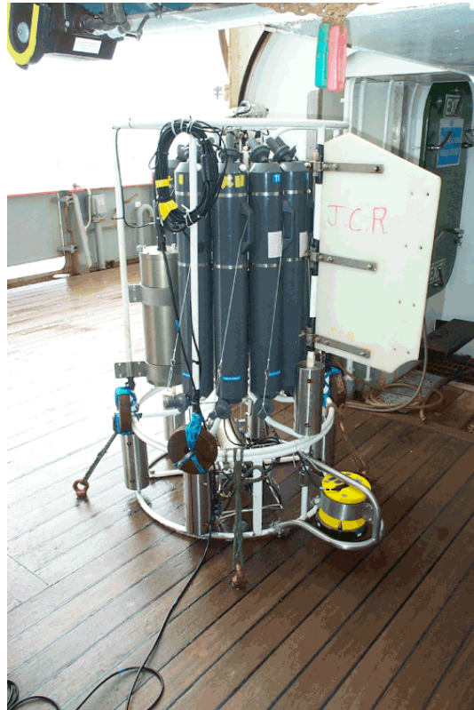
Figure 1.1a: above left: CTD frame being deployed. Note the LADCP and protective frame mount, the stabilising fin, the extra weights and the swivel. The battery pack is on the opposite side.
