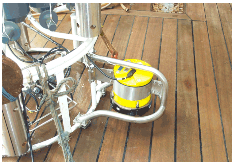
Figure 1.1c: Detail of LADCP frame mount. There are three attachment points to the CTD frame for the LADCP frame; the LADCP mounting bracket is attached on the right to the LADCP frame and on the left to the CTD frame.
