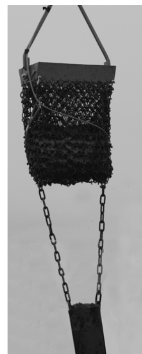
Figure 94. The UK National Marine Equipment Pool (SOC) rock dredge as used during RRS James Clark Ross cruise JR97 conventionally rigged with dredge bucket.
