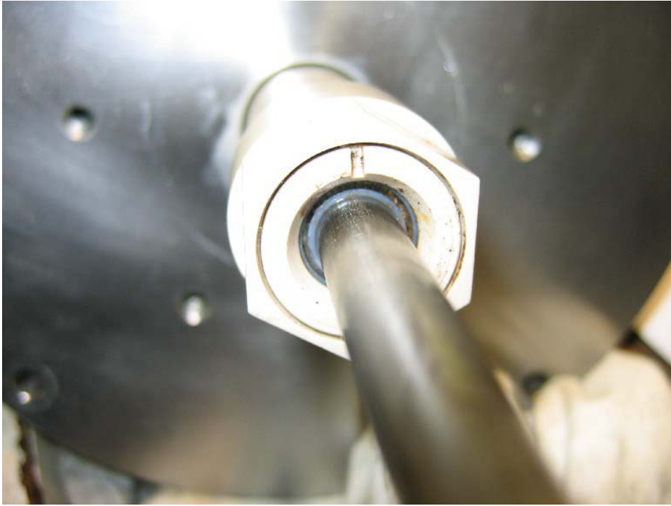
Figure 42a. Lip seal on syringe drive shaft
