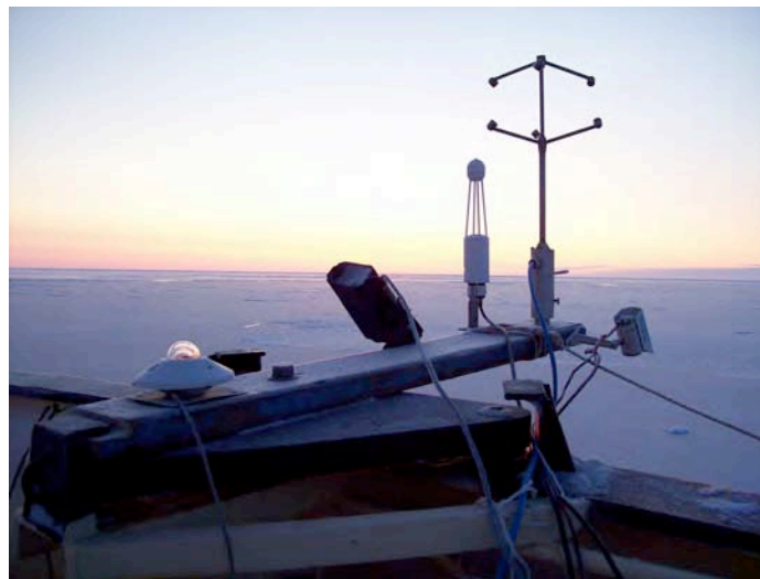
Figure I.6.2.1: Turbulent devices installed on the ship.
