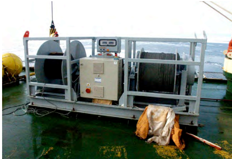
Figure I.2.2: LEBUS double-drum oceanographic winch on the helicopter deck.
