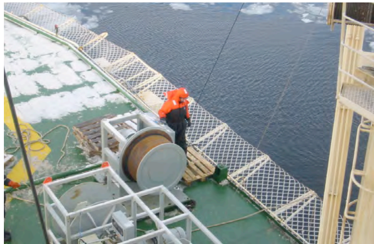
Figure I.2.3: HAWBOLDT C15-40 horizontal capstan on the helicopter deck.
