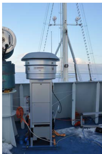
sol sampler on the monkey island deck of the RV Lance during
