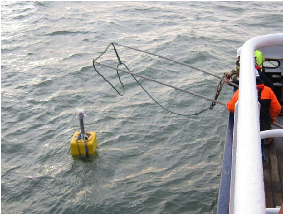
Figure 3. Recovering the spar buoy (deployed 8th November 2011 on cruise 80), with loop and boathooks.
