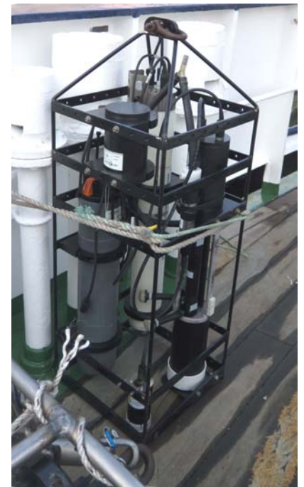
Figure 6. Dipping frame with CTD, ac-s (Triplet not used).
