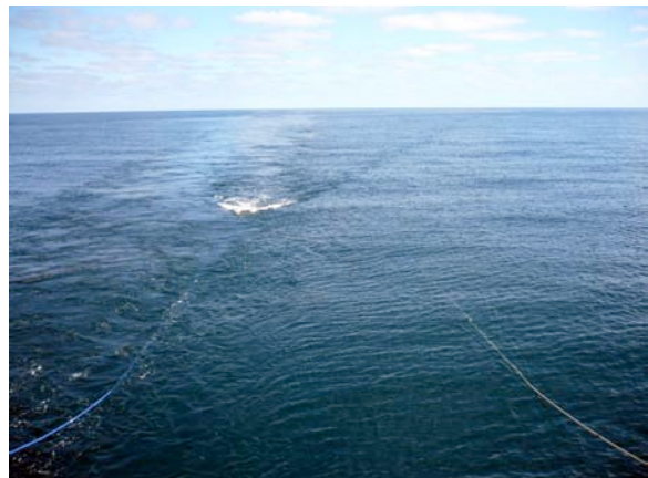
Figure 4. View of the Sparker system in the water, with the source catamaran on the left of the picture and the multichannel streamer seen on the right.
