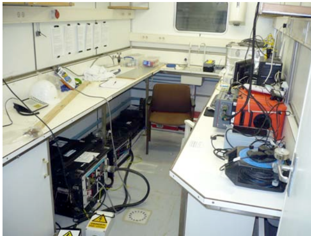
Figure 5. View of the Sparker and Boomer recording laboratory in the container on the fantail of the vessel. Recording equipment and computer controls are seen on the right on the shelf, while the two source units were placed under the counter on the left of the image.
