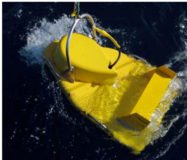
Figure 2. Edgetech SB-512i "Chirp" seismic system being deployed over the stern of RV Pelagia during cruise 64PE300.
