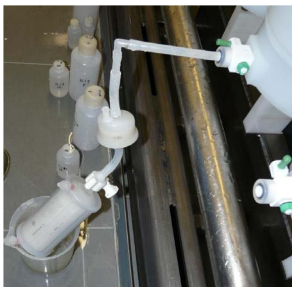
Figure 22. Ultrafiltration of seawater samples directly from the UCC CTD bottles.
