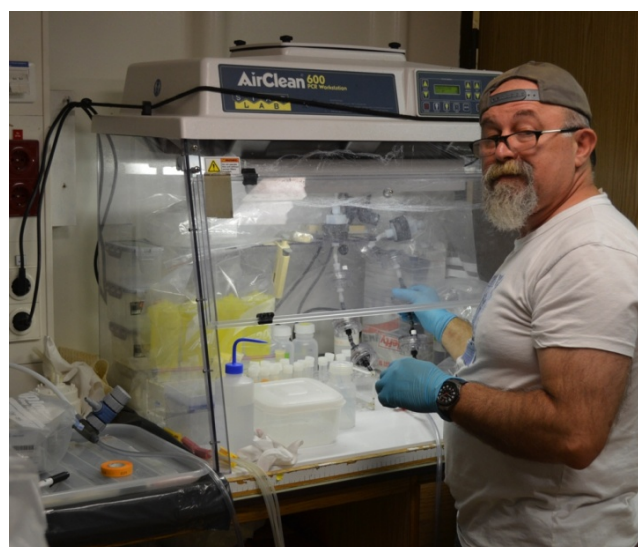
Figure 23. Can Bizsel size-fractionating the phytoplankton population during cruise 64PE373.
