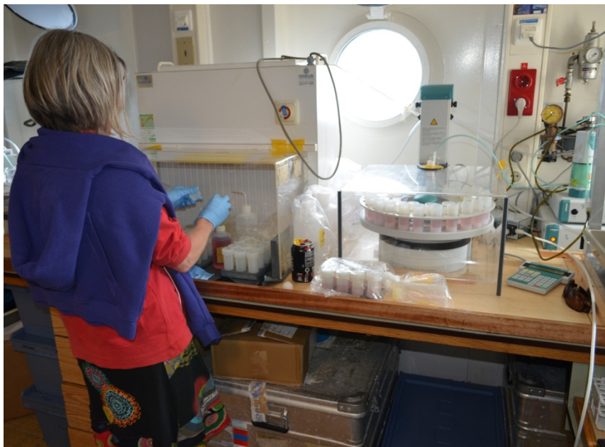
Figure 22. Loes preparing a titration for organic Fe-binding ligands during cruise 64PE373.
