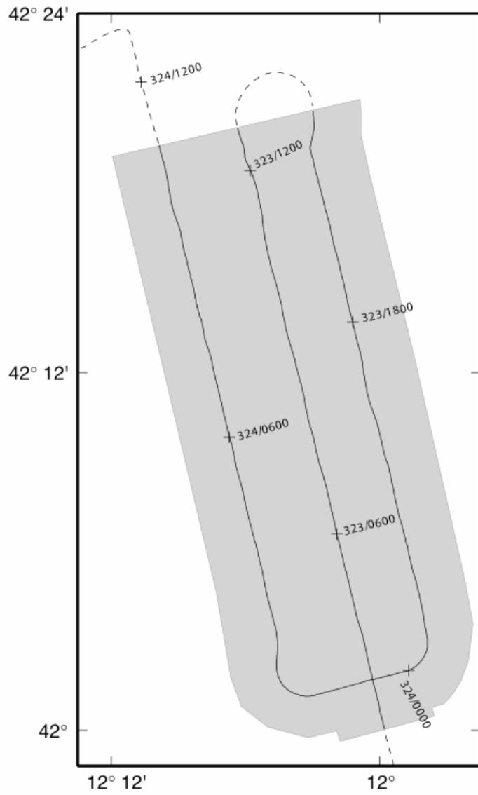
Figure 4. Track chart and TOBI sidescan sonar coverage (shaded) for the *Prestige* study area. Solid track lines are those along which sidescan data was acquired, dotted lines are passage tracks.
