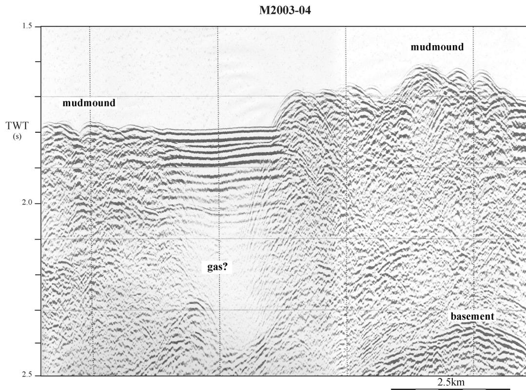
Example of a seismic line across the mud mounds in the Faeroe-Shetland Channel. The lack of internal reflectors in the centre of the image might result from the presence of gas.
