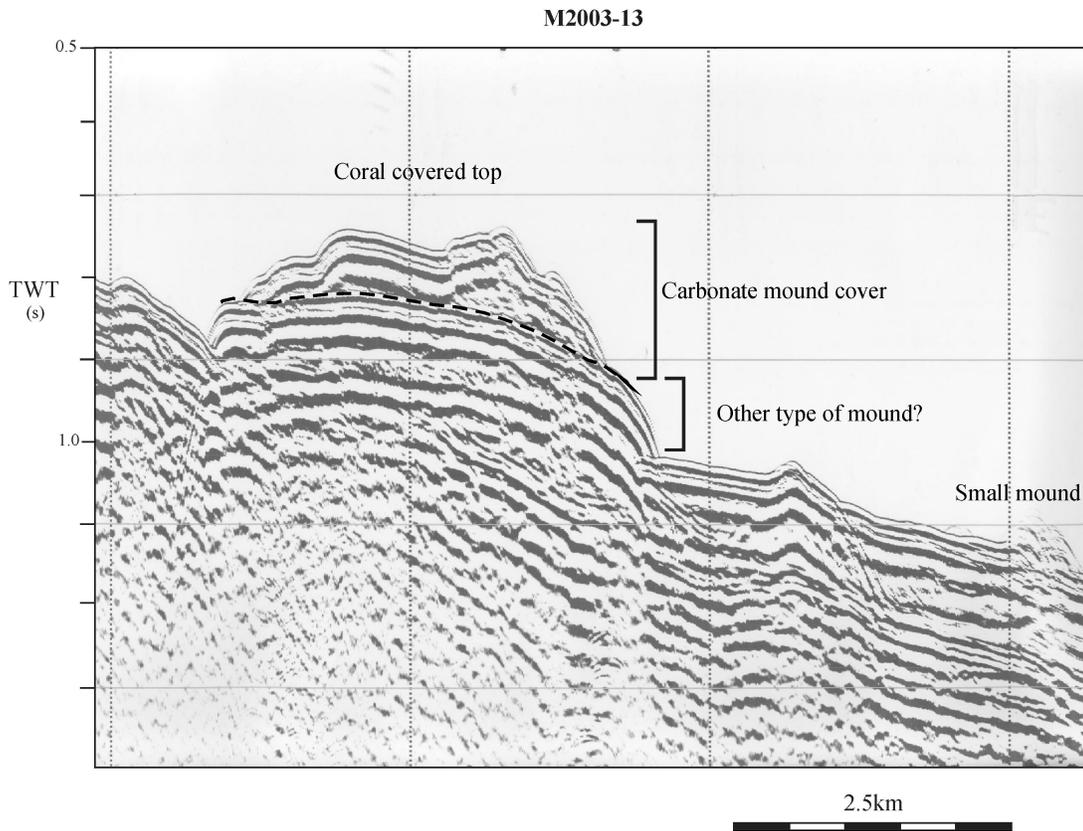
Seismic profile across a mound on the slope of the Rockall Bank. This mound appears as a circular structure on the M2002 TOBI side scan mozaic (Appendix III, right hand side of the TOBI image). A clear internal reflector (dashed line) is present on which a cold water carbonate mound appears to have developed.
