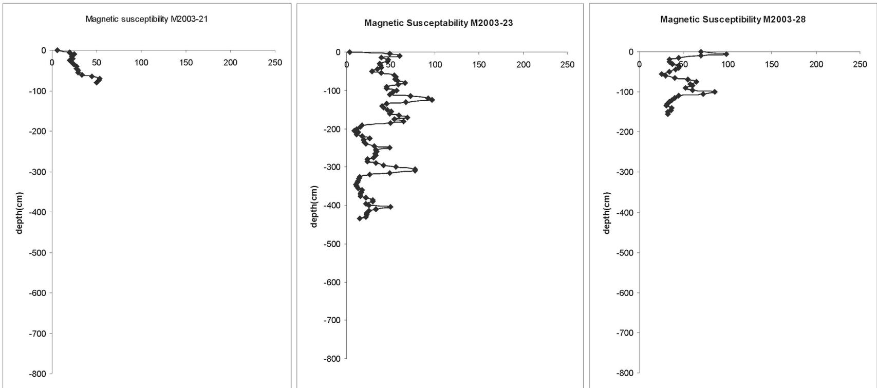
Magnetic susceptibility of piston cores taken on the mounds on the flank of Rockall Bank.
