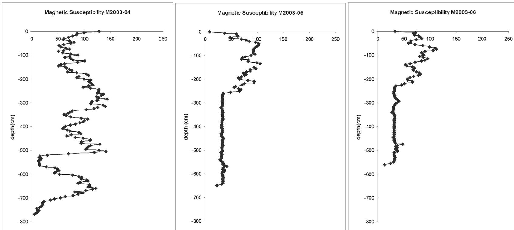
Magnetic susceptibility of piston cores taken in the Faeroe-Shetland Channel. Note the similarity in susceptibility pattern of cores 5 (taken out side the mound area) and 6 taken in the central depression of a mound). Core 4 was taken on top of a mound.
