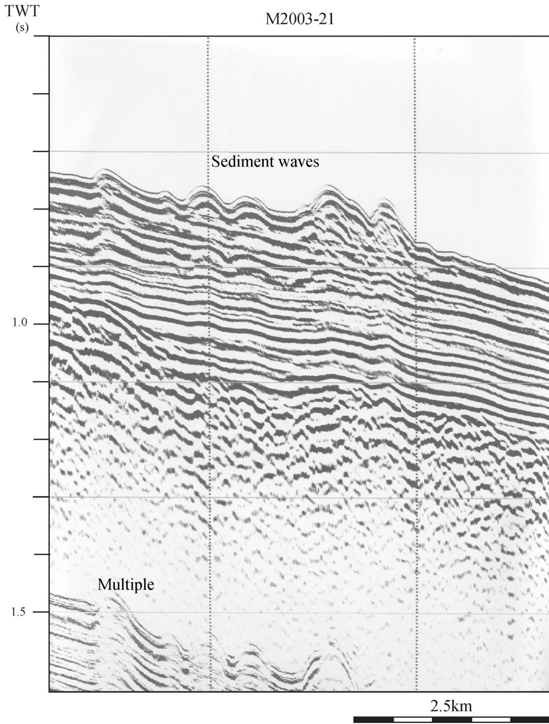
Seismic line across megaripples shown on the upper left hand side of the M2002 TOBI mozaic (Appendix III).
