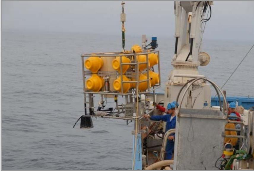
**Fig. 19** Deployment of benthic ALBEX lander.
