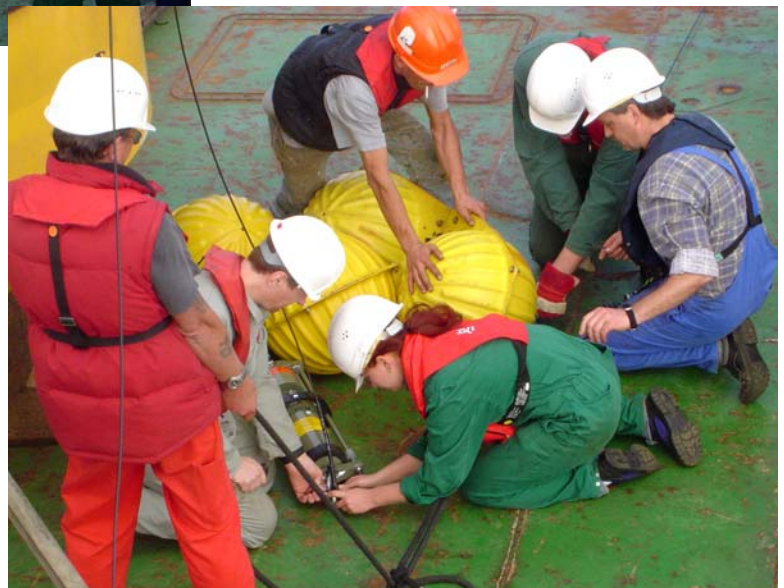
Figure 17: Preparing the RCM 11 for deployment.
