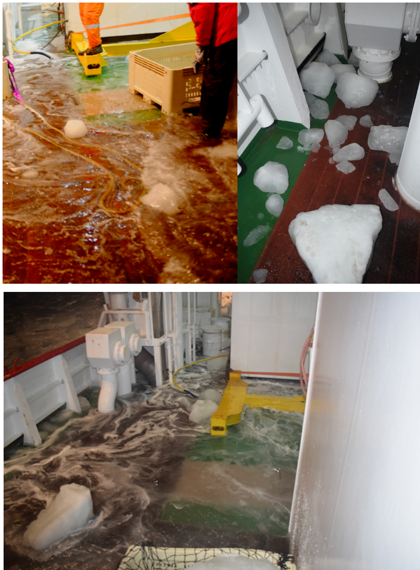
Figure 64 Consequences of ship slamming on sea ice during the pancake lifting operations
