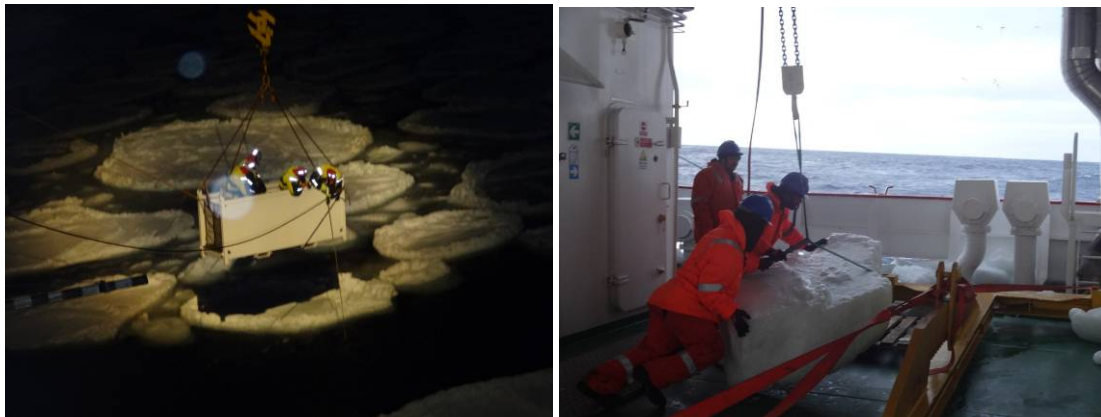
Figure 63. Sampling in the marginal ice zone. Left: UCT Oceanography and Civil Engineering teams sampling surface water in pancake ice using a handheld Niskin bottle. Right: typical chunk of pancake ice collected from the marginal ice zone (note the ice displayed on the photo is a spare ice float that was not used for trace metal or biogeochemical subsampling).
