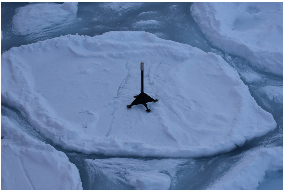
Figure 36 View of tracker transceiver unit on the ice
