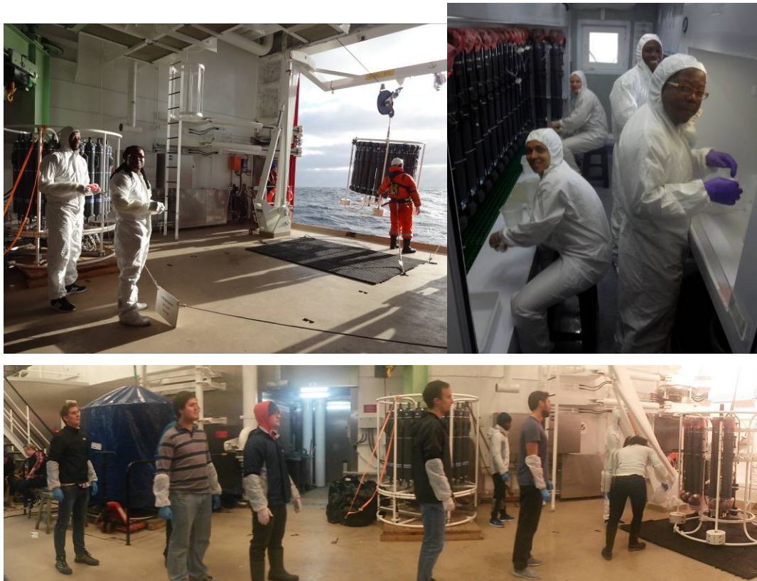
Figure 59. Upper left panel: Water sampling using the GEOTRACES rosette, equipped with Teflon coated frame and GoFlo bottles. Lower panel: Cruise participants queuing to carry GoFlo bottles from the CTD rosette to the clean container laboratory on the aft deck. Upper right panel: Natasha, Thato, Ryan and Andile subsampling from the GoFlo bottles in the trace metal clean container.
