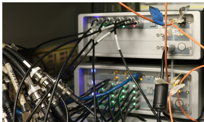
Figure 10: Frontend of the hull vibration measurement setup
