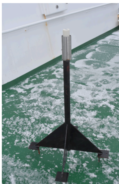
Figure 35 View of a typical tracker transceiver unit fixed into a socket on a foundation assembly.
