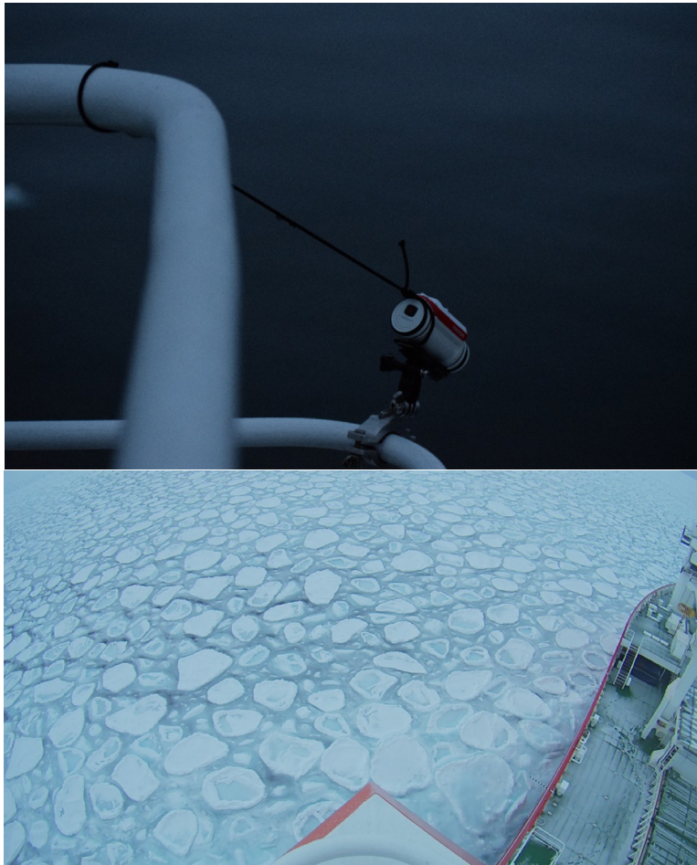
Figure 45 Location of the TomTom action camera on port side and the relative field of view over sea ice.
