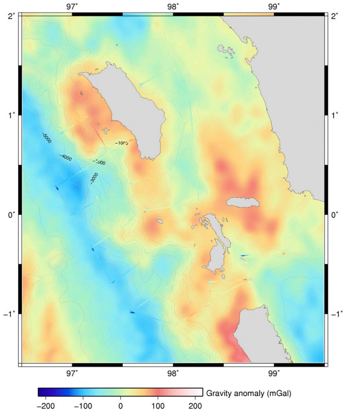
**Figure 83:** 2-minute gravity measurements in Survey Box 2, adjusted for instrument clock drift and basic Eötvös correction. The main misfits arise from error in ship velocity and heading, as can be observed in the data near turns. The background grid is from Sandwell and Smith (1997).
