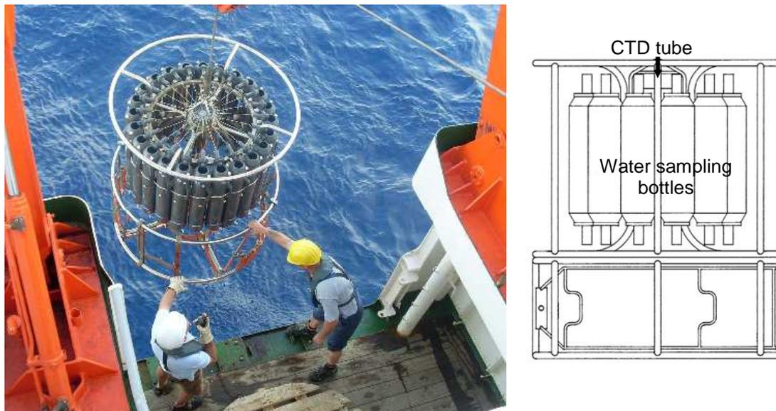
**Figure 22: The Sea-bird Electronics Carousel Water Sampler and 911plus CTD being recovered (left), and in schematic form (right); the CTD is in a vertically oriented tube located in the centre of the water sampling bottles. The water sampling system was not used during SO198-1. Photo by D. Sobaruddin.**
