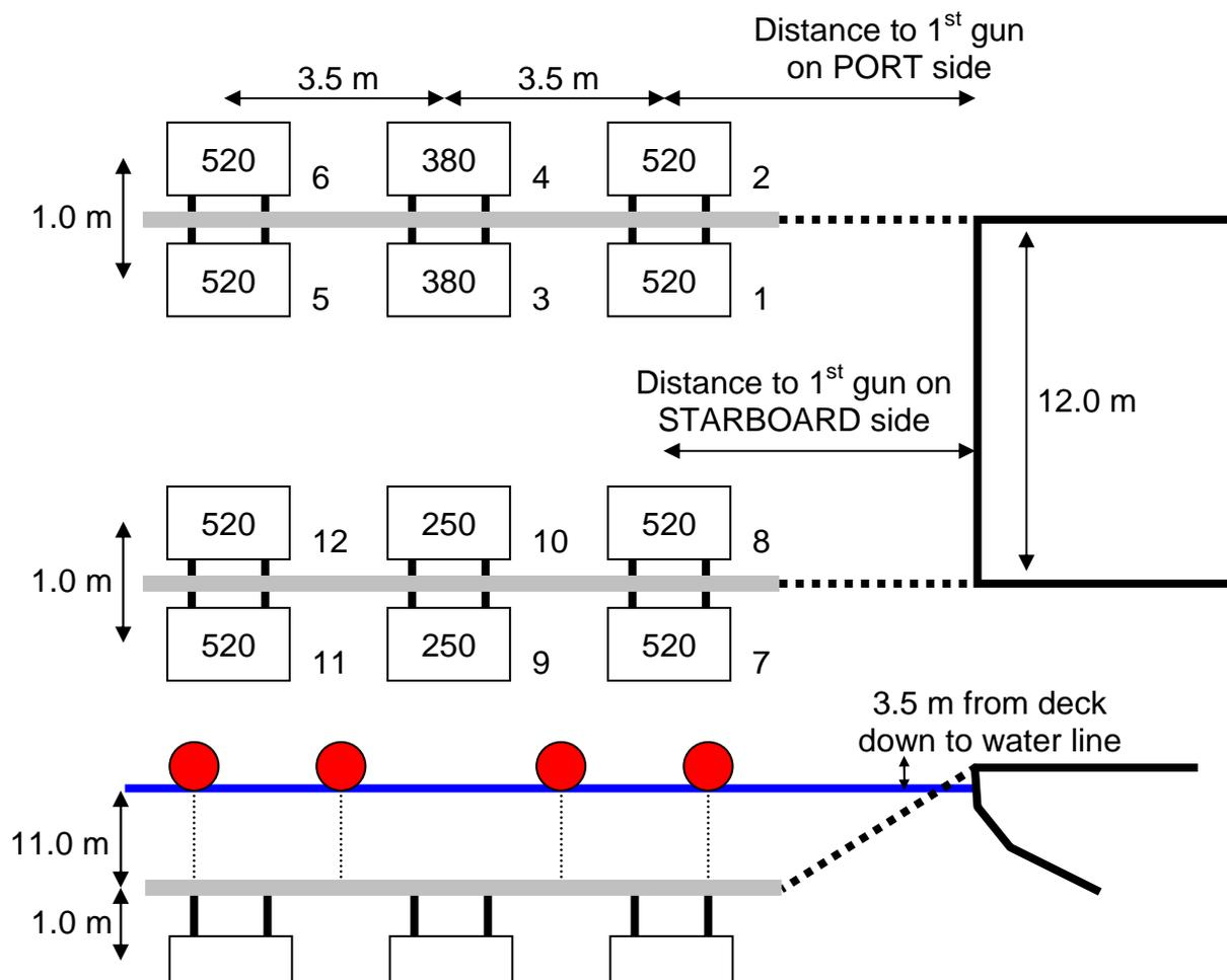
**Figure 5: Schematic diagram showing the dimensions of the airgun array towed during SO198-1, and the airgun numbers, as used by the gun controller. Airgun volumes are given in cubic inches, all other dimensions are in metres. The distance between the back of the ship and the first airgun in the port and starboard array varied during the cruise and are given in Table 1.**
