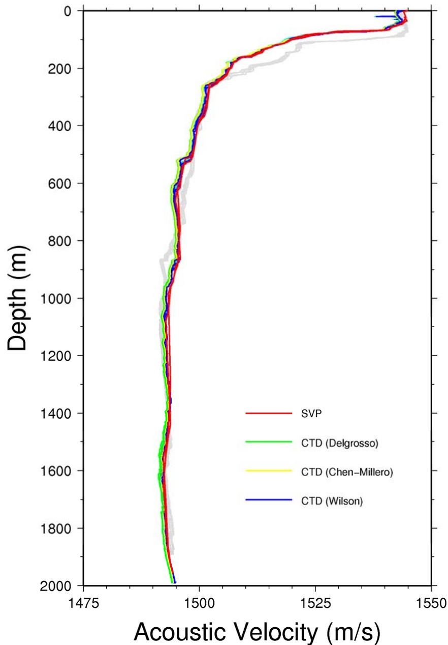
Figure 77: Acoustic velocity measured by the SVP probe in Survey Box 2 (red) and calculated from the CTD data at the same location using the method of Delgrosso (green), Chen-Millero (yellow) and Wilson (blue); the grey lines show the data from Survey Box 1 (Figure 58).
