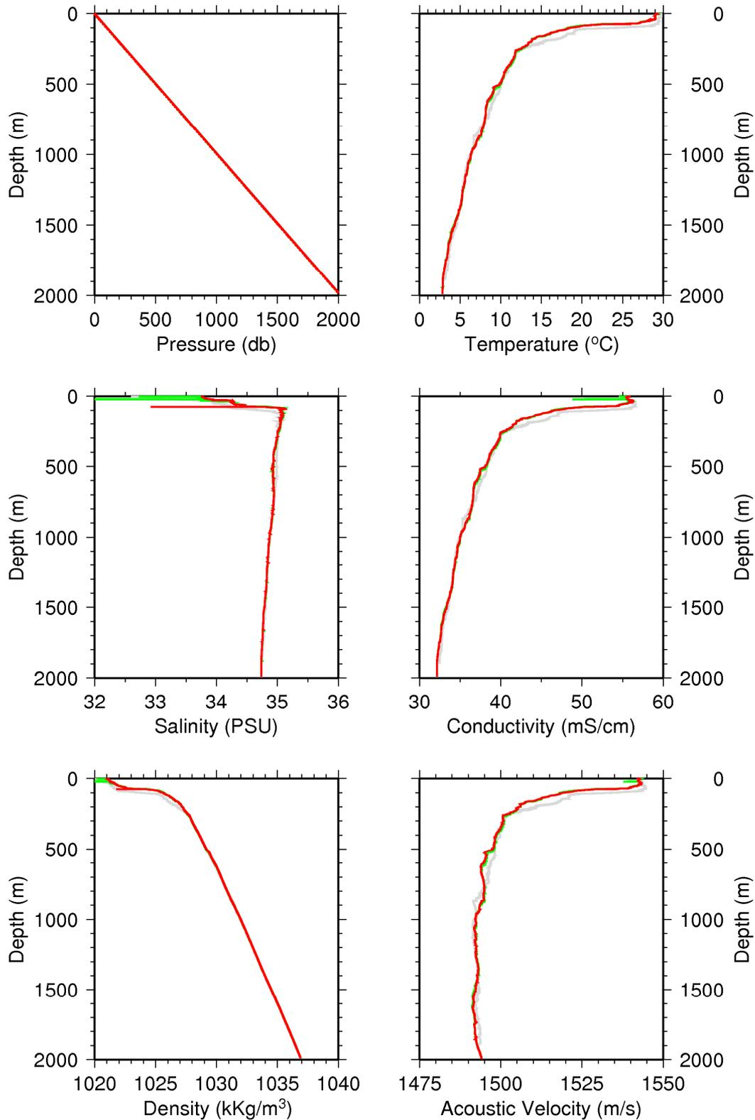
**Figure 76: The result of the CTD drop acquiring during OBS recovery in Survey Box 2; red lines identify data acquired as the probe went down, green lines identify data acquired as the probe came back up, grey lines show the result of the CTD drop in Survey Box 1 (Figure 57) for comparison.**
