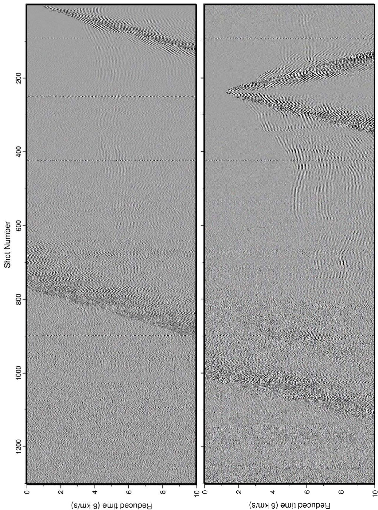
**Figure 54: Hydrophone data from OBS instruments at Sites A01 (upper panel) and A02 (lower panel) for all the shots along SUMA (197 km). Data are shown with reduced time (6 km/s), zero-phase band-pass filtered (3-5-25-30 Hz), and gain proportional to offset.**
