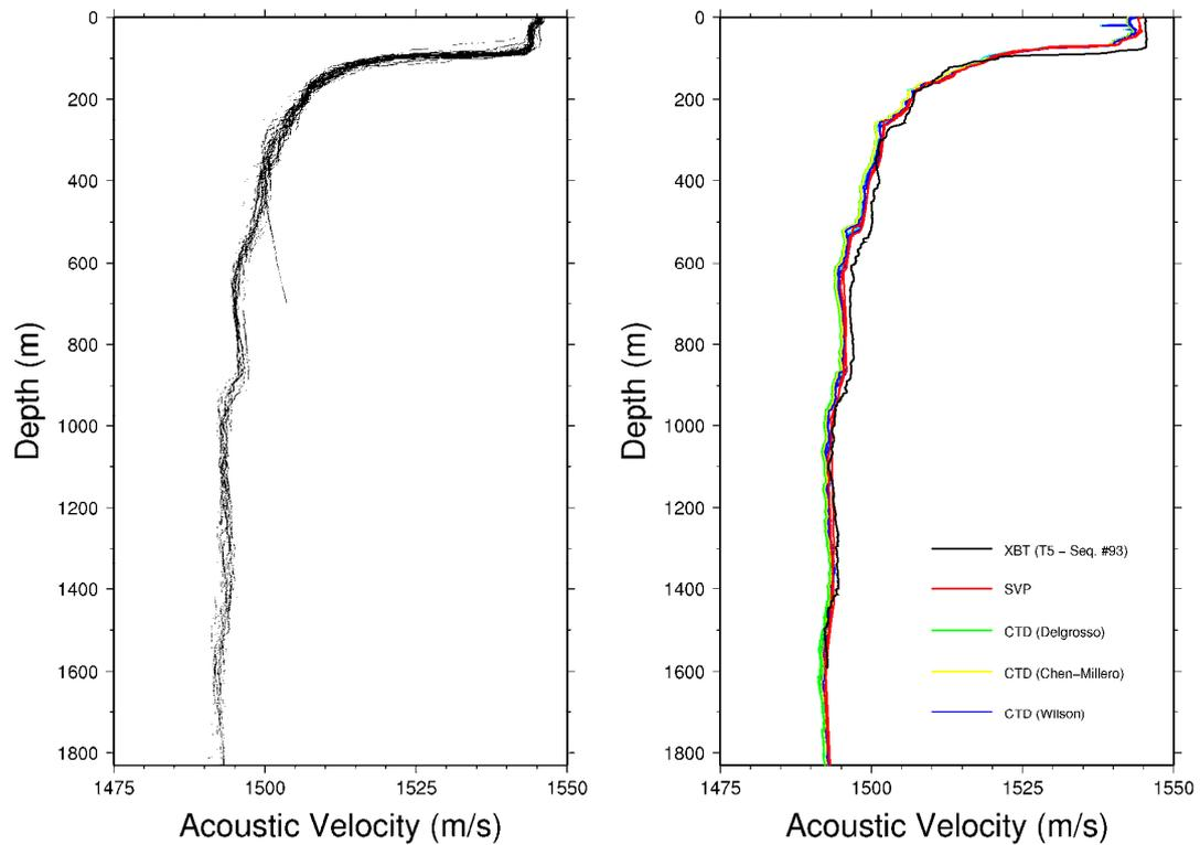
**Figure 79: Acoustic velocity versus depth profiles obtained from all XBT probes launched in Survey Box 2 (left). The velocity values obtained by the SVP and CTD probes are close to those from the nearest XBT probe (right), but do not match as well as the results from Survey Box 1 (Figure 60).**
