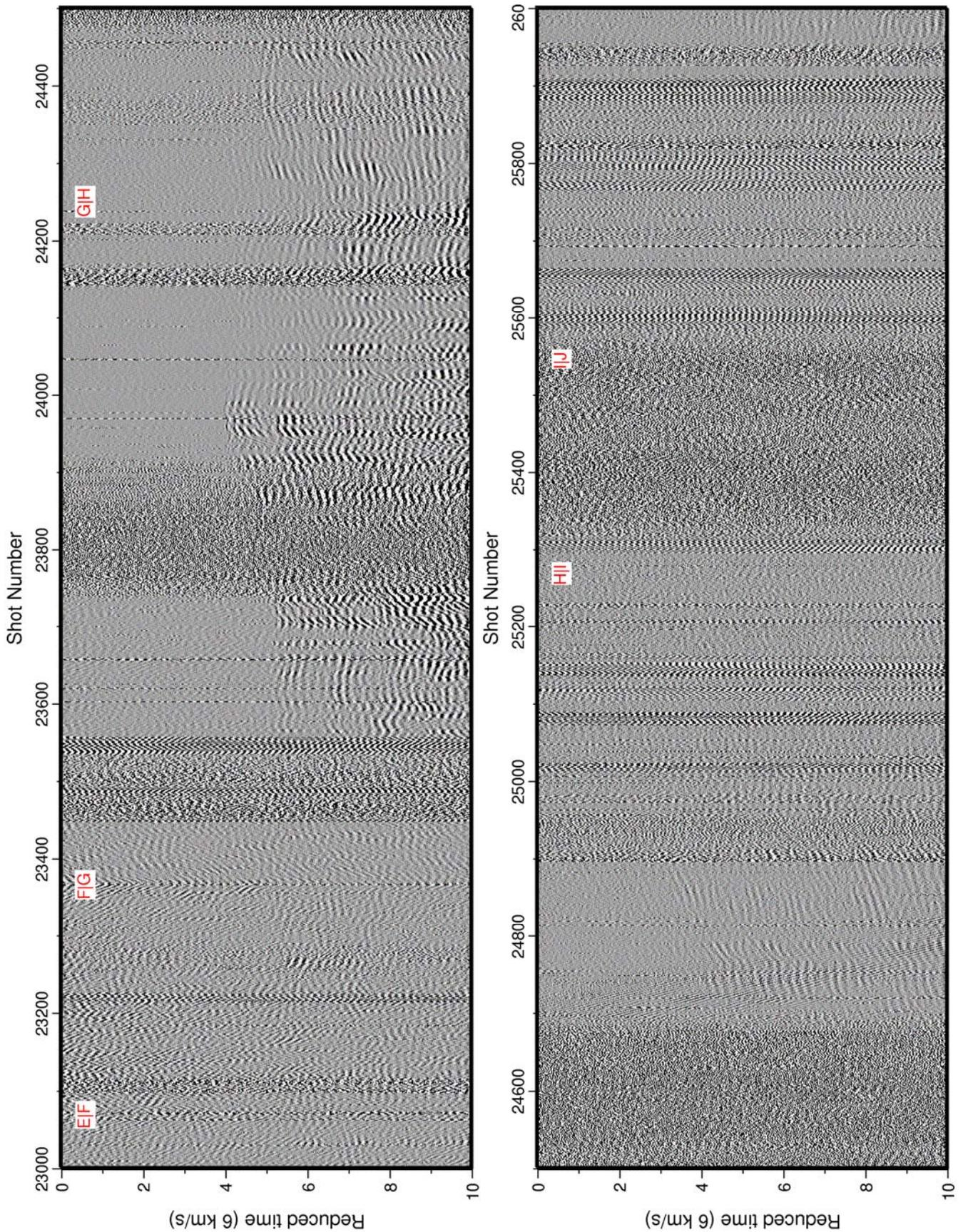
**Figure 74: Vertical geophone data from Site B34. Data are shown with reduced time (6 km/s), zero-phase band-pass filtered (3-5-25-30 Hz), and gain proportional to offset. Line segments SUMBE to SUMBJ are labelled in red.**
