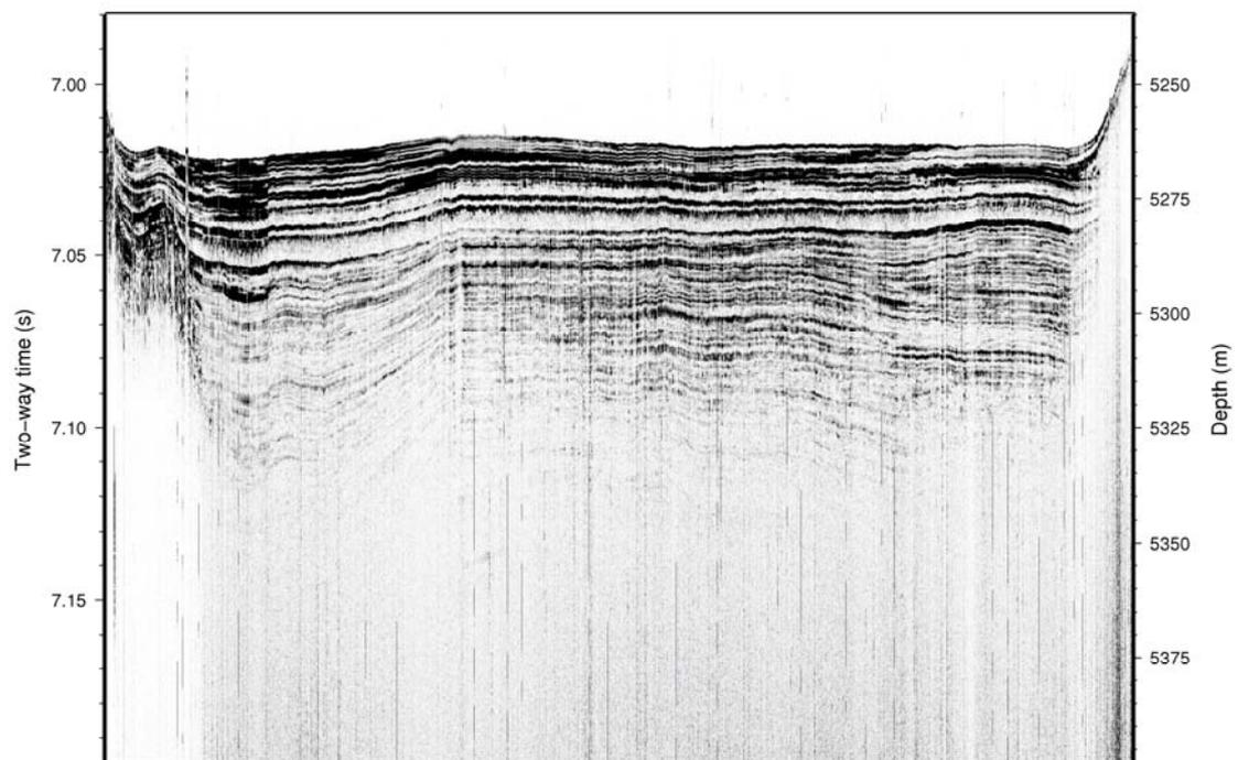
Figure 82: An example *Parasound* section along profile SUMBP in Survey Box 2, showing reflection horizons up to 75 m below the seabed. The data have had time<sup>3</sup> amplitude recovery applied, and an automatic trace static correction to increase coherency.
