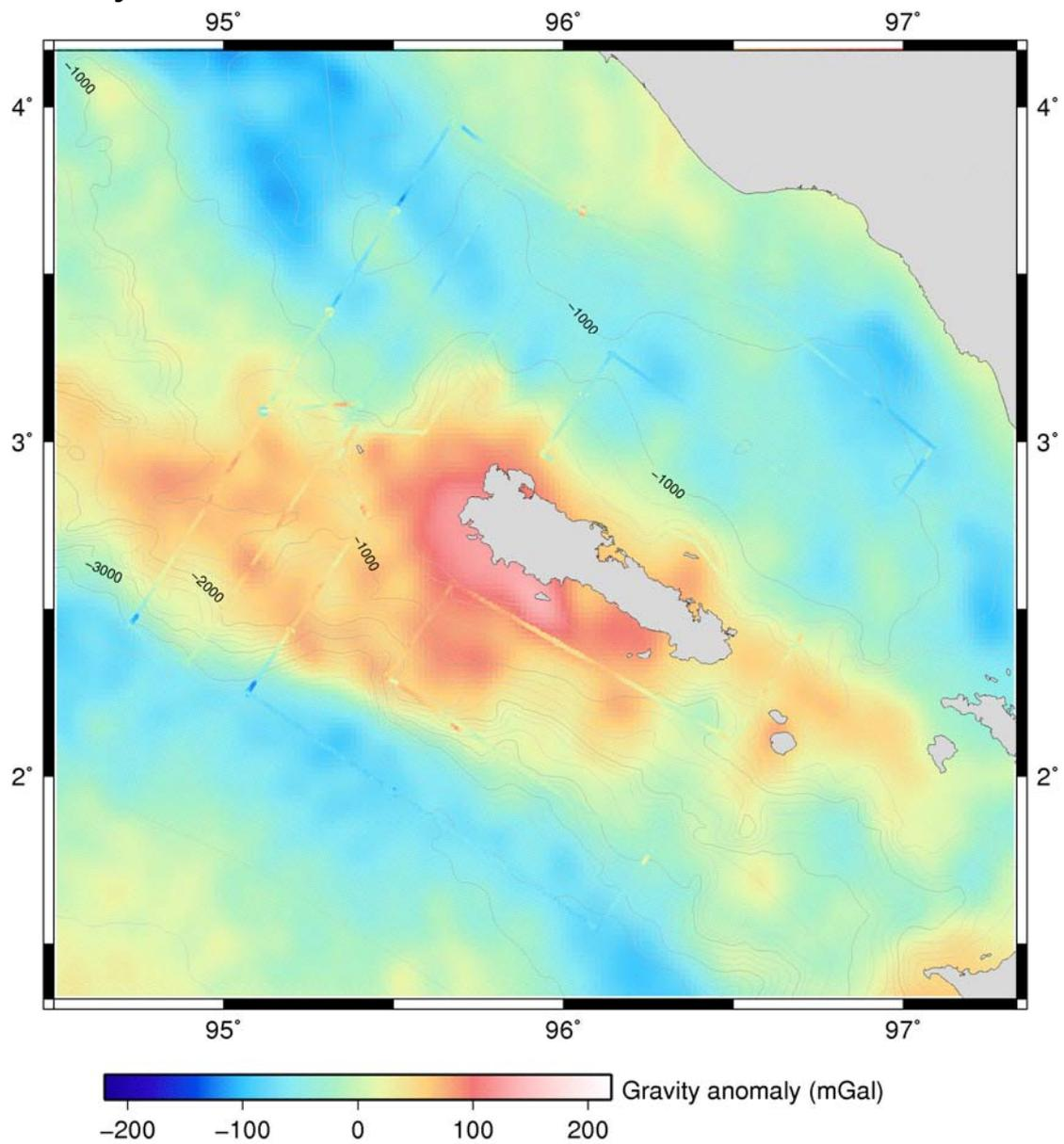
**Figure 66:** 2-minute gravity measurements in Survey Box 1, adjusted for instrument clock drift and basic Eötvös correction. The main misfits arise from error in ship velocity and heading, as can be observed in the data near turns. The background grid is from Sandwell and Smith (1997).
