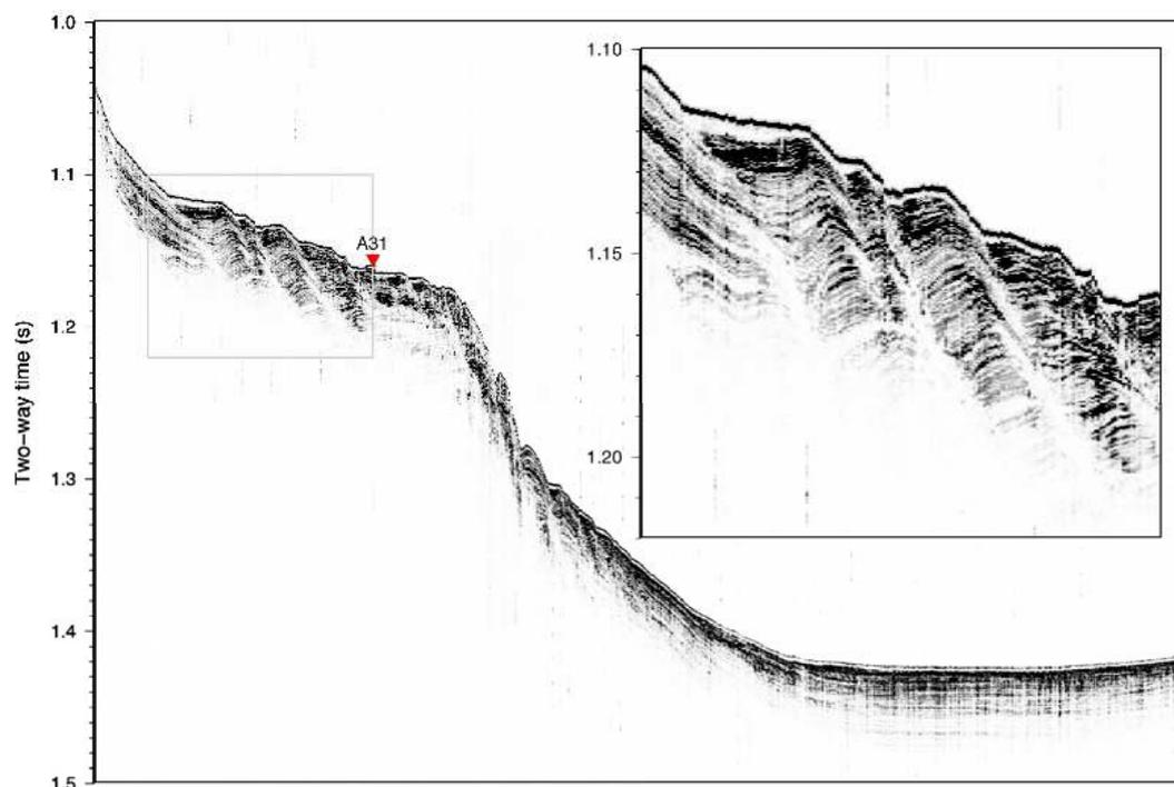
Figure 65: An example *Parasound* record, oriented SSW-NNE, acquired during the deployment of the OBS instruments in SB1; the deployment location of instrument A31 is identified by the red triangle. The data were converted to SEG-Y format and processed as described in the text. The inset shows an enlarged region identified in the main figure by the grey box. Note that the horizontal scale is dependent on the speed of the vessel and is not constant in this figure.
