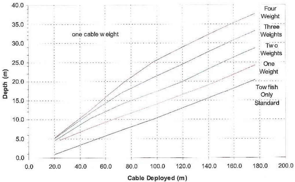
Figure 45: Towing depth of the SeaSPY tow fish at 3 kt towing speed. The un-weighted (standard) tow fish (bottom curve) represents the sensor used during SO198-1 (after Marine Magnetics Corporation, 2008).
