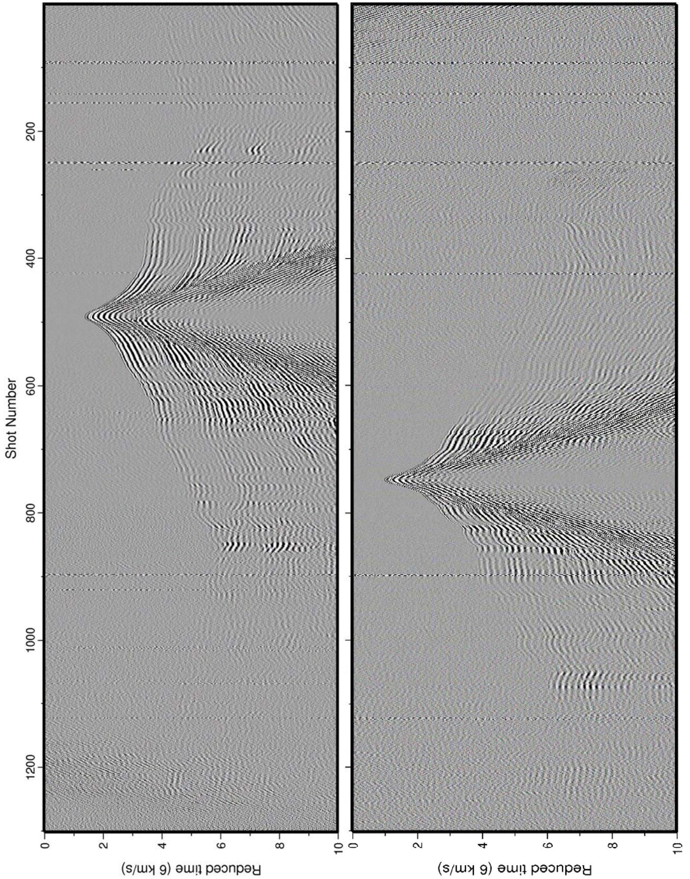
**Figure 55: Hydrophone data from OBS instruments at Sites A03 (upper panel) and A04 (lower panel) for all the shots along SUMA (197 km). Data are shown with reduced time (6 km/s), zero-phase band-pass filtered (3-5-25-30 Hz), and gain proportional to offset.**
