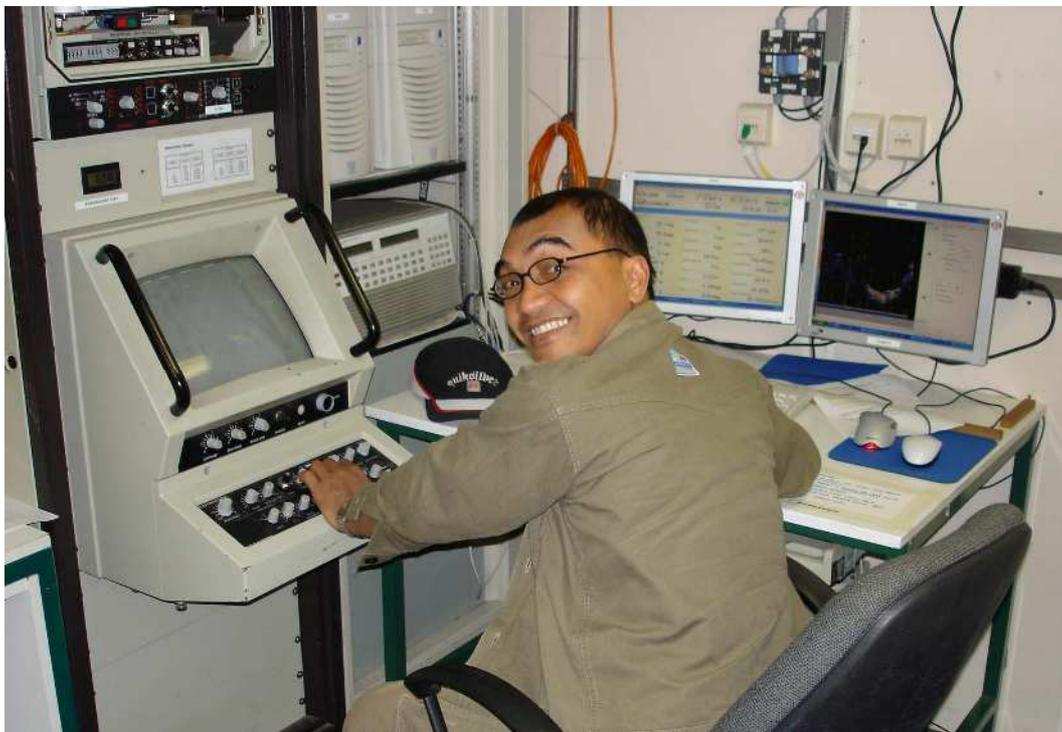
Figure 30: The *Parasound* Operator Console (left), and the *ParaDigMA* data processing and logging system display (right).
