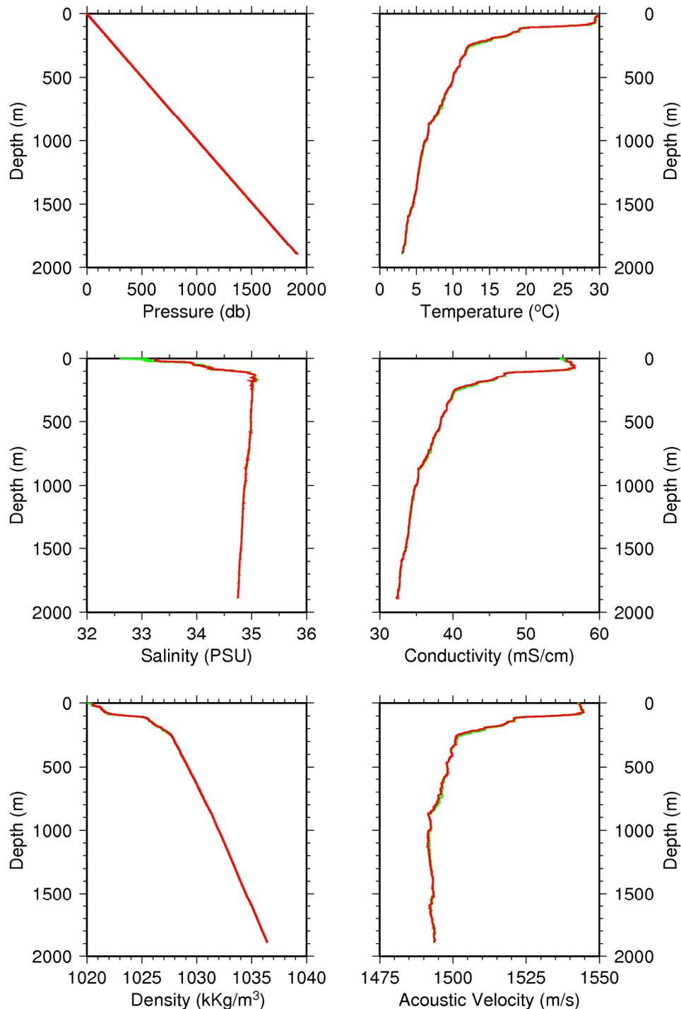
**Figure 57: The result of the CTD drop prior to acquiring swath bathymetry in Survey Box 1; red lines identify data acquired as the probe went down, green lines identify data acquired as the probe came back up.**
