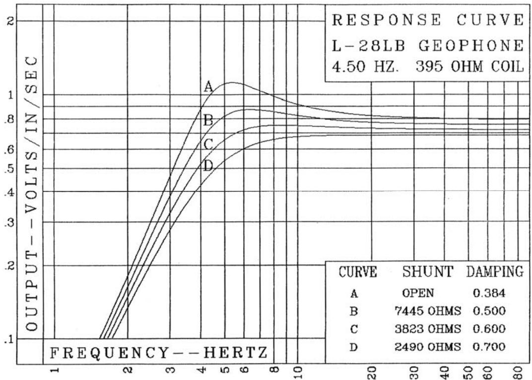
Figure 14: Frequency response for the Mark Products (Sercel) L-28LB geophone (curve A) used in the 4-channel LC2000 instruments.
