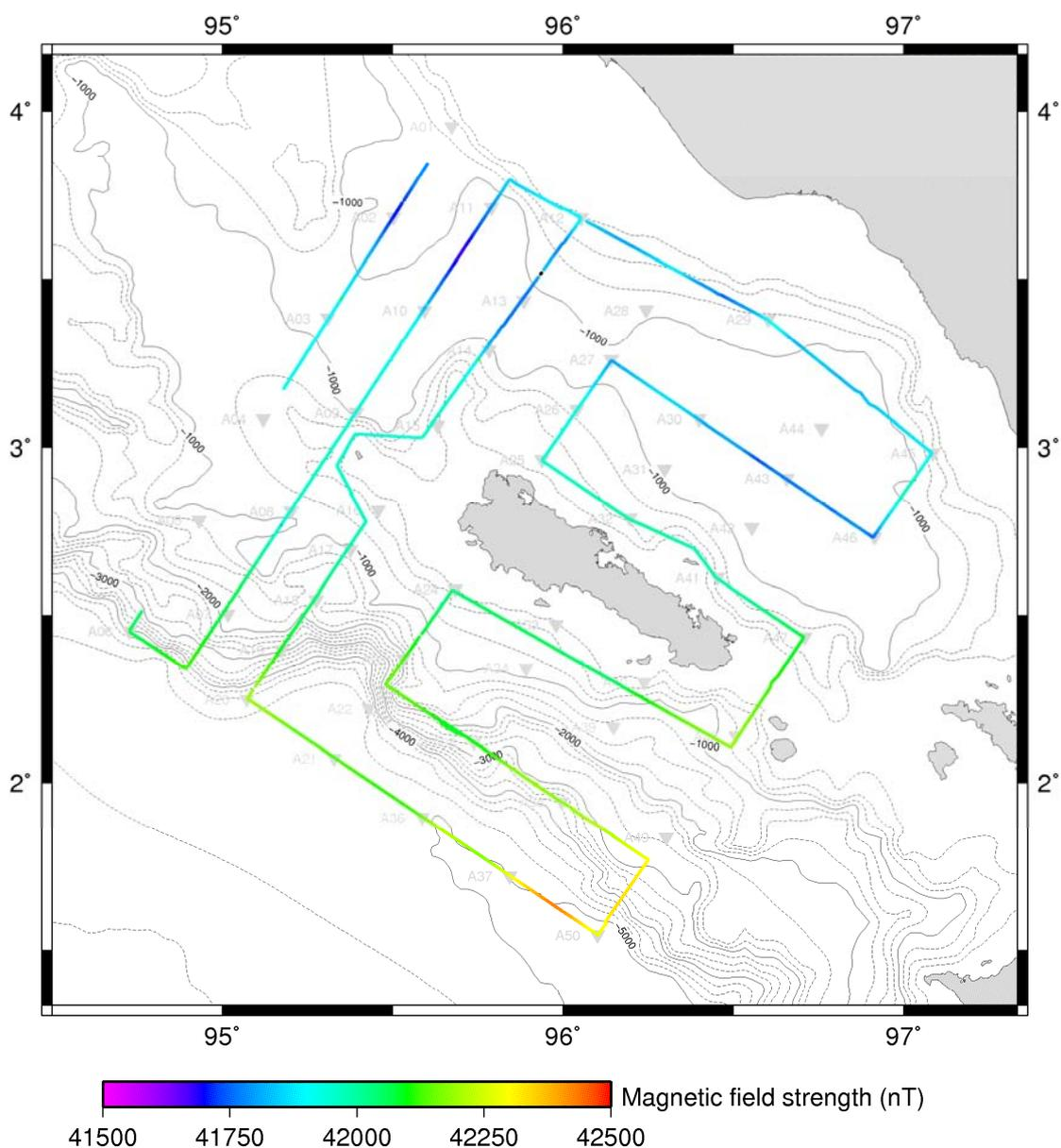
**Figure 67: Magnetic field strength in nT measured along the airgun profiles in Survey Box 1. There is a clear trend from high values in the south, over the trench, to lower values to the north, over the basin.**
