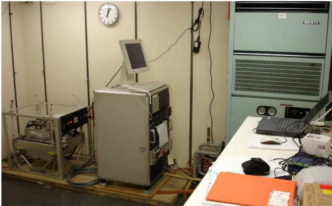
**Figure 33: The gravity meter S40 (left) installed in the *Gravimeterraum* on deck II of the Sonne with the control and logging console (centre) and the laptop PC used to capture 2-minute gravity data via an RS-232 serial connection (right; on the bench).**
