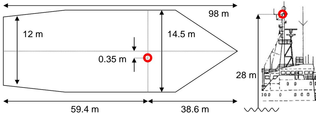
**Figure 2:** The location of the GPS antenna (red circle) on the mast above the bridge of the RV Sonne, 28 m from the water line.
