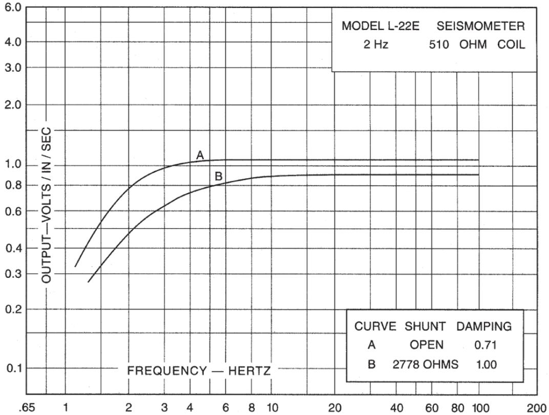
Figure 13: Frequency response for the Mark Products (Sercel) L-22E geophone (curve A) used in the 2-channel LC2000 instruments.
