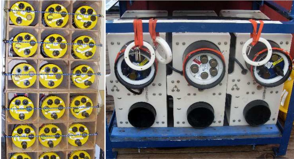
**Figure 19: The LC4x4 OBS instruments. British LC4x4 loggers (left) are distinguished from LC2000 loggers by yellow end caps. US LC4x4 loggers, hired by OBIC, have blue end caps (right; an OBIC LC2000 is lurking in the middle deployment frame). Photos by D. Sobaruddin.**
