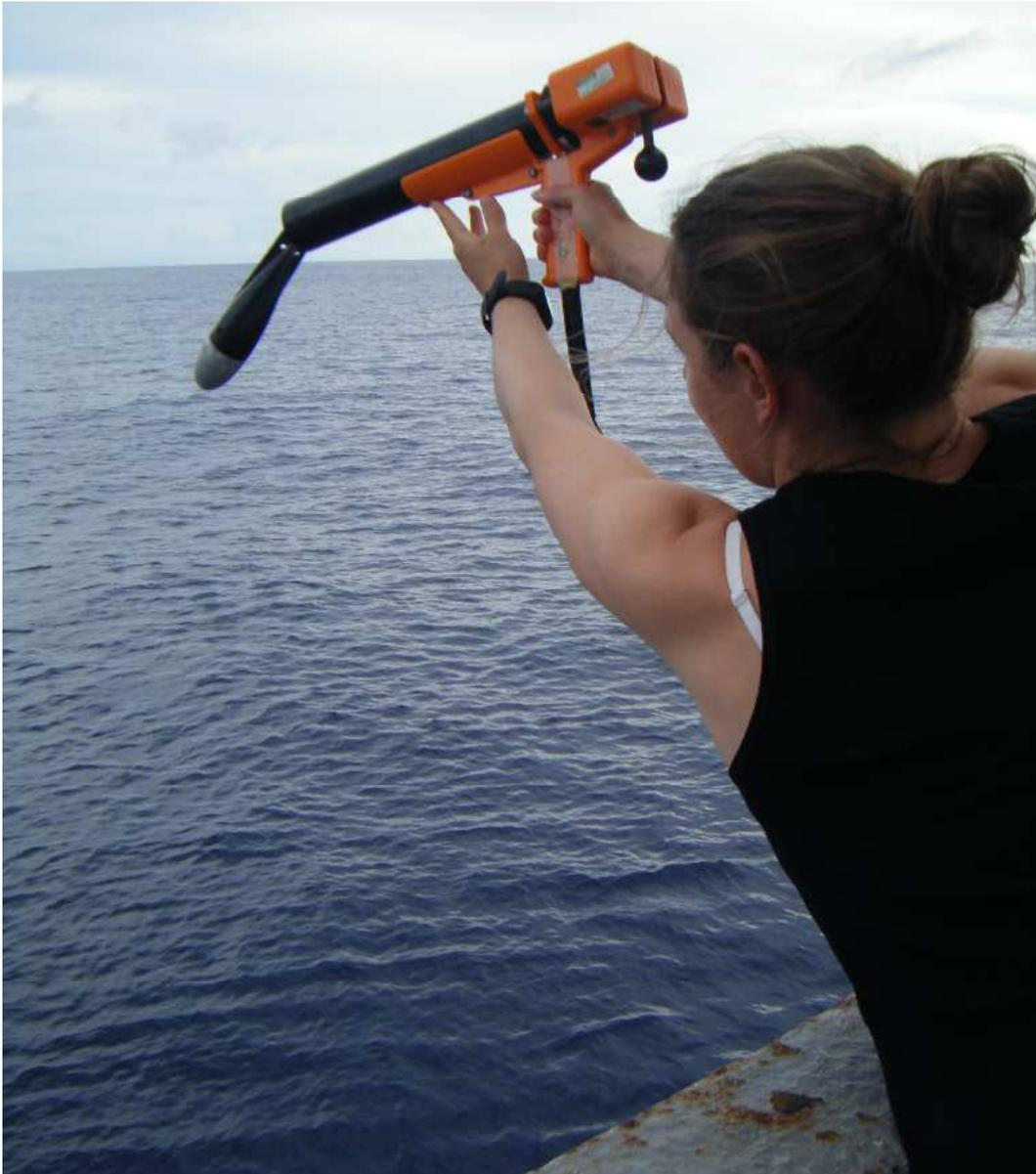
Figure 26: An XBT probe being deployed using the hand-held launcher. Photo by P. Barton.
