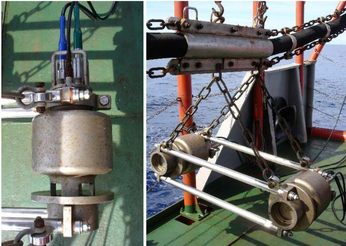
**Figure 4: An Sodera G-gun (left panel) with air hose, solenoid valve and M/P time break connectors (top), chamber (middle) and ports (bottom). Airguns were clustered in pairs of like-sized guns (right panel), each suspended by chains beneath a flexible towing frame to which the flotation buoys were attached.**
