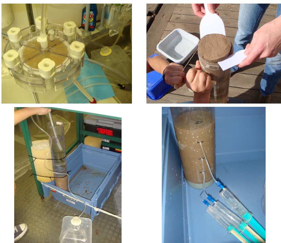
Fig. 4.3 Sampling of suspended particles (top left), sediments (top right), overlying MUC-water (bottom left), and porewater using Rhizons (bottom right).
