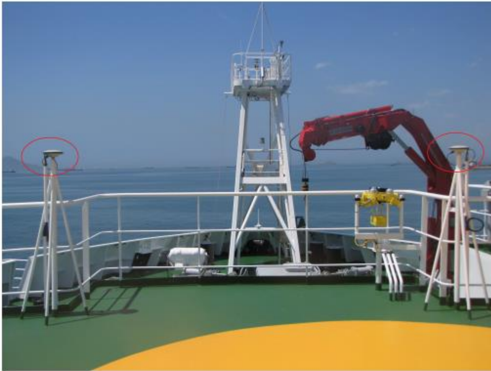
Figure 11. GPS1 and GPS2 antennas in the red circles.
