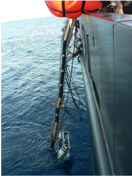
Figure 6. Deployment of the G Guns (Photo credits: SO238 Captain Oliver Meyer).
