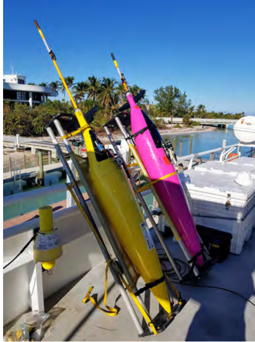
Figure 7: Two of the three Seagliders during selftests.
