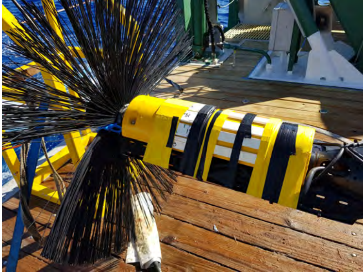
Figure 6: Seaglider buoyancy was taped onto the secondary VMP to compensate for a too-fast fall rate.
