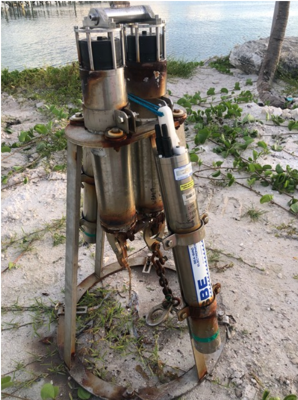
Figure 17.5 Photo of WBAL7 lander frame as recovered by a University of Miami professor.
