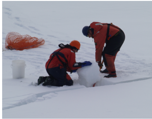
Figure 3.11 Collecting the compacted snow sample from sea ice
