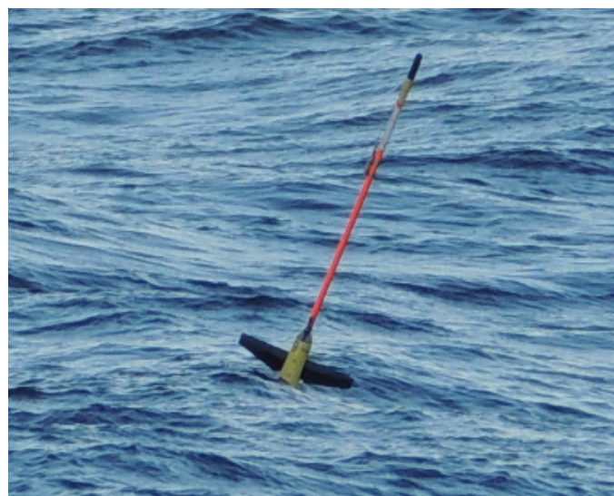
Figure 7.3 SG579 showing good surface position upon deployment
