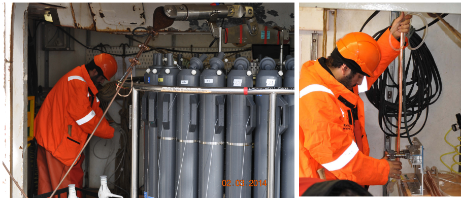
Figure 3.12 Noble gas sampling using 5/8" ID refrigeration tubing. (Left panel) Water samples were collected from the rosette
