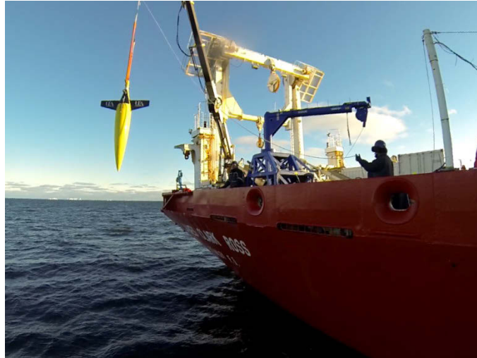
Figure 7.2 Deployment of SG579 using the starboard aft crane
