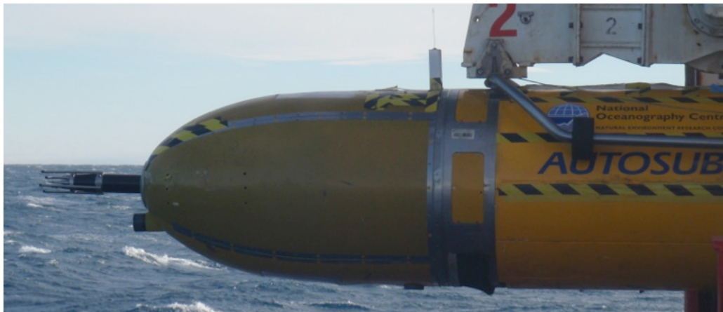
Figure 6.10: Photo of Autosub 3 being launched for mission M447. Note the position of the MicroRider at the nose of Autosub. The probes were positioned approximately 40 cm forward of the main structure in an attempt to reduce the AUV form drag impact on the flow surrounding the probes without compromising too heavily on the added vibration induced by having a long forward extension. Also, AUV-induced mechanical vibrations were dampened by special rubber-band fixings.
