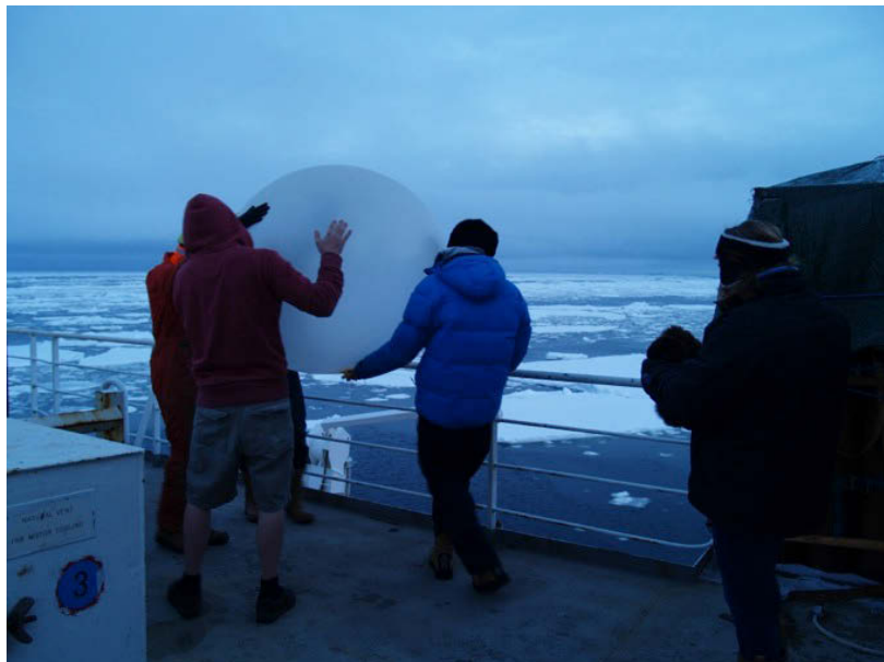
Figure 9.4: A photo showing a launch team moving the balloon towards the correct location. In high winds the two people on the downwind side must be prepared to move quickly out of the way to avoid the balloon and sonde.
