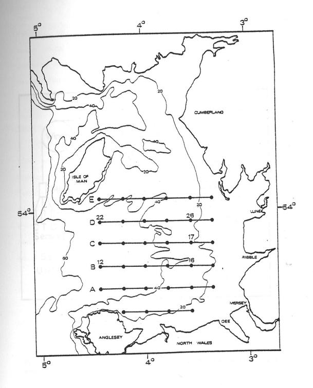
Fig. 3.1 Sampling grid for the Liverpool bay surveys. CTD casts were performed at all stations marked with heavy dots and at additional stations midway between them. The mooring was deployed at station 17.
