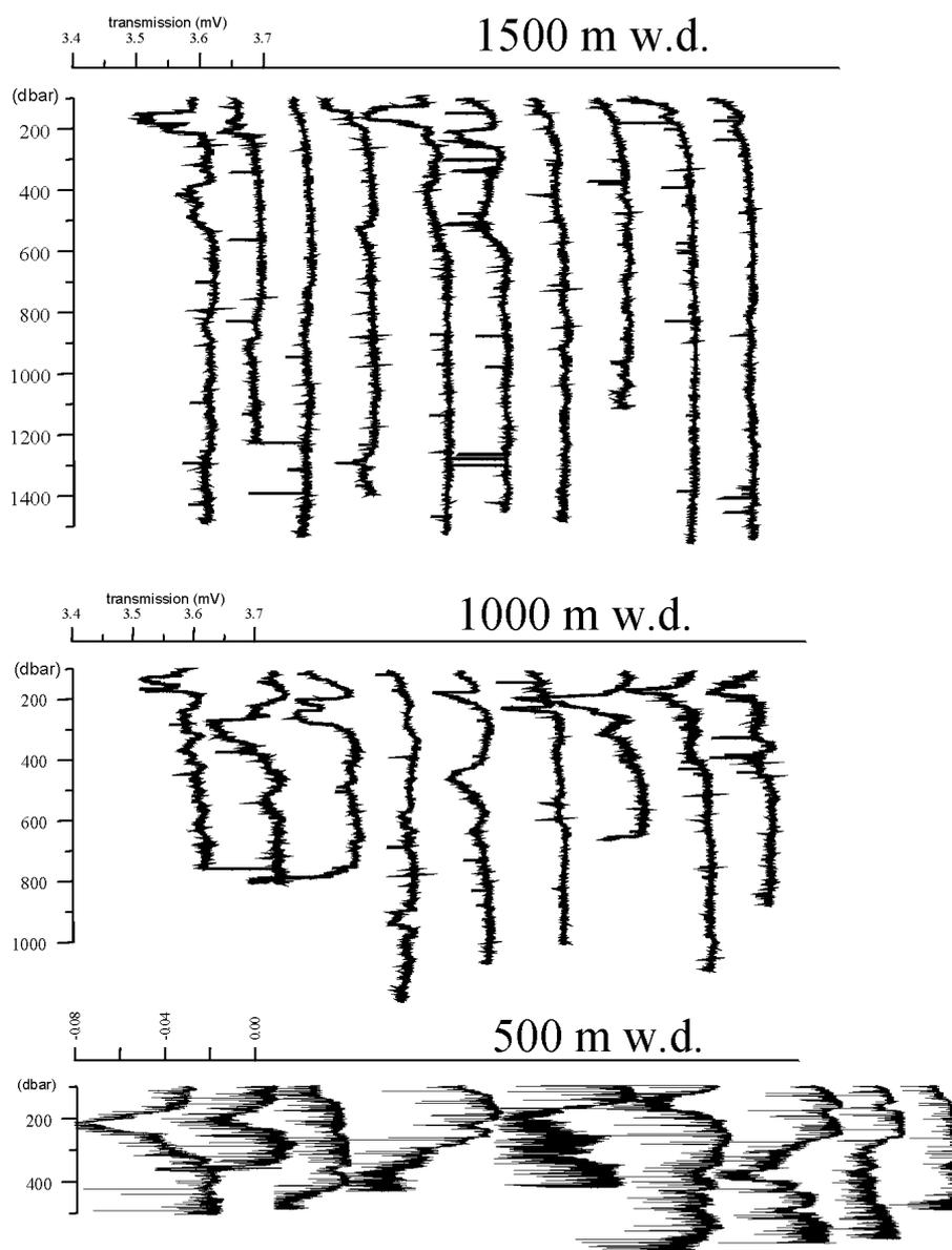
Figure 3: Transmissiometer profiles (raw data; mV) below 100-m depth taken on along-slope transects following the 1500-m and 1000-m depth contours. Lower plot gives backscatterometer readings (raw data in mV, multiplied by -1) along the 500-m isobath.
