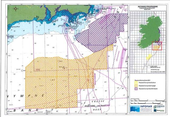
The Orange hatched area in the image is the proposed survey area for the Celtic Voyager. This area is in Irish waters but survey line turns will take the vessel into UK waters. The Celtic Voyager will not be conducting seabed sampling in UK waters. A magnetometer will be towed 100 metres behind the vessel. There is no requirement to install any equipment on the seabed.
