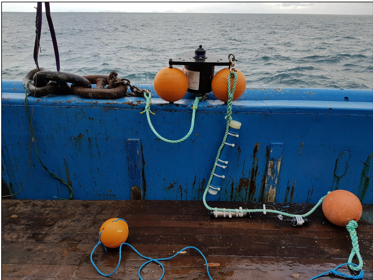
Figure 1: Mooring laid out on deck of Scotia.
