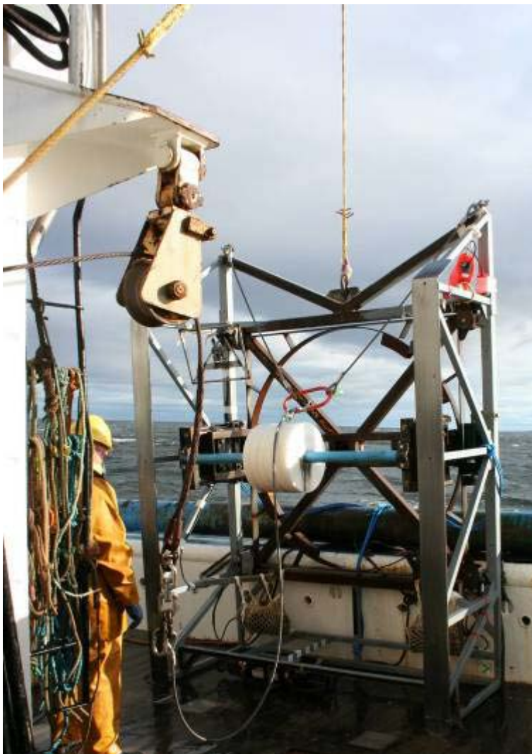
Figure 2: The Big sledge with towing bridle and lifting line attached, the ground gear being tested is 400mm discs in the “block” arrangement.
