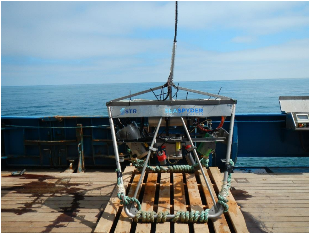
Figure 2. STR SeaSpyder drop frame camera system.
