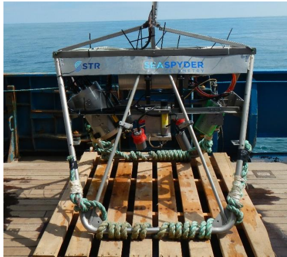
Figure 2. STR SeaSpyder drop frame camera system.
