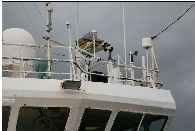
Figure 3. Locations of the FSSP, OAP, and AWS (above). Close up of FSSP, OAP (below).
