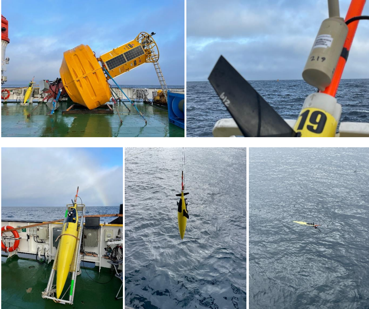
SG-219 next to the PAPI surface buoy during self-tests on the day of deployment and deployment shots later that morning.
