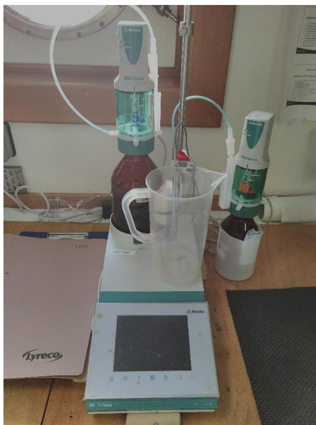
The Metrohm Ti-touch 916 setup used for dissolved oxygen analysis on DY130.
