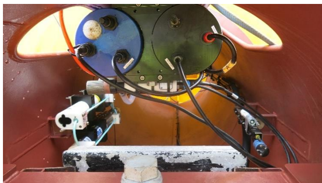
Photo shows 2 microCATs, Atmos CO2 (to right) and blue CO2 Pro plus optode and Starmon sensor in Buoy DY130
