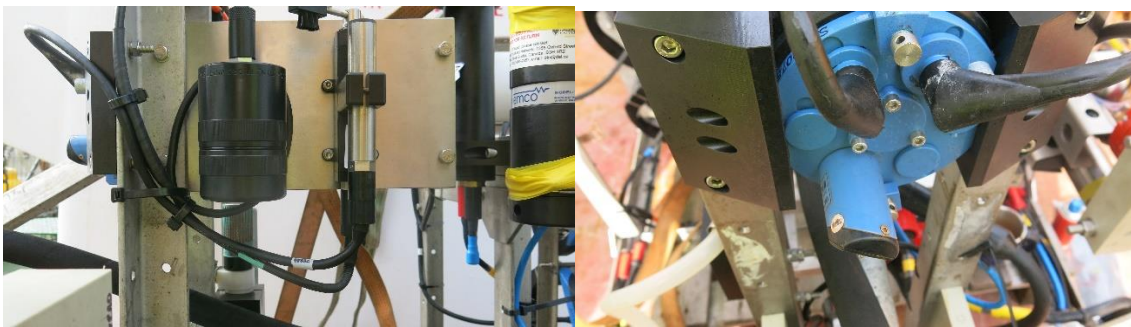
Photos of the Turner fluorometer and optode on the seaguard
