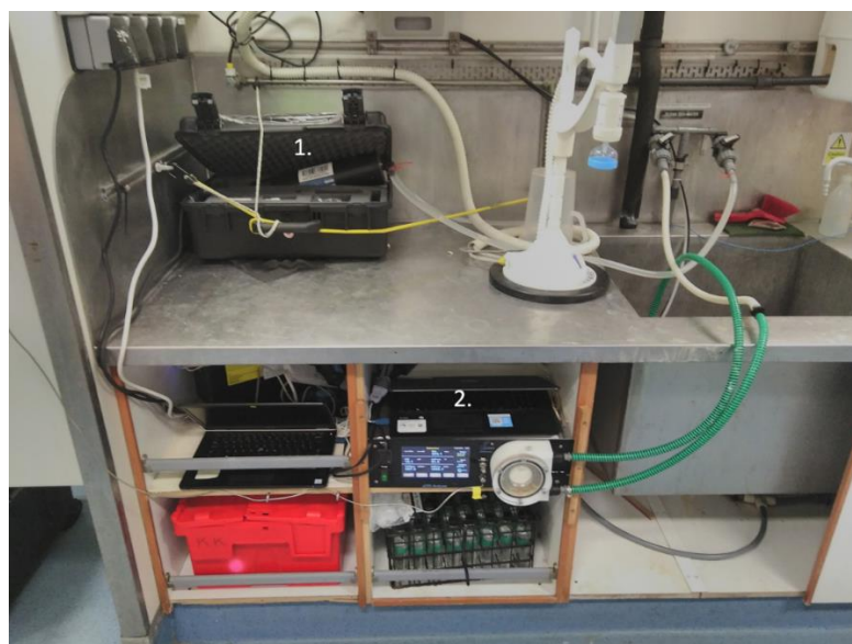
ProOceanus CV (1.) and SubCtech (2.) connected to the non-toxic seawater supply during DY130
