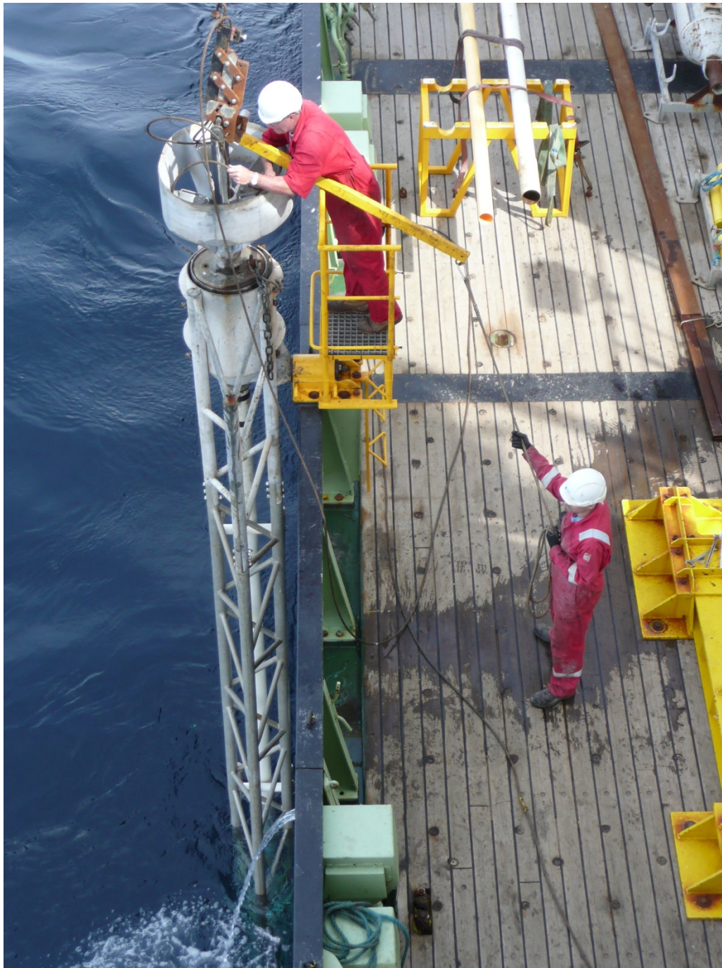
Figure 11. Deployment of NMFSS piston corer, North Sea.
