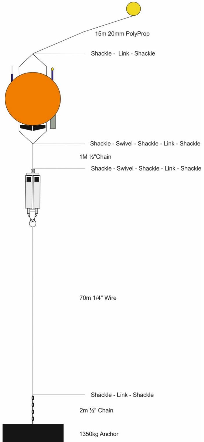
**Figure 8.1.** Diagram of NERC Mooring-8.
