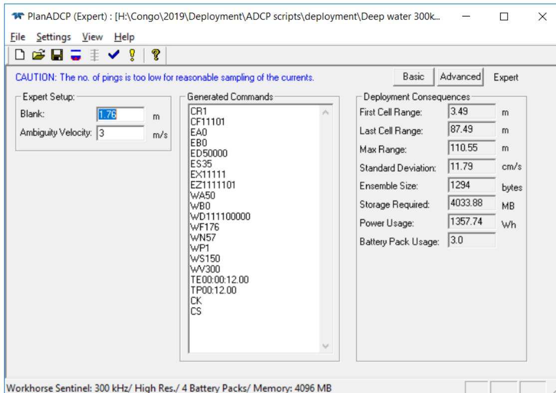
**Figure 8.13:** Settings for 300 kHz ADCPs on NERC Moorings M5, M6, M7, and M8 (first deployment), located 80 m above seafloor.
