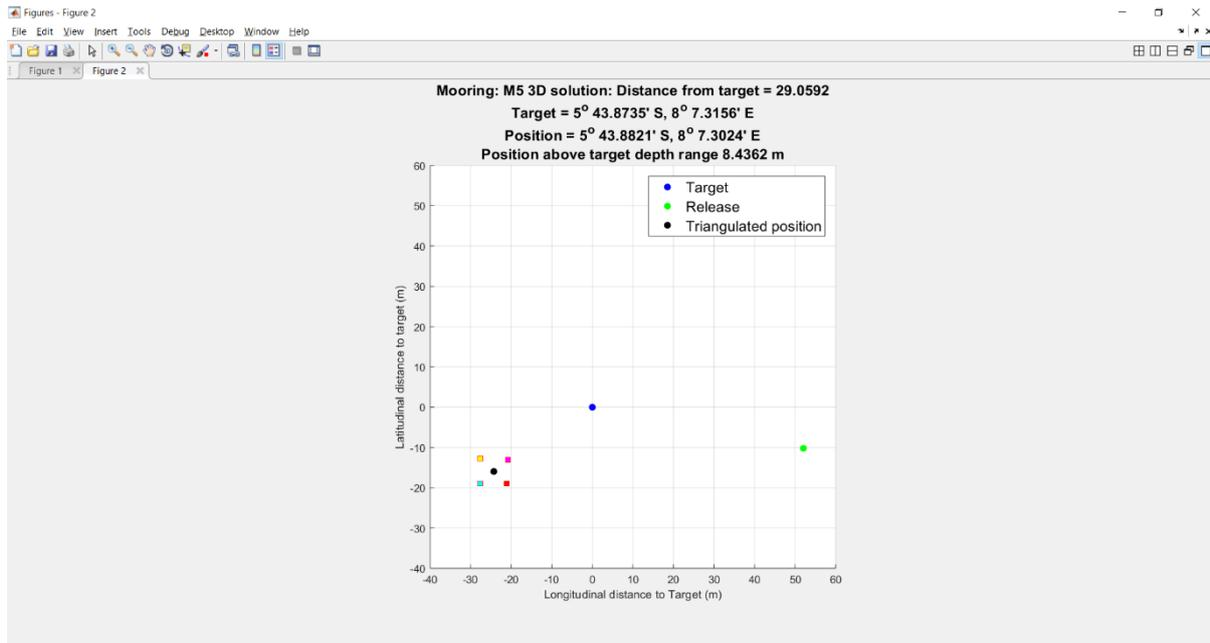
**Figure 8.58.** Target, release, triangulated position and distance from target of the NERC Mooring M5 determined by averaging the four direct trigonometric solutions (squares).
