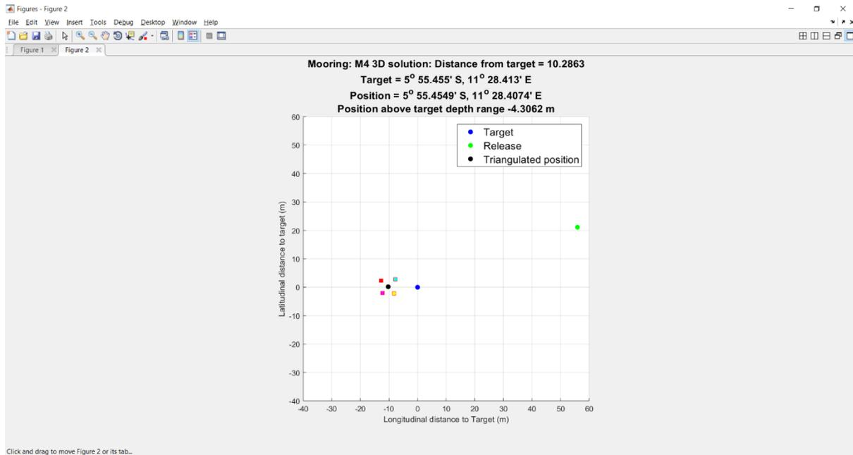
**Figure 8.43.** Target, release, triangulated position and distance from target of the NERC Mooring M4 determined by averaging the four direct trigonometric solutions (squares).
