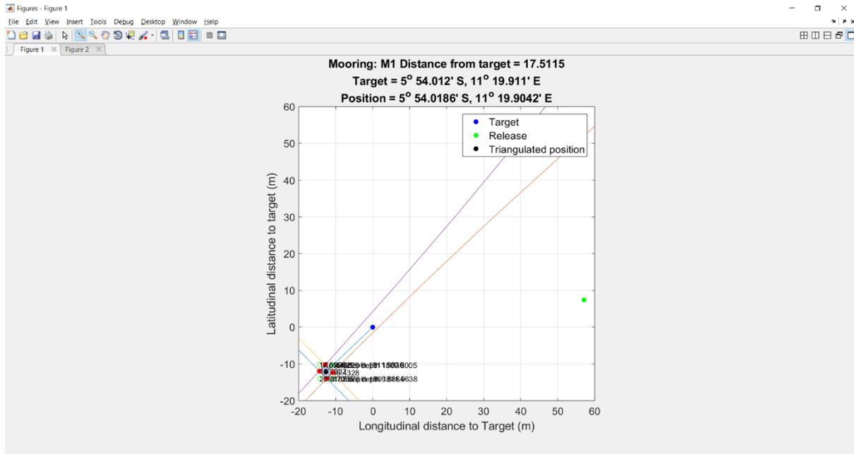
**Figure 8.38.** Target, release and triangulated position of NERC Mooring M1 determined using the centroid of the intersection (shaded blue) of four range circles.
