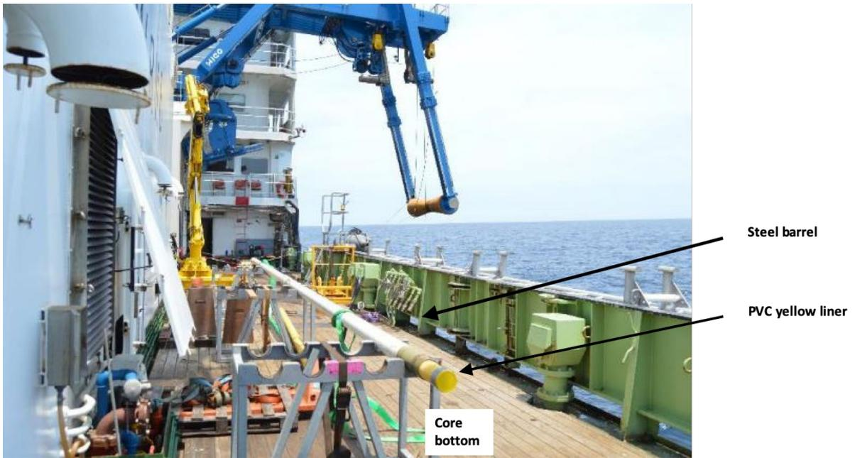
**Figure 8.72.** Core on stand, ready to be removed from the steel tube barrel and split into sections
