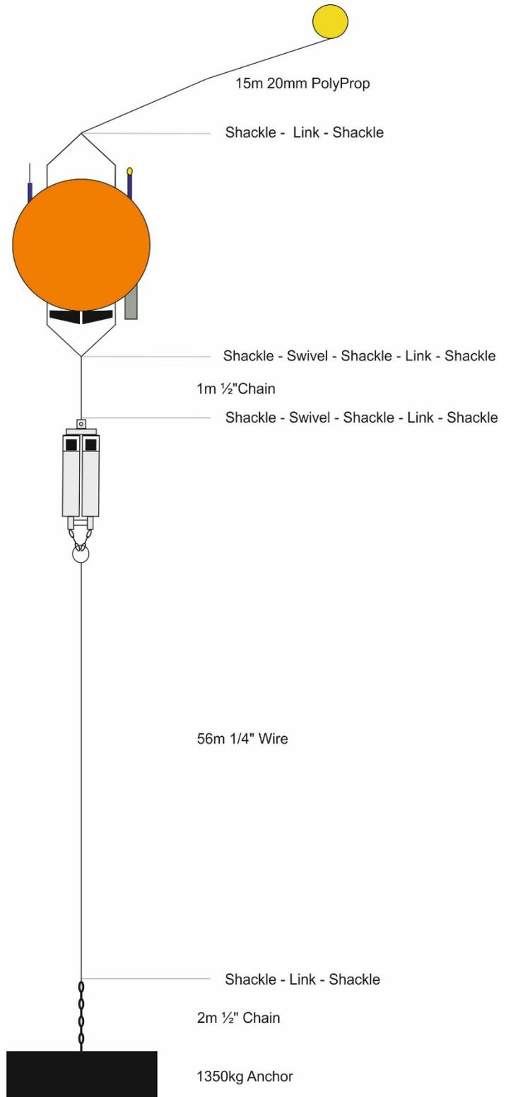
Figure 8.4. Diagram of NERC Mooring-1.
