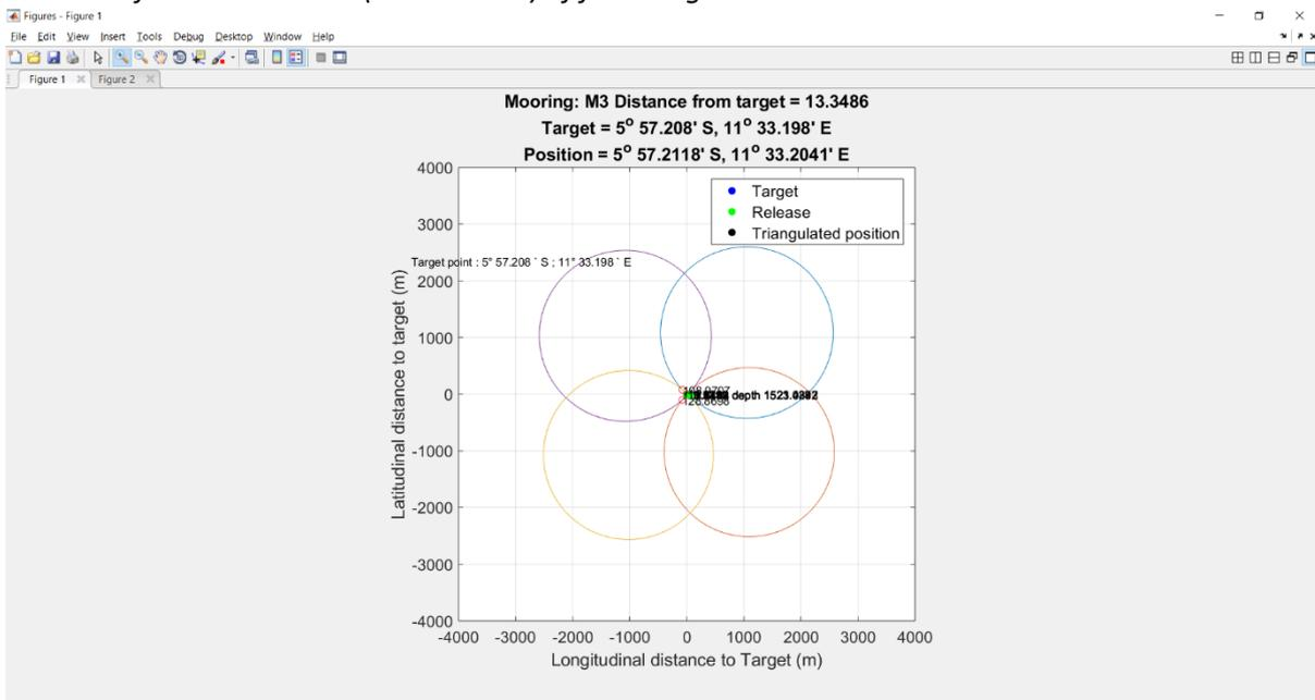
**Figure 8.45.** Zoom out of previous figure showing the full extent of the range circles from the four ranging positions.
