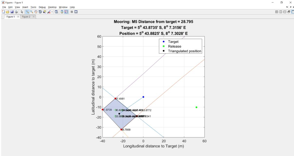
**Figure 8.56.** Target, release and triangulated position of NERC Mooring M5 determined using the centroid of the intersection (shaded blue) of four range circles.
