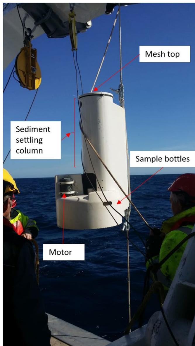
**Figure 8.22.** Photograph of the sediment trap on the Anitra mooring during deployment.
