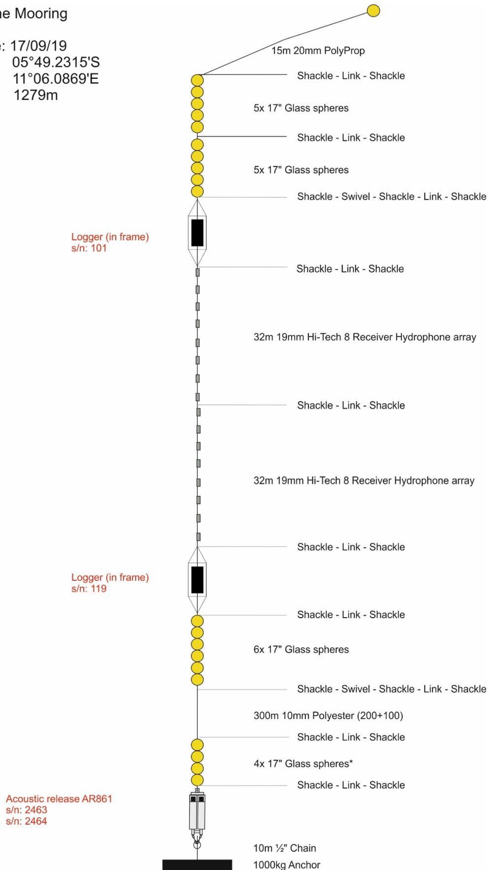
Figure 8.3. Diagram of Vertical Hydrophone Array (for initial test deployment).
