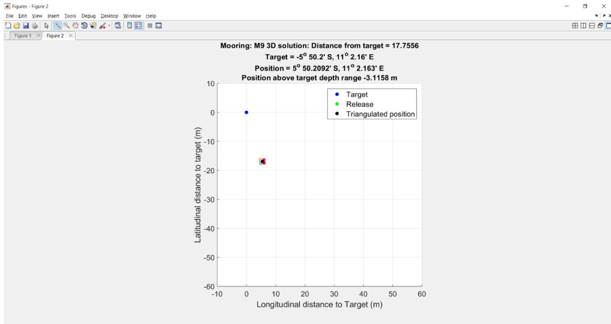
**Figure 8.49.** Target, release, triangulated position and distance from target of the NERC Mooring M9 determined by averaging the four direct trigonometric solutions (squares).
