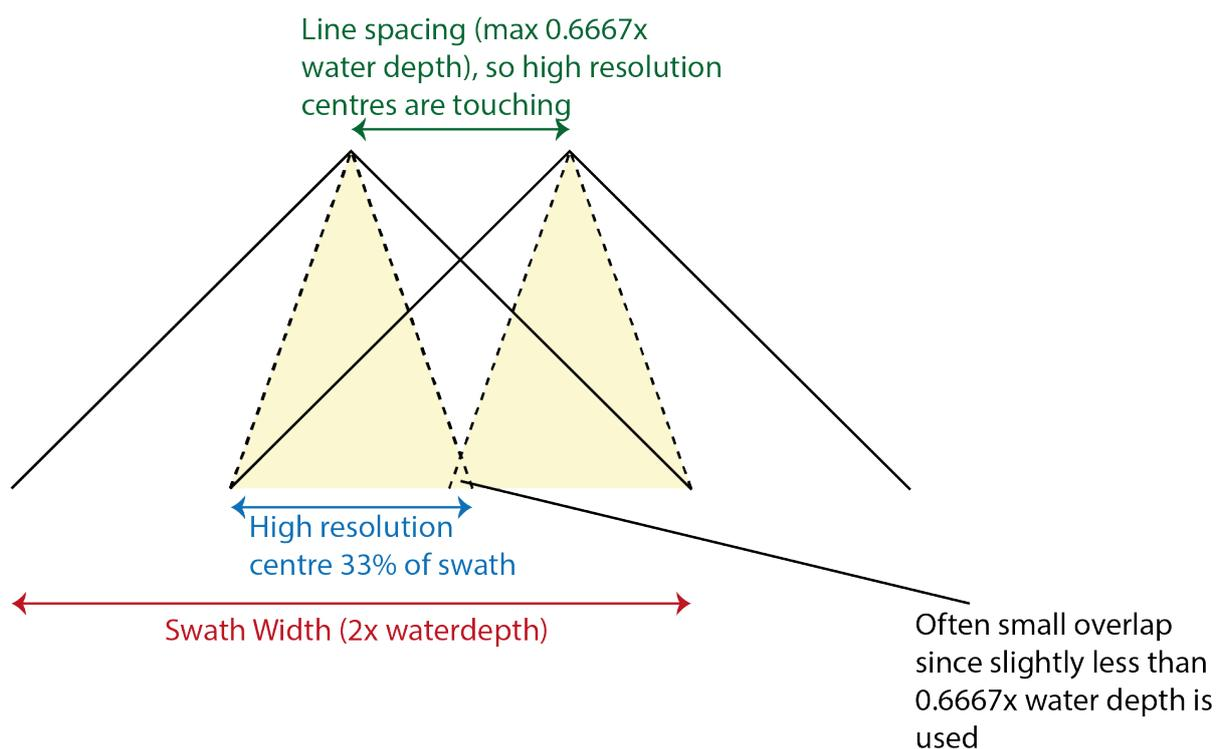
**Figure 8.65.** Schematic diagram explaining how the desired overlap was determined.
