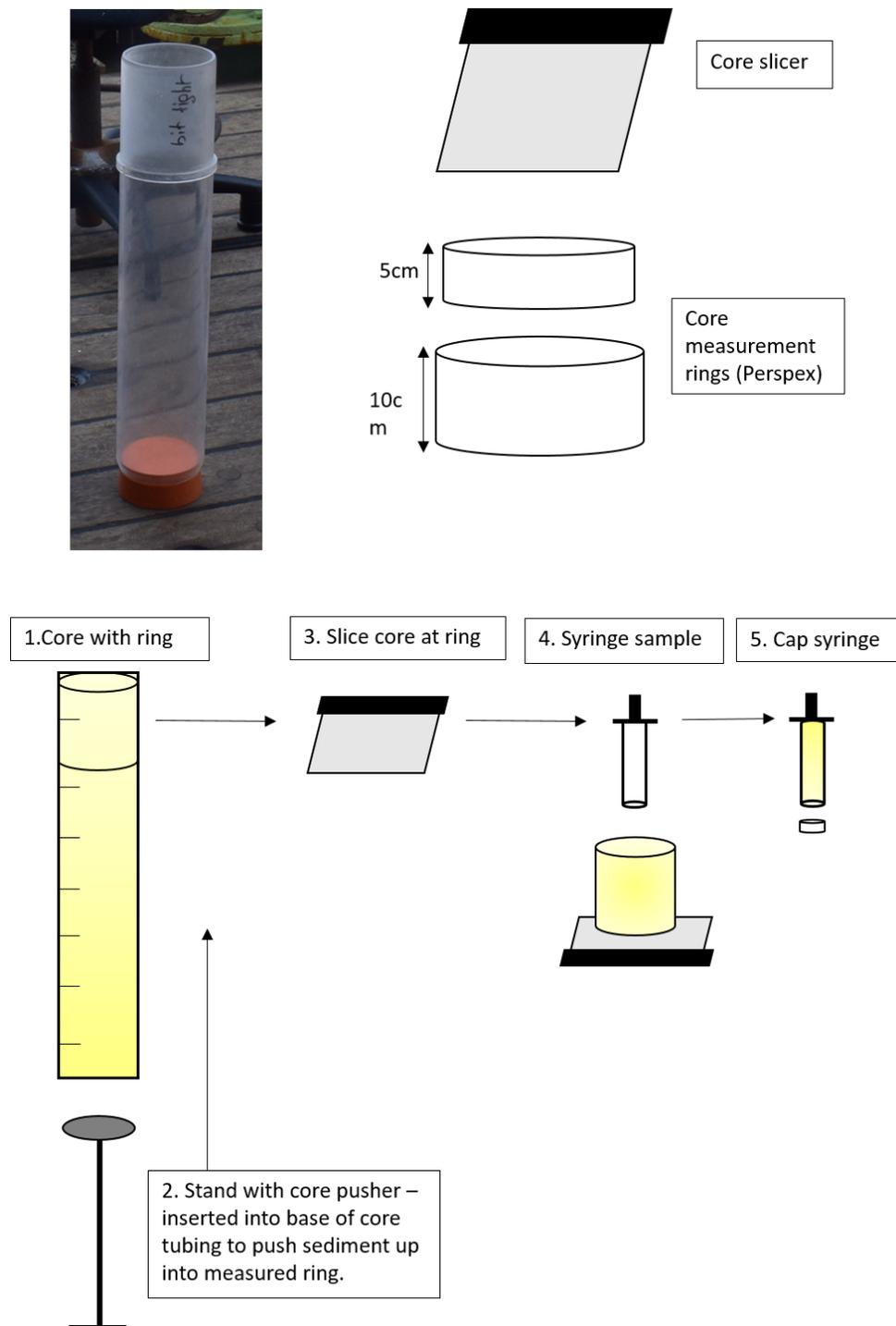
**Figure 8.79:** Method to subsample cores for EPS and clay. See text for details.
