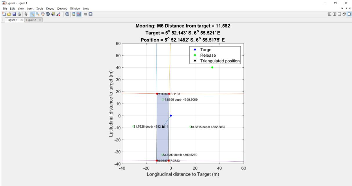
**Figure 8.59.** Target, release and triangulated position of NERC Mooring M6 determined using the centroid of the intersection (shaded blue) of four range circles.
