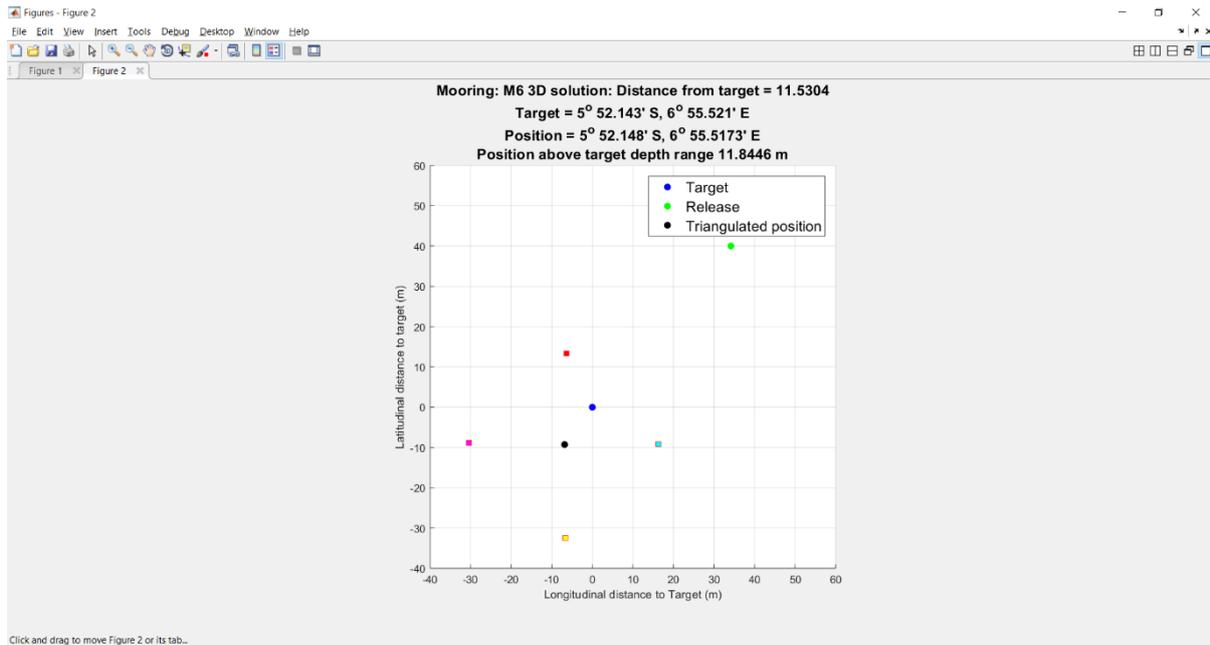
**Figure 8.61.** Target, release, triangulated position and distance from target of the NERC Mooring M6 determined by averaging the four direct trigonometric solutions (squares).
