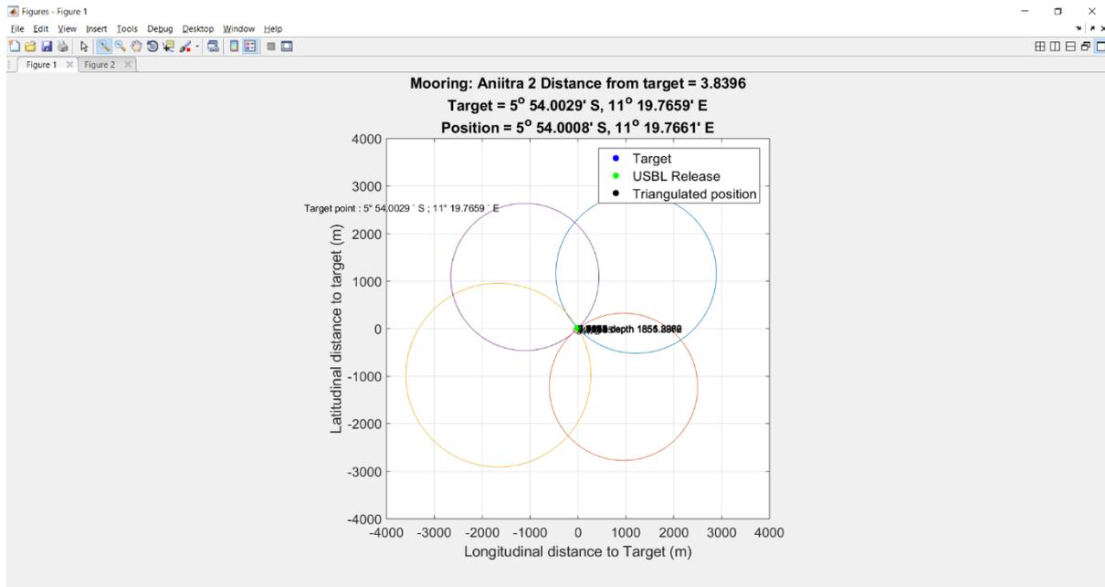
**Figure 8.36.** Zoom out of previous figure showing the full extent of the range circles from the four ranging positions.
