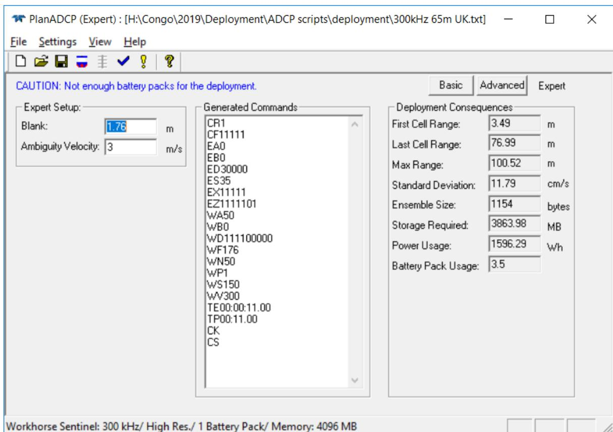
Figure 8.15: Settings for 300 kHz ADCPS on NERC moorings M1, M2, M3 and M4, 65 m above seafloor.
