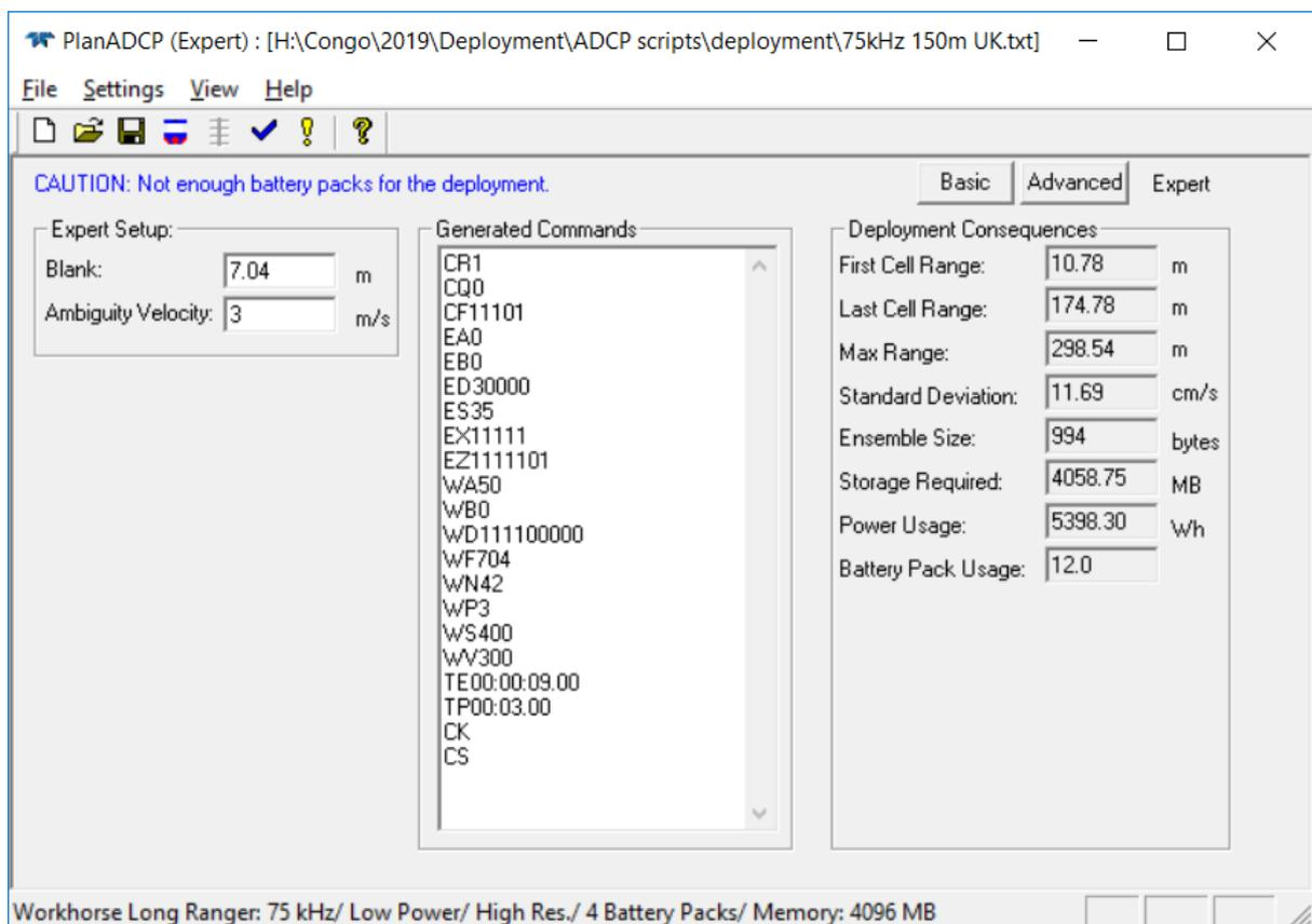
**Figure 8.17:** Settings for 75 kHz ADCP on NERC mooring M2, located 150 m above seafloor
