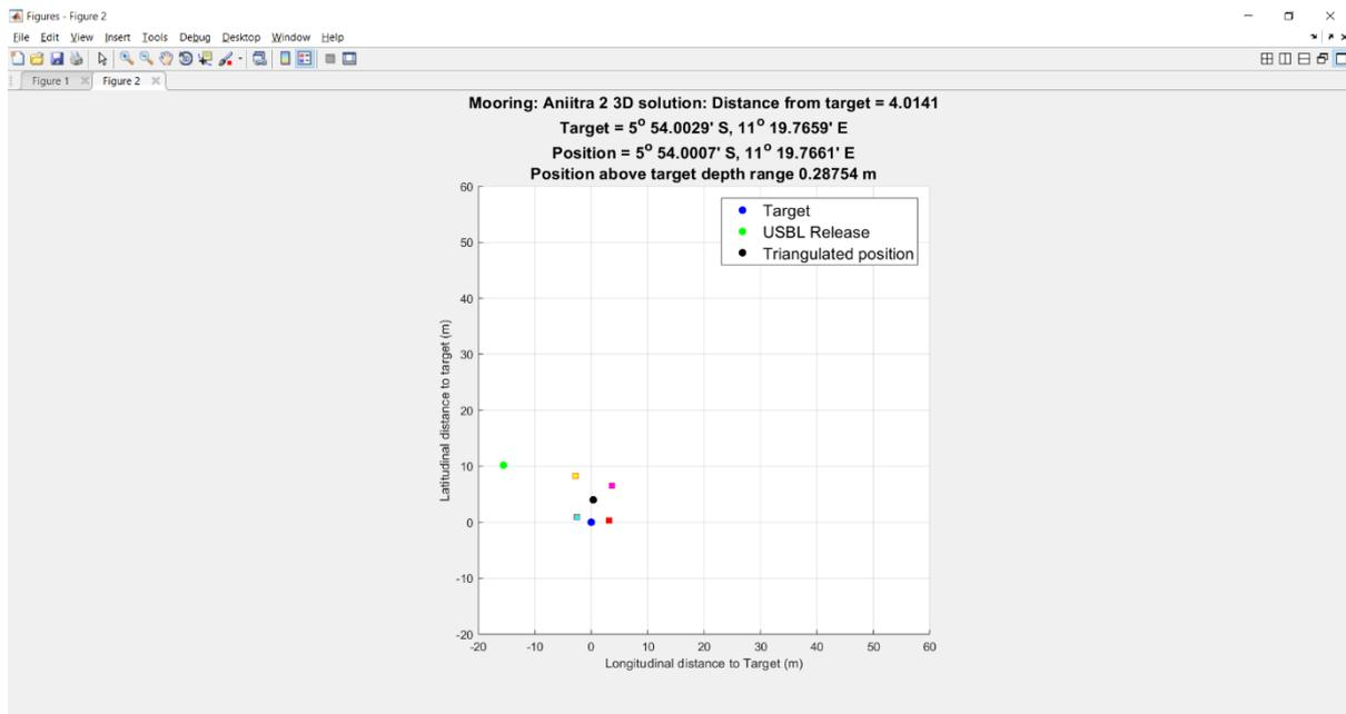
**Figure 8.37.** Target, release, triangulated position and distance from target of the Anitra 2 mooring determined by averaging the four direct trigonometric solutions (squares).
