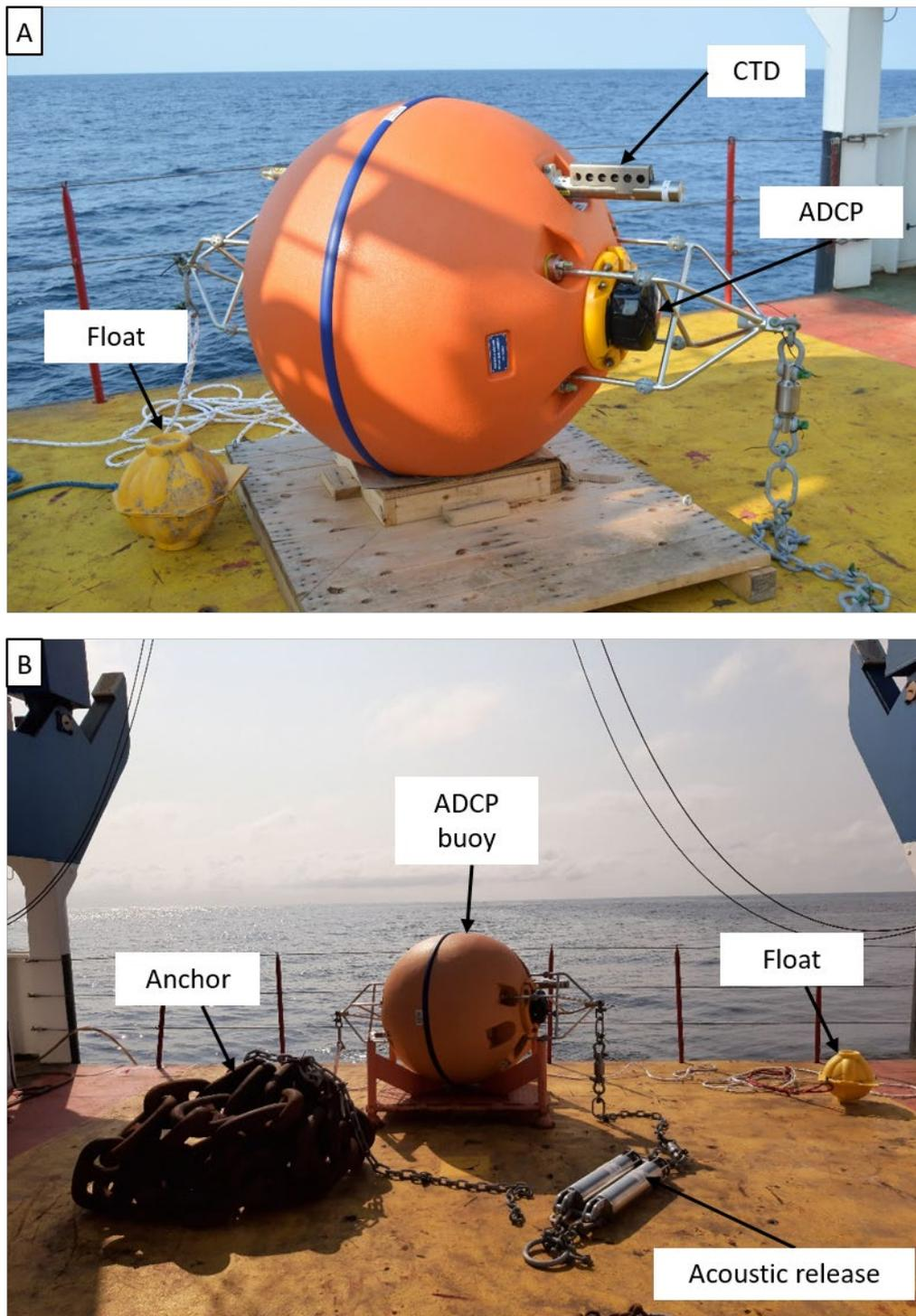
Figure 8.20: Components within the moorings.
