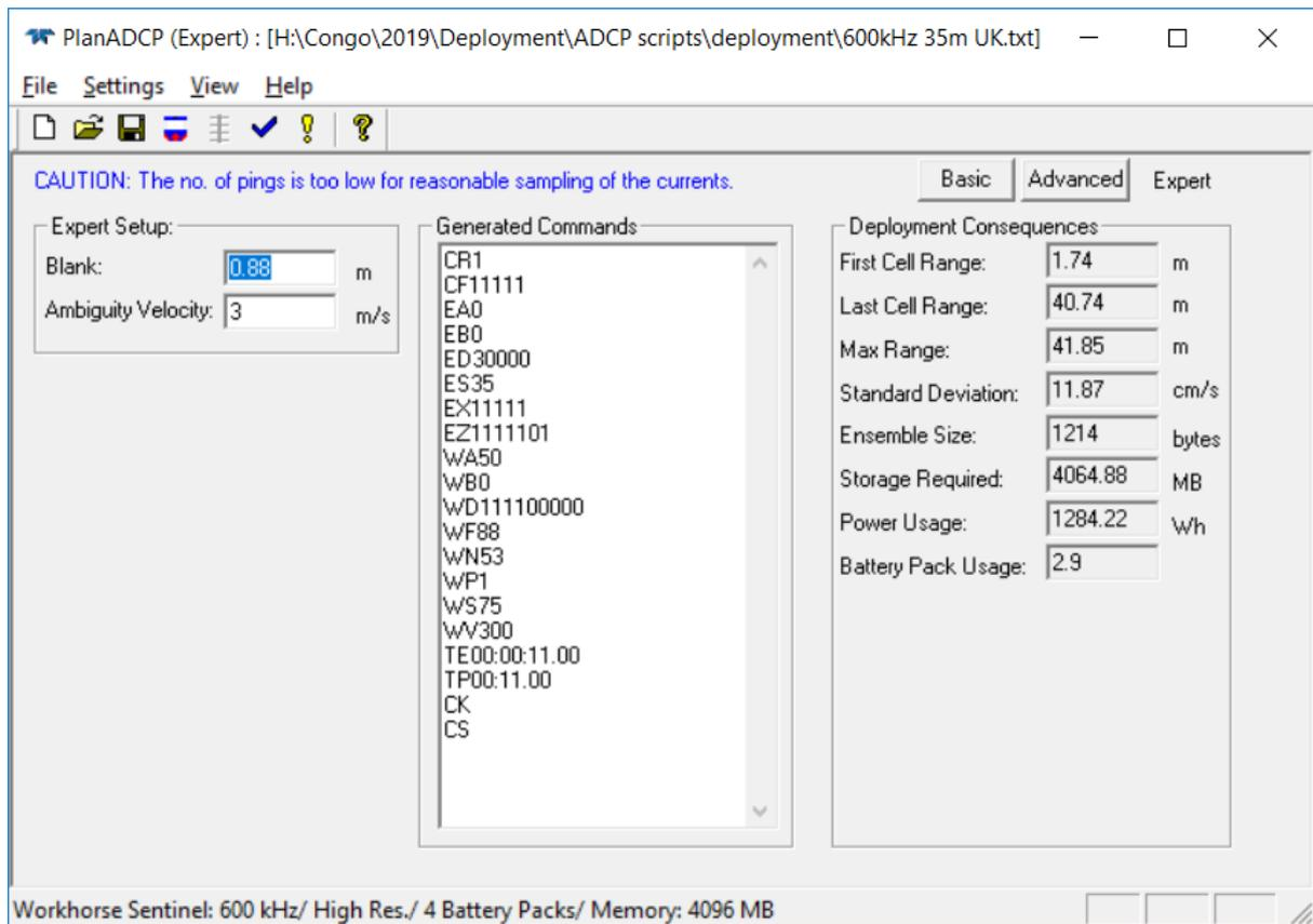
**Figure 8.16:** Settings for 600 kHz ADCP on NERC mooring M9, located 65 m above seafloor
