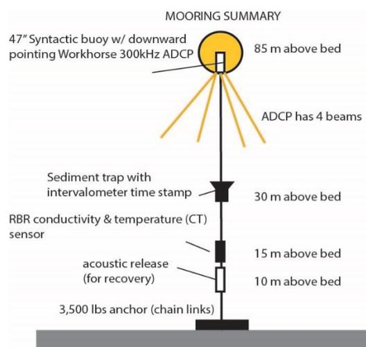
**Figure 1.3:** Diagram illustrating a typical mooring design with buoyancy (syntactic buoy), 300 kHz ADCP, sediment trap, CTD sensor and anchor chain. The mooring is lowered (anchor first) to the seabed, and then recovered by triggering the acoustic release from the ship, such that the mooring floats back to the surface.
