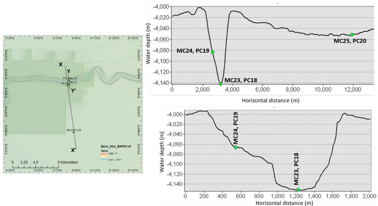
**Figure 9.22:** Zoom-in and cross sections showing the locations of MC23 to 25 and PC 18 to 20.
