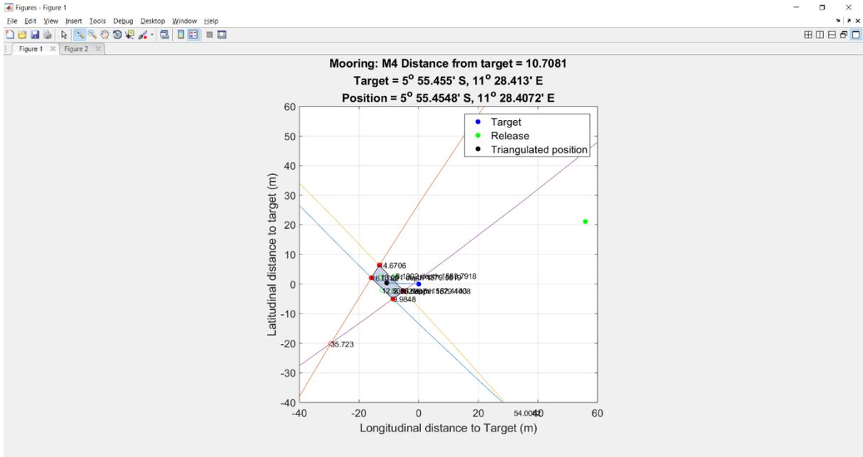
**Figure 8.41.** Target, release and triangulated position of NERC Mooring M4 determined using the centroid of the intersection (shaded blue) of four range circles.
