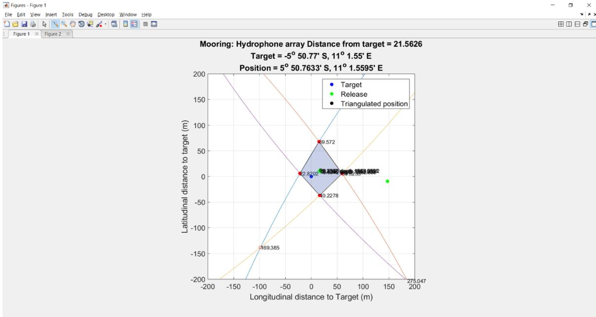
**Figure 8.50.** Target, release and triangulated position of the hydrophone array mooring determined using the centroid of the intersection (shaded blue) of four range circles.
