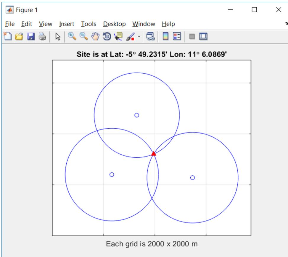
**Figure 8.32.** *Triangulation\_v6.m output showing target position, three ranging positions (blue circles), range circles (blue lines) for the triangulation of the hydrophone array experiment mooring.*
