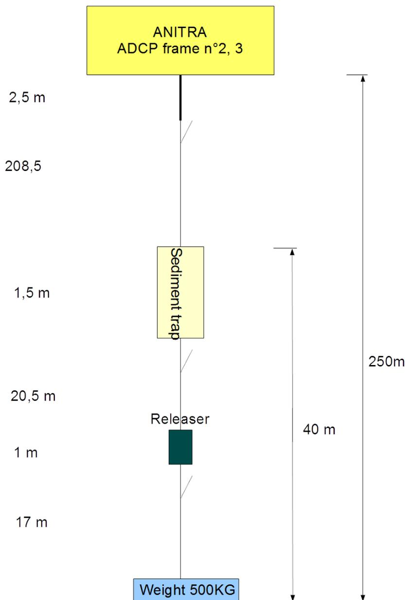
**Figure 8.23.** Technical drawing of the Anitra mooring design.
