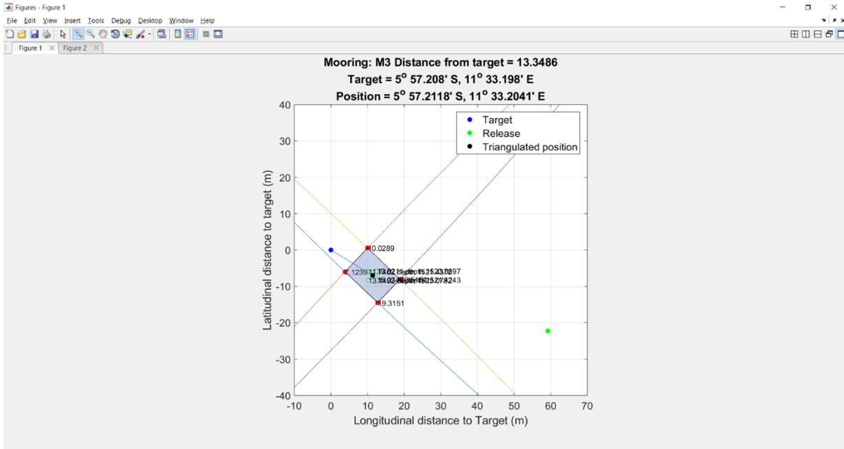
**Figure 8.44.** Target, release and triangulated position of NERC Mooring M3 determined using the centroid of the intersection (shaded blue) of four range circles.
