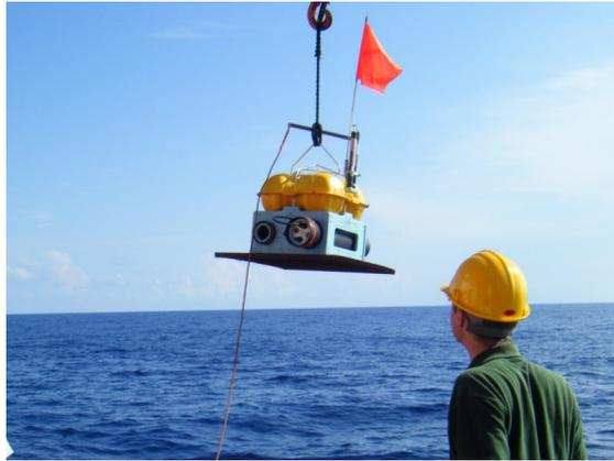
**Figure 1.4:** Deployment of an Ocean Bottom Seismometer (OBS) from a NERC vessel. The OBS is lowered to the seabed, and recovered via an acoustic release, triggered from the ship, which causes the OBS to float back to the sea surface (where it is collected).
