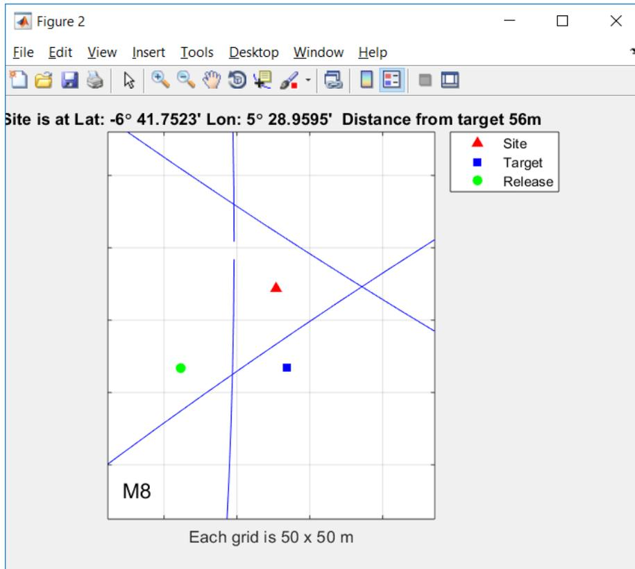
**Figure 8.27.** *Triangulation\_v6.m* output showing target position, release position and triangulated position of NERC Mooring M8.
