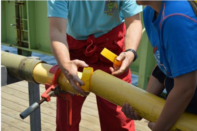
**Figure 8.74.** Caps are put at the ends of each section
