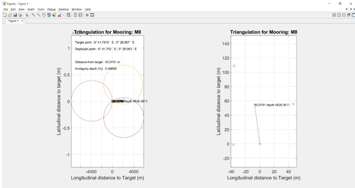
**Figure 8.28.** *Triangulo\_M8.m* output showing target position and triangulated position (left plot) and the distance from the target and the depth of the release determined by the direct trigonometric solution (right plot) for NERC Mooring M8.
