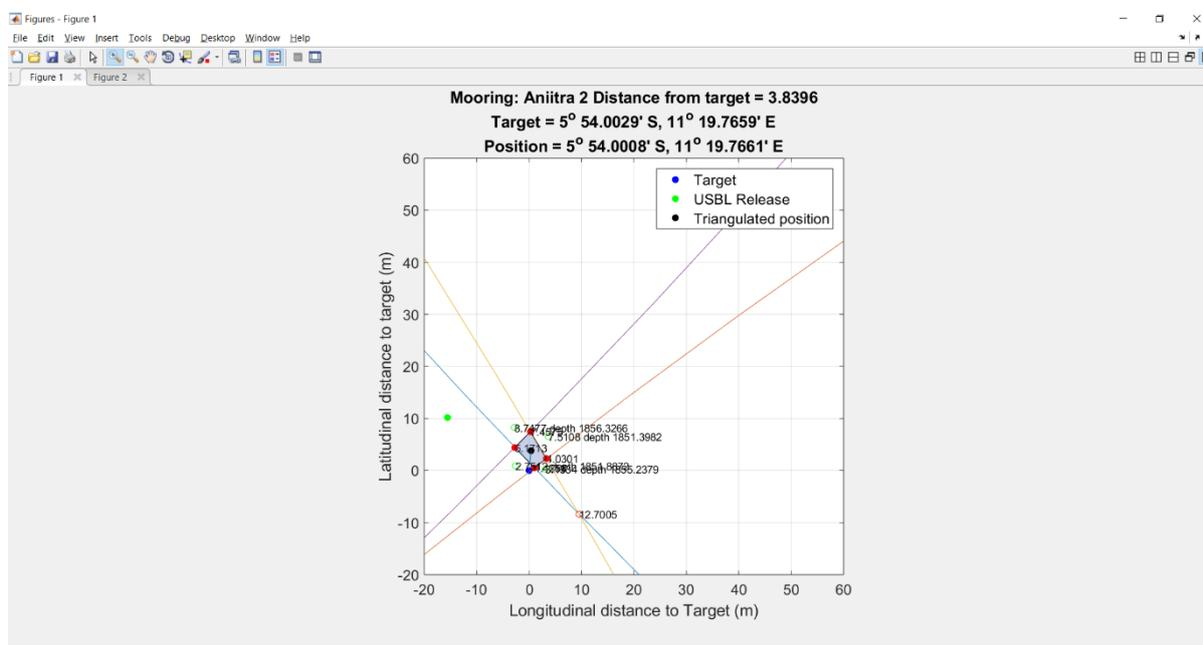
**Figure 8.35.** Target, release and triangulated position of the Aniitra 2 mooring determined using the centroid of the intersection (shaded blue) of four range circles.
