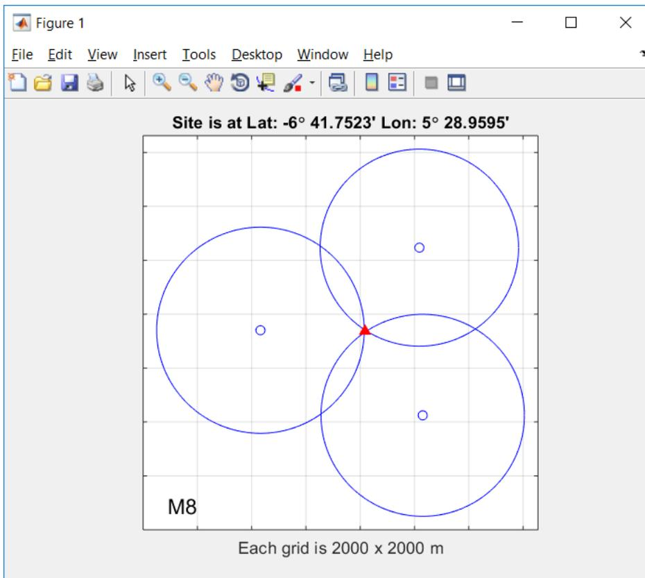
**Figure 8.26.** *Triangulation\_v6.m output showing target position, three ranging positions (blue circles), range circles (blue lines) for the triangulation of NERC Mooring M8.*
