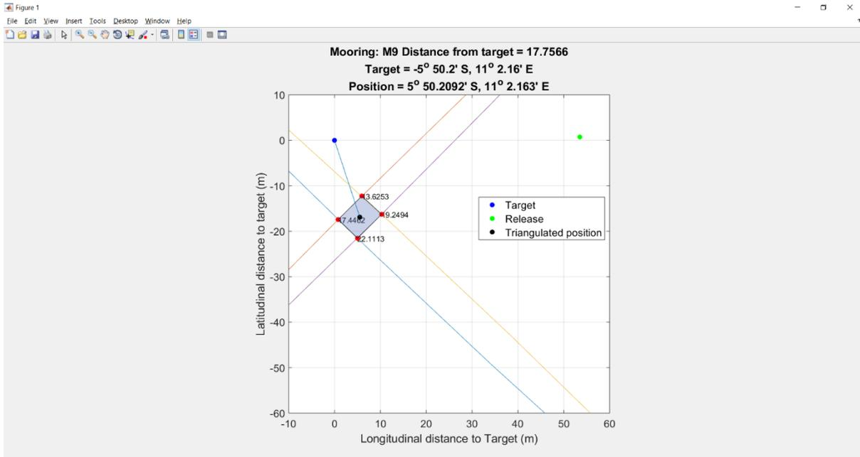
**Figure 8.47.** Target, release and triangulated position of NERC Mooring M9 determined using the centroid of the intersection (shaded blue) of four range circles.
