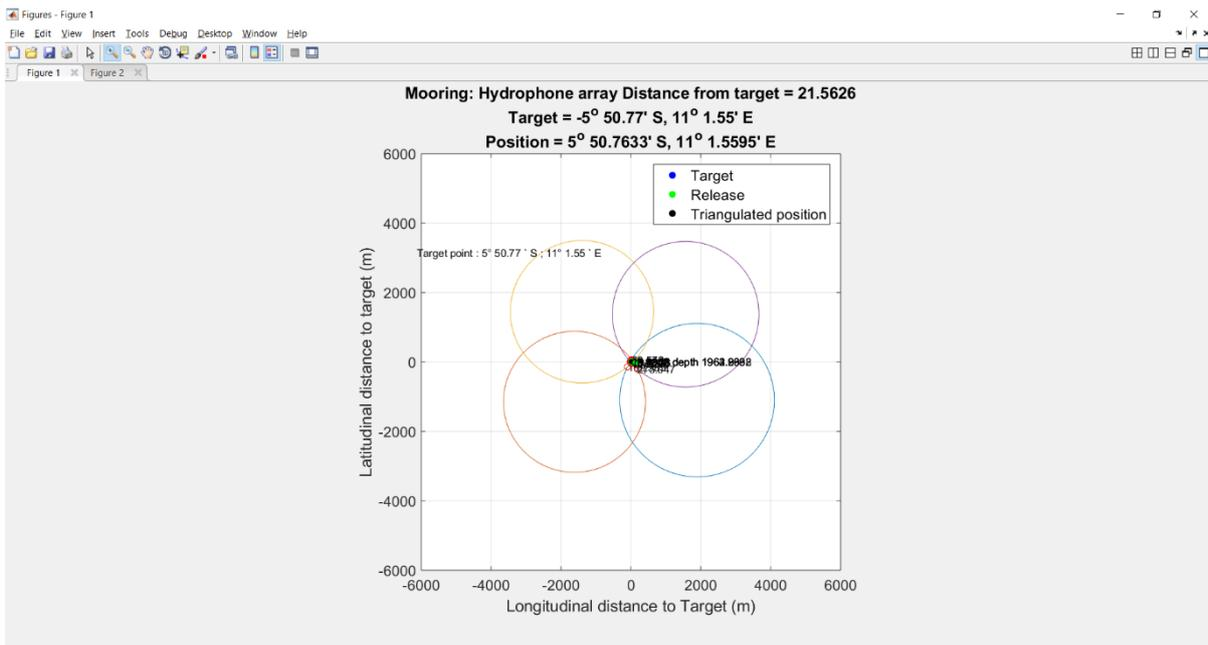
**Figure 8.51.** Zoom out of previous figure showing the full extent of the range circles from the four ranging positions.
