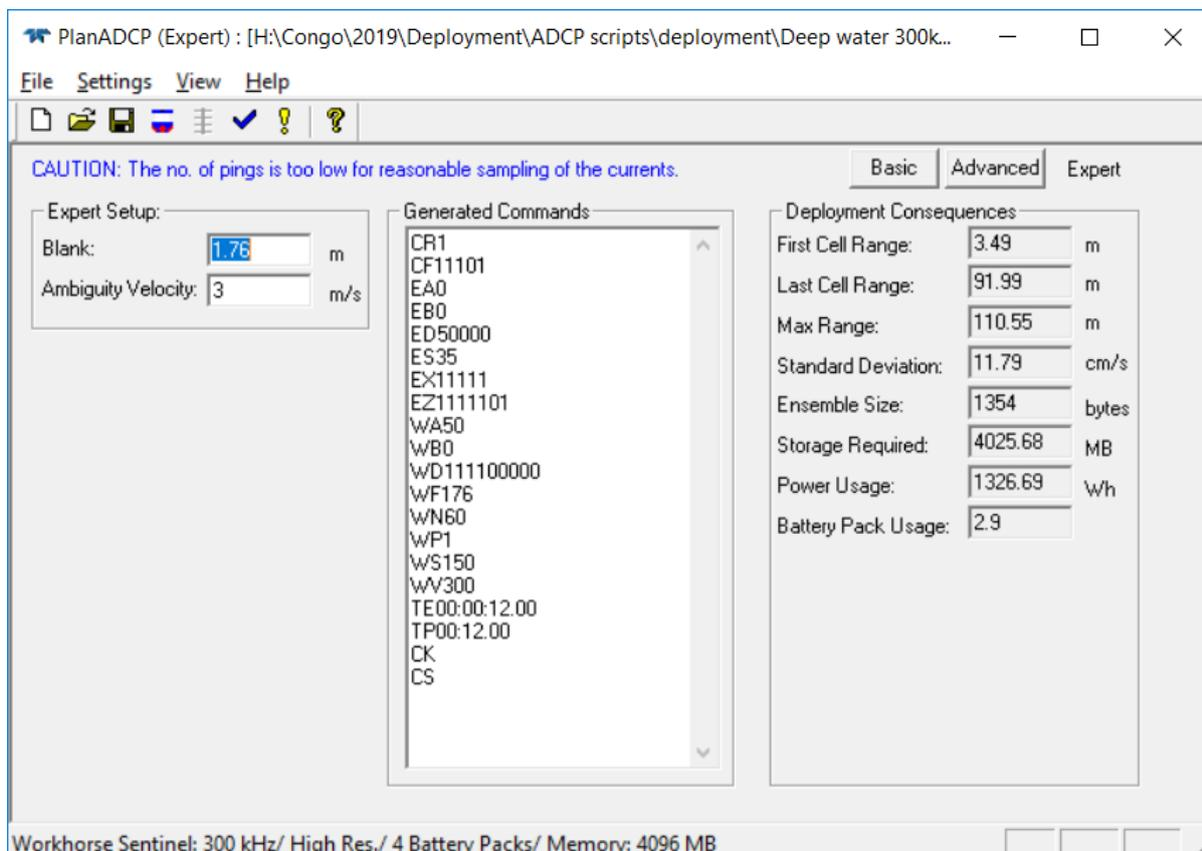
Figure 8.14: Settings for 300 kHz ADCPs on NERC Mooring M8-R (re-deployment), 80 m above seafloor.
