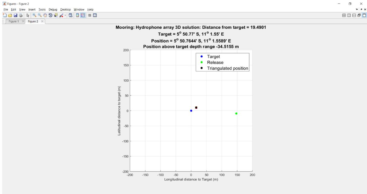
**Figure 8.52.** Target, release, triangulated position and distance from target of the hydrophone array determined by averaging the four direct trigonometric solutions (squares).
