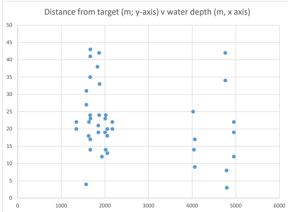
Fig. D-1. Distance from USBL on corer from original coordinates of target given to the bridge.
