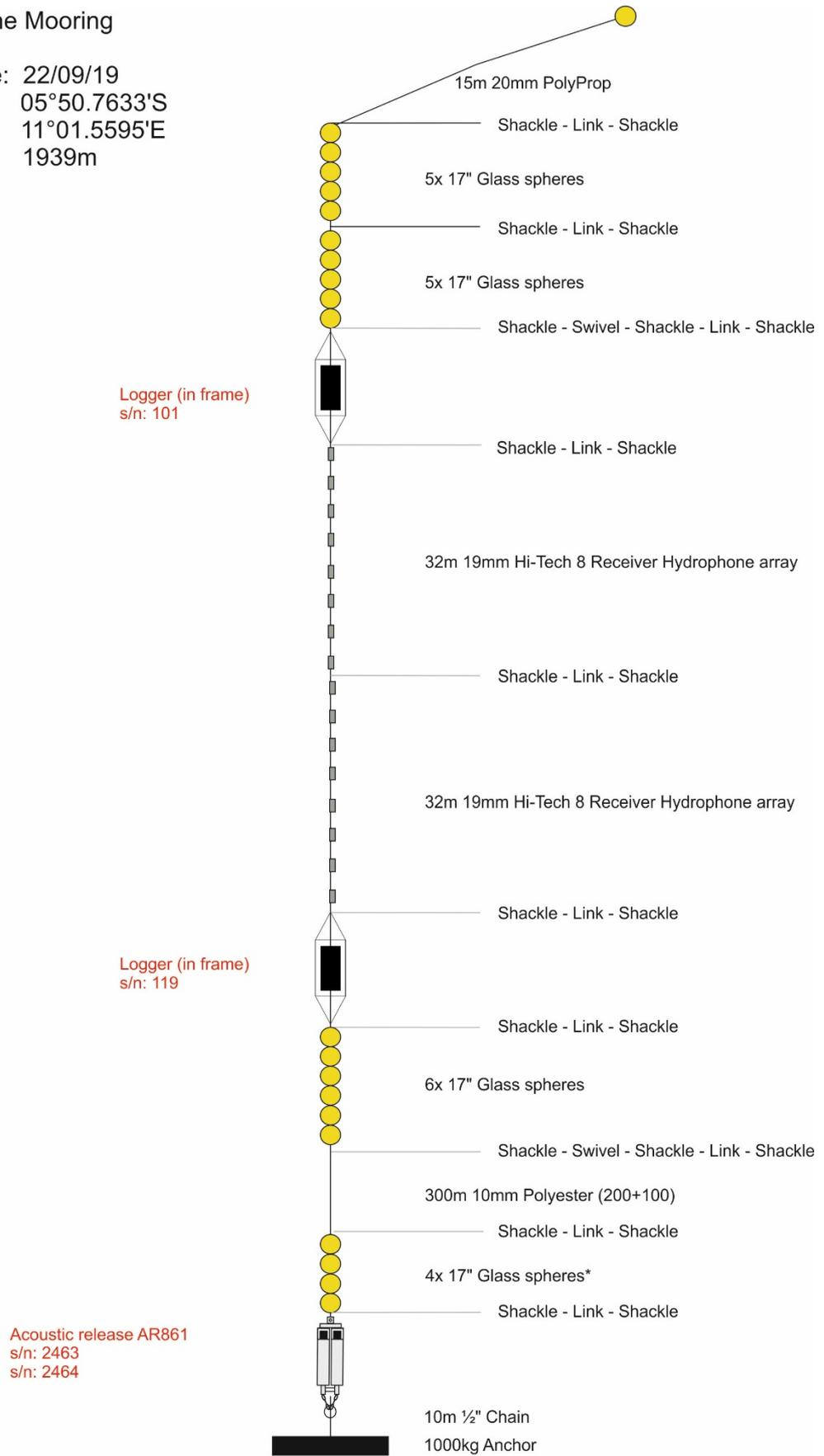
Figure 8.8. Diagram of Vertical Hydrophone Array (final deployment).
