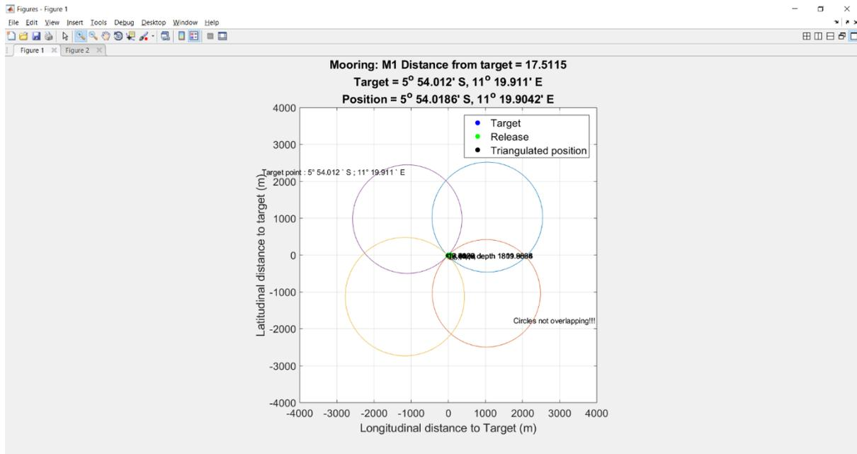
**Figure 8.39.** Zoom out of previous figure showing the full extent of the range circles from the four ranging positions.
