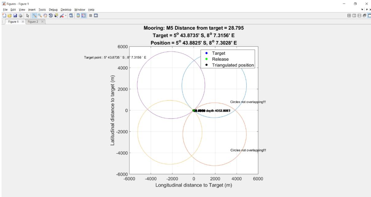
**Figure 8.57.** Zoom out of previous figure showing the full extent of the range circles from the four ranging positions.
