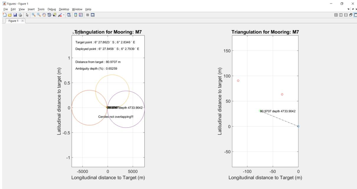
**Figure 8.30.** *Triangulo\_M7.m* output showing target position and triangulated position (left plot) and the distance from the target and the depth of the release determined by the direct trigonometric solution (right plot) for NERC Mooring M7.
