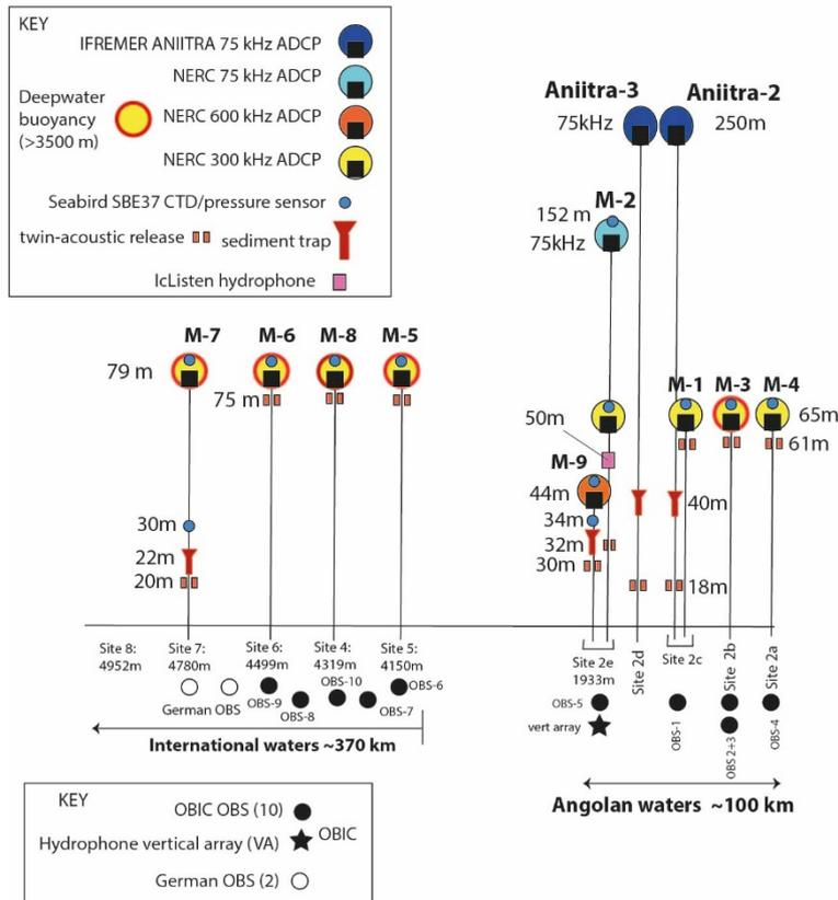
**Figure 1.2:** Summary of the planned array of moorings and other sensors along the Congo Submarine Canyon, from shallower water (right) to deeper water (left). The height of each sensor is marked in meters above the seabed. ADCPs (300, 600 or 75 kHz frequency) are shown as black squares, together with sediment traps, CTD (water temperature and salinity) sensors, single hydrophone, and the acoustic releases triggered to recover the moorings (see key).
