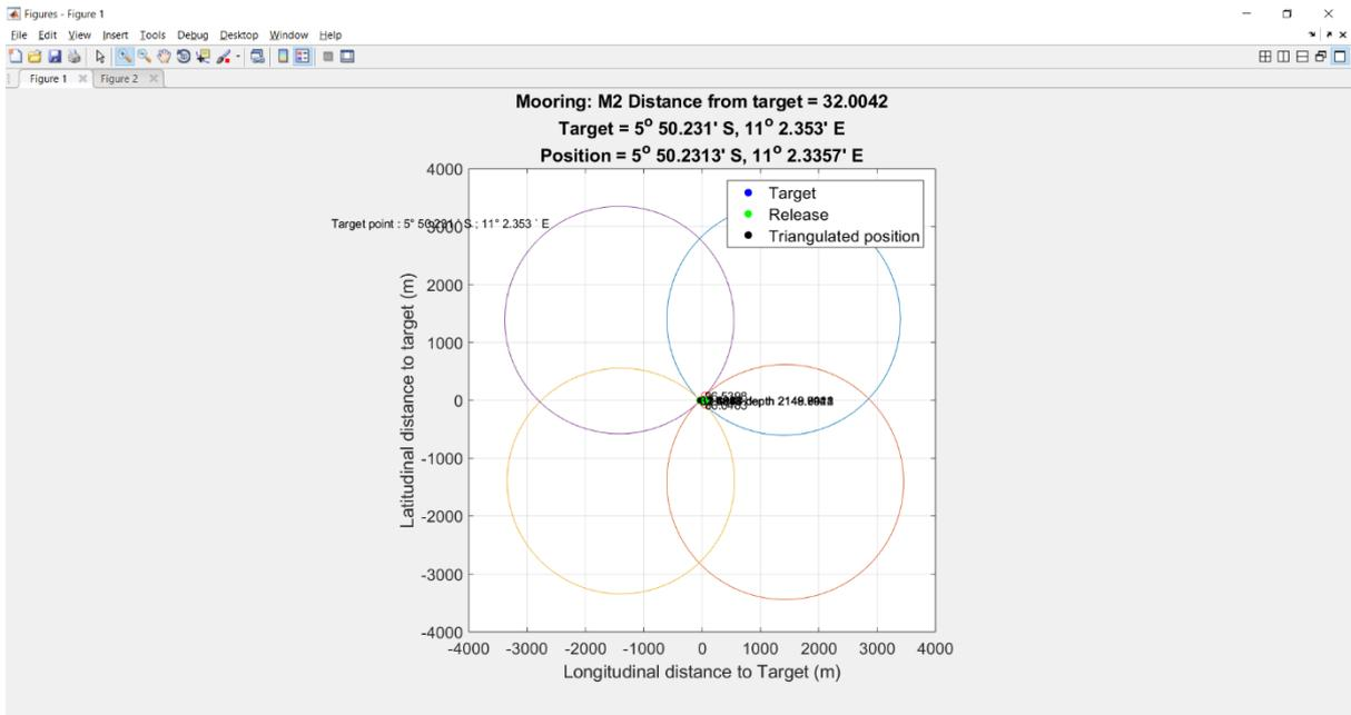
**Figure 8.54.** Zoom out of previous figure showing the full extent of the range circles from the four ranging positions.
