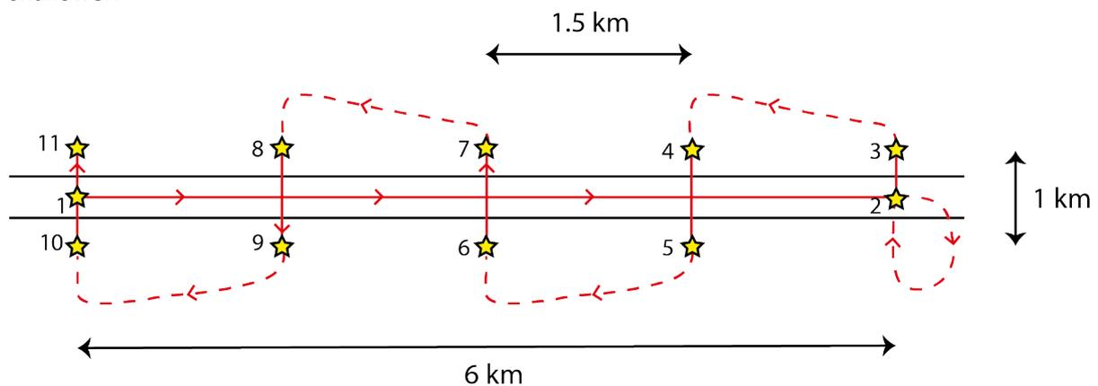
**Figure 8.66:** Idealised standard multibeam path layout. Yellow stars are the coordinates and solid red lines defined paths, communicated to the bridge. The dashed red lines are the paths followed by the bridge between the lines.
