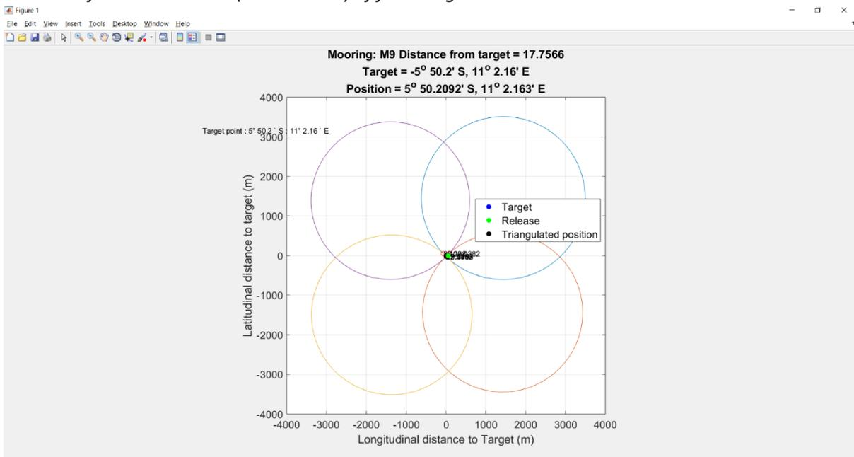
**Figure 8.48.** Zoom out of previous figure showing the full extent of the range circles from the four ranging positions.
