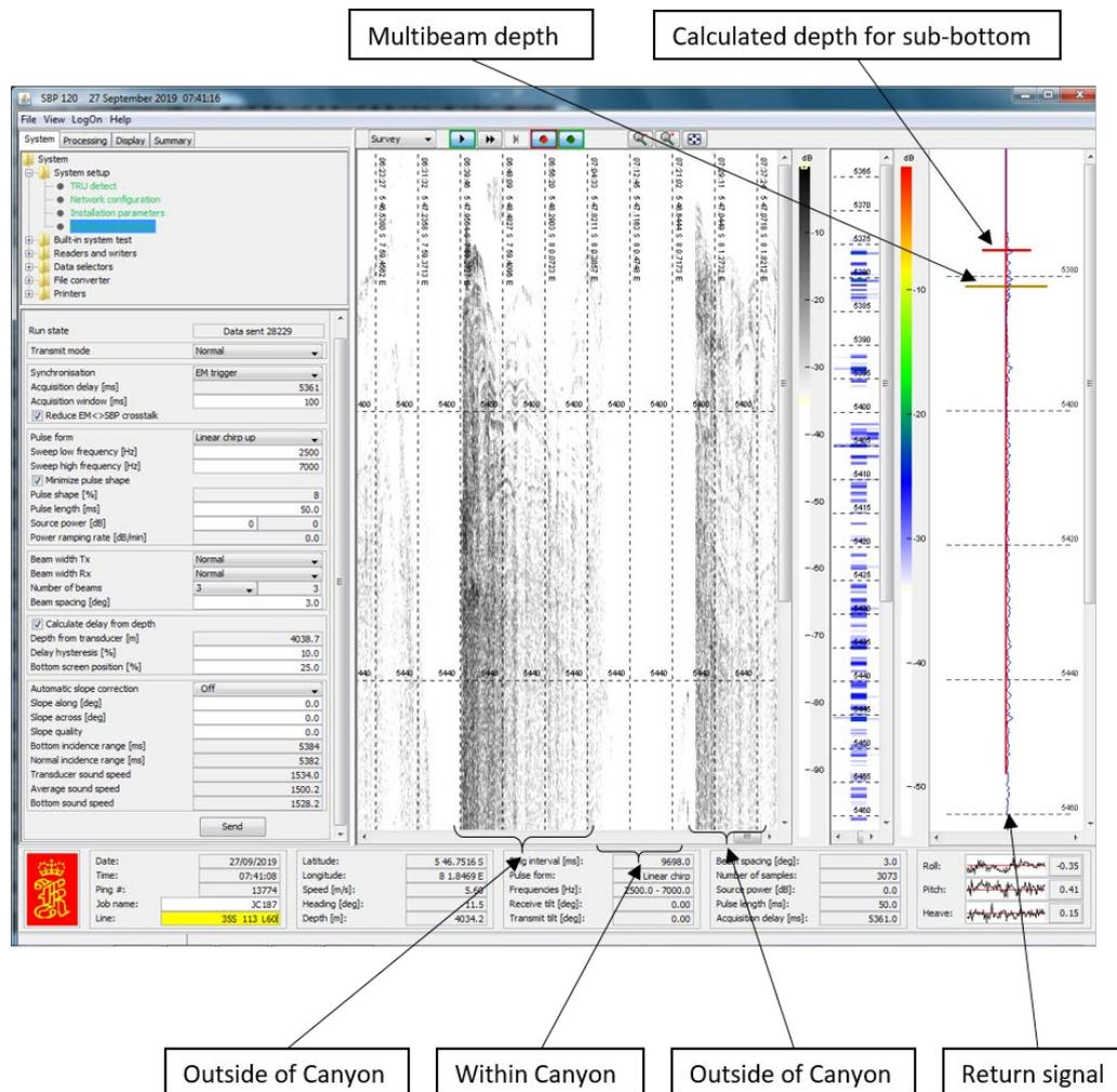
**Figure 8.68.** Sub-bottom profile screenshot showing the system settings, as well as the survey data as it is collected. Note the lack of return signal shown within the canyon (white), compared to the data collected outside of the canyon.
