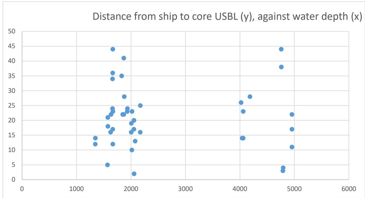
Fig. D-2. Distance of USBL on corer from the position of the ship (measured at the GRU in the Gravimeter Room – which is ~13m from where cores dropped) at time of release, against water depth.
