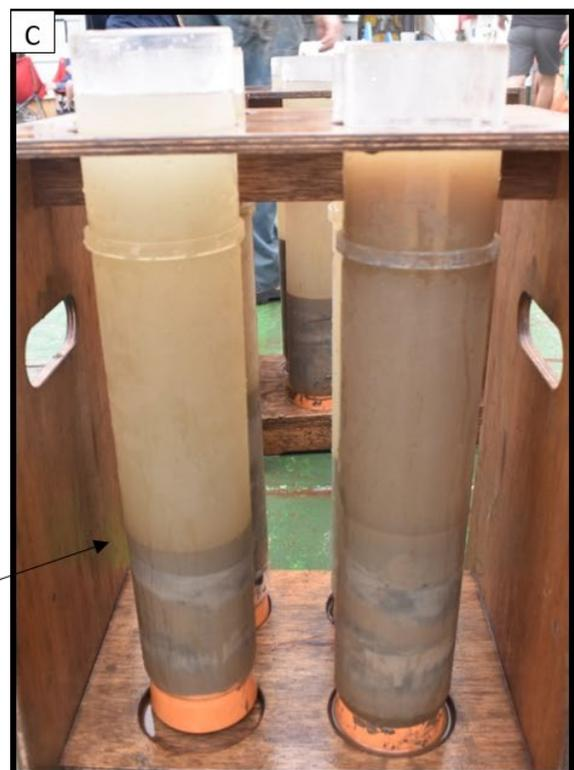
**Figure 8.76:** Sequence of events to obtain multicores: A) the multi-core prepared and ready to be deployed, B) Multicore back on deck, C) sediment cores are placed into the wooden rack with the bungs in place.
