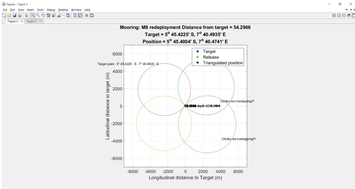
**Figure 8.63.** Zoom out of previous figure showing the full extent of the range circles from the four ranging positions.
