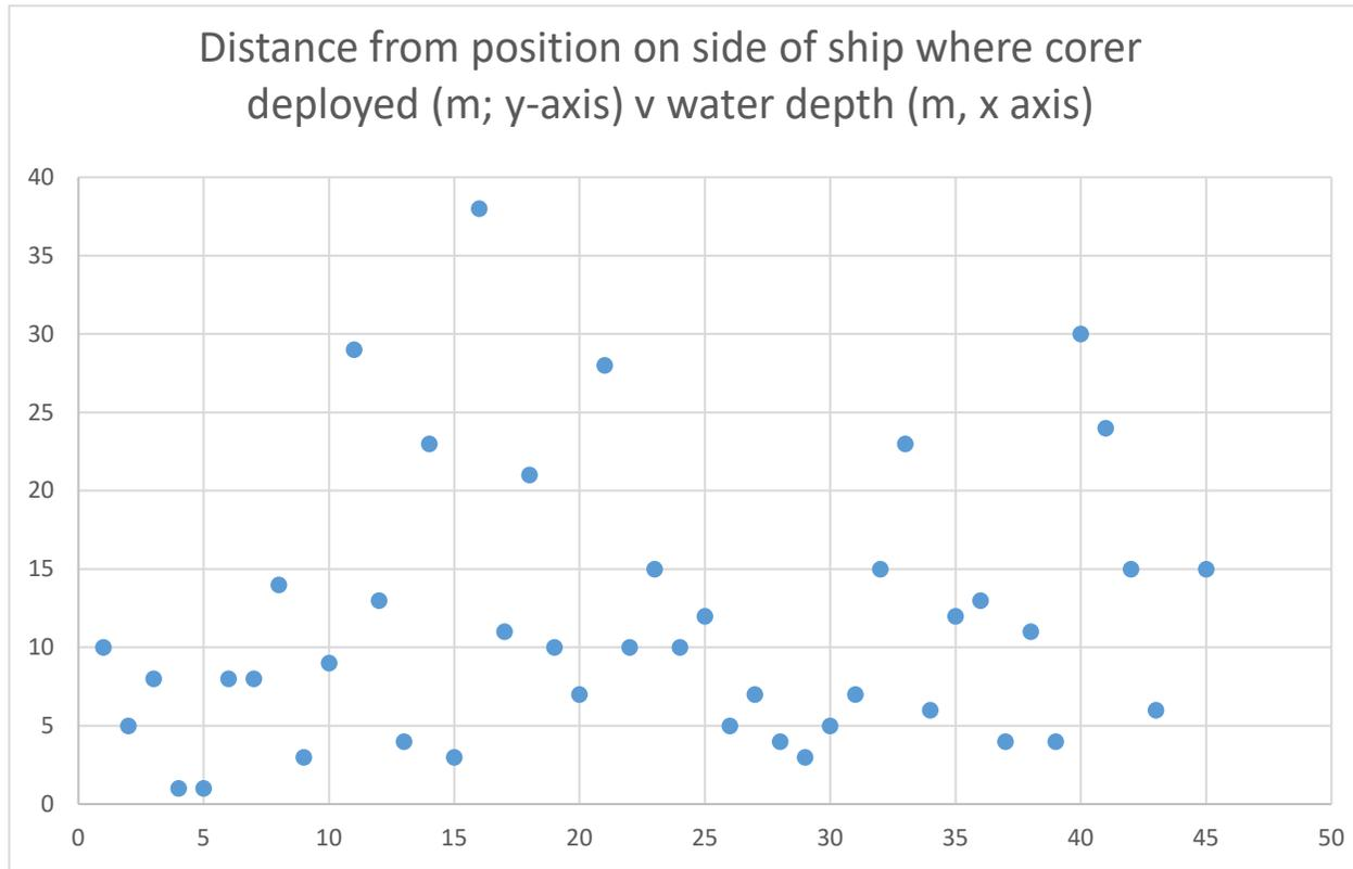
Figure D-3. Distance from the location of the corer on the ship’s starboard side to the USBL on the core (i.e. where core dropped). This includes adjustment of 13m at 120° from ship’s heading, from GPS position of ship (gravimeter room) to where the corer is located on the side of ship.
