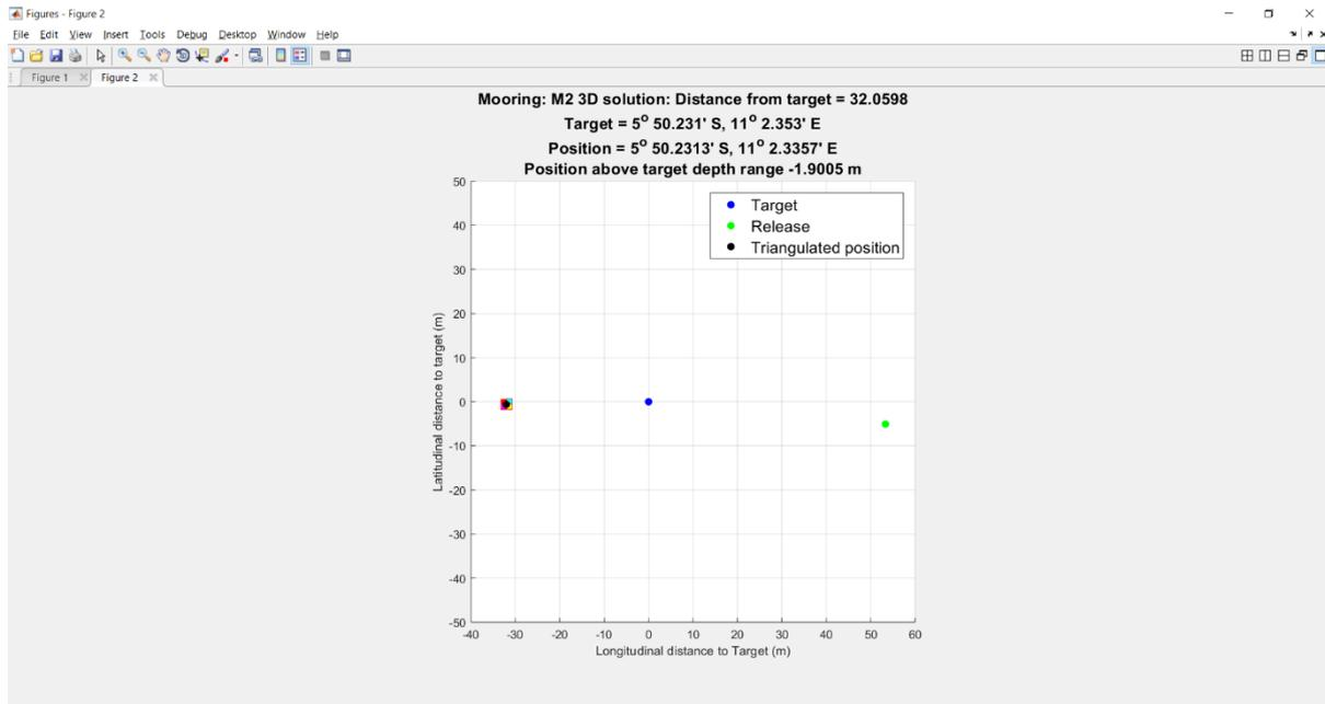
Figure 8.55. Target, release, triangulated position and distance from target of the NERC Mooring M2
