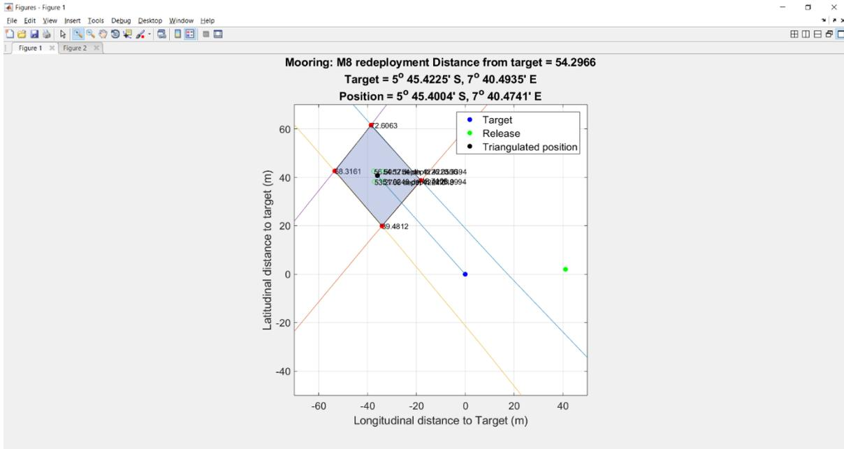
**Figure 8.62.** Target, release and triangulated position of NERC Mooring M8 determined using the centroid of the intersection (shaded blue) of four range circles.
