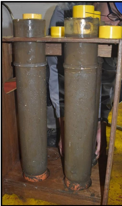
Sub-sampling trigger cores (yellow) that are carefully pushed into the multi-corer tubes.
