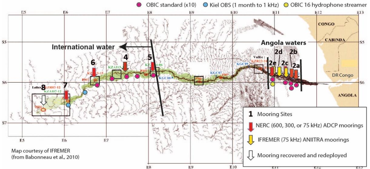
**Figure 1.1:** Map of the Congo Canyon, showing locations of the project’s ADCP-moorings (arrows), Ocean Bottom Seismometers and 16-hydrophone array (circles). The map shows how moorings are located within two sets. The first set of moorings (2a-d) are in Angolan territorial waters in the upper canyon. The second set of moorings (4, 5, 6, 7 and 8) are situated within deeper international waters.
