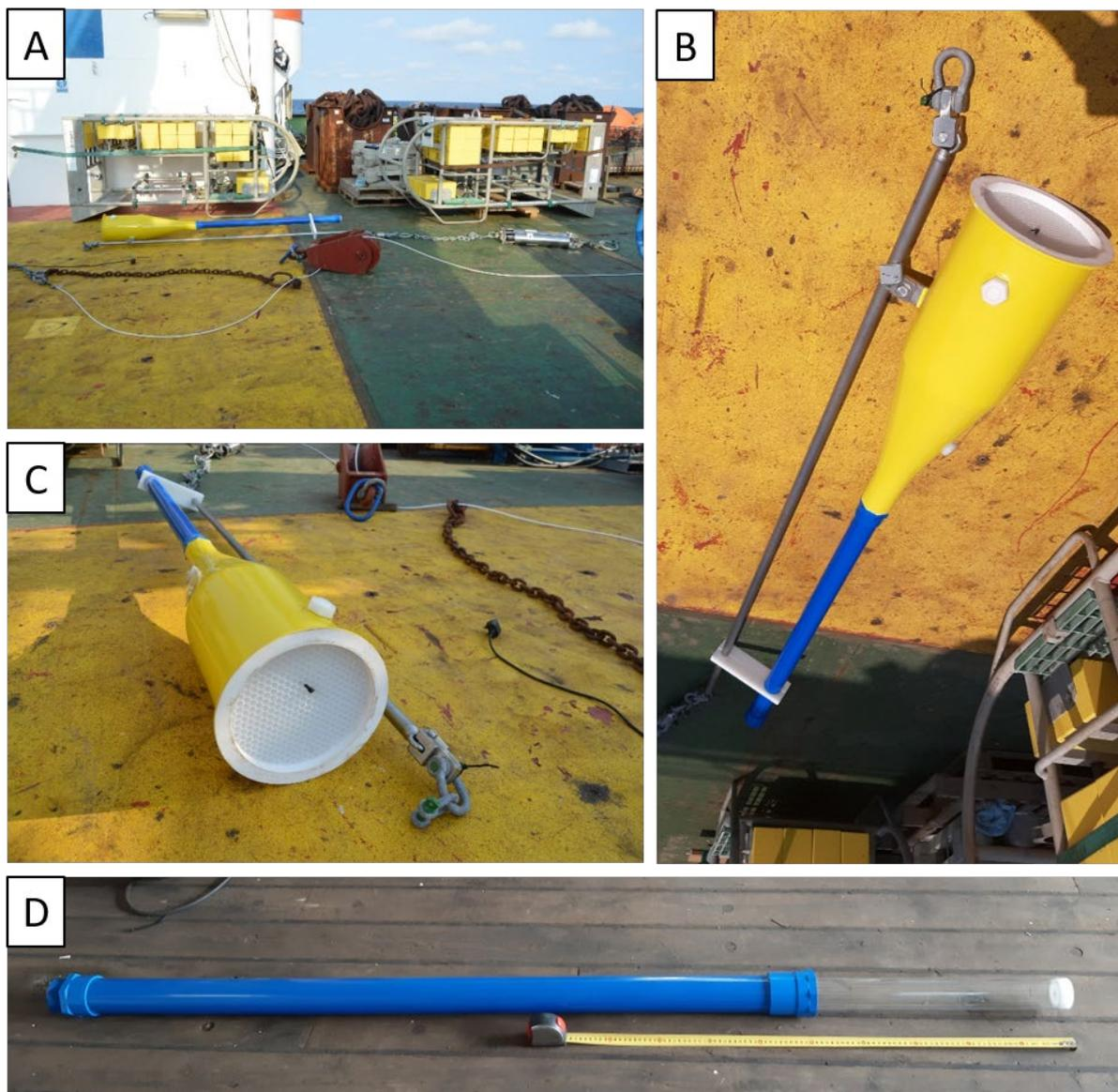
**Figure 8.18:** A) sediment trap on deck showing the acoustic releases just below the trap; B) Sediment trap and metal pole attached; C) top view of sediment trap showing mesh at the top of the funnel; D) clear plastic liner tube within the main tube.
