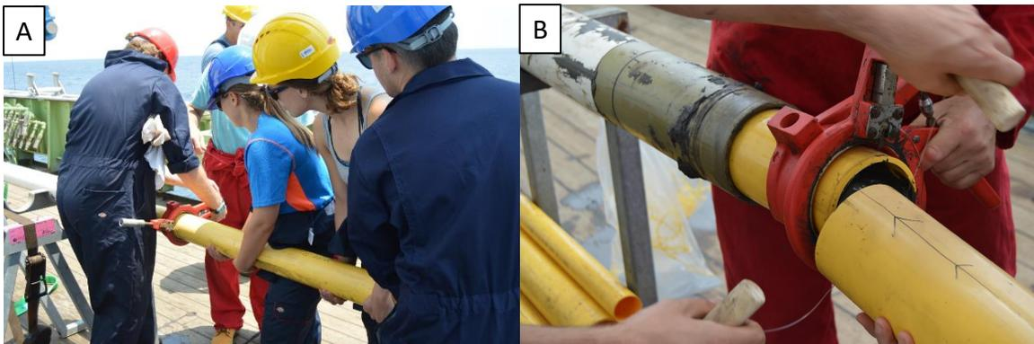
**Figure 8.73.** Cutting of core into 1.5 m sections, and use of a cheese wire.
