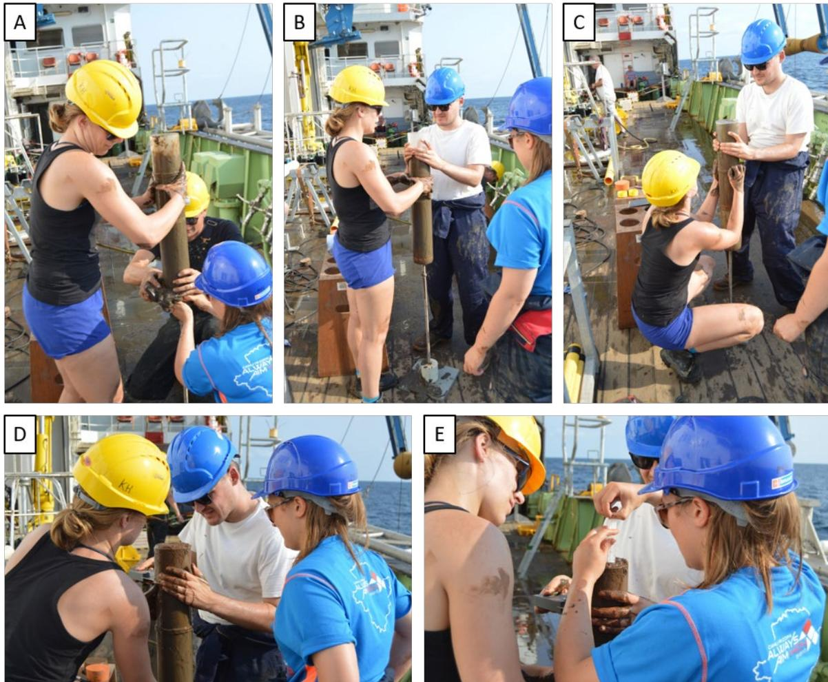
**Figure 8.80:** Photos of the method for sub-sampling the multi-core for EPS and clay: A) the multi-core is quickly slid onto the core pusher; B) the 10 cm-high ring is placed on top of the multi-core; C) the multi-core is pulled down and sediment enters the ring; D) a core cutter is pushed through the gap between the top of the multi-core and the ring; E) syringe is pushed into the top of the 10 cm slice of sediment.
