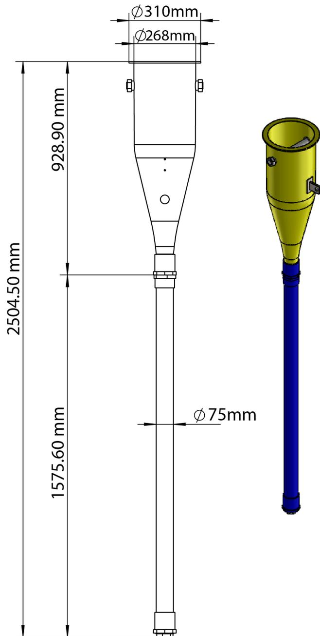
Figure 8.19: Technical drawing of sediment trap. From Hangzhou Sea & Stream Technology Co., Ltd.
