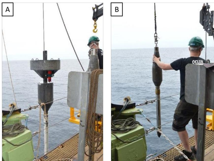
**Figure 8.69.** Left: Piston corer at sea surface, Right: Trigger core
