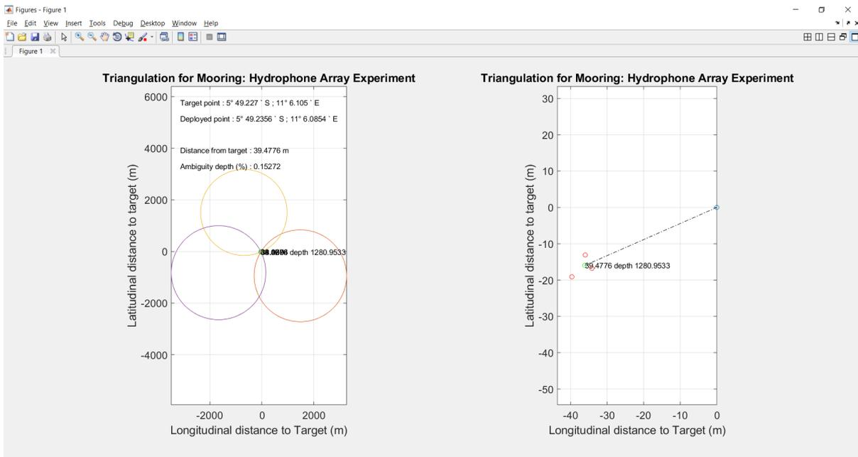
**Figure 8.34.** *Triangulo\_M7.m* output showing target position and triangulated position (left plot) and the distance from the target and the depth of the release determined by the direct trigonometric solution (right plot) for the hydrophone experiment mooring.
