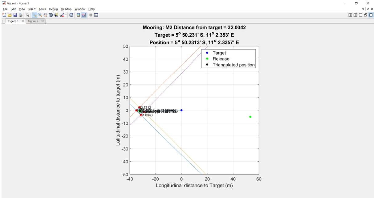
**Figure 8.53.** Target, release and triangulated position of NERC Mooring M2 determined using the centroid of the intersection (shaded blue) of four range circles.
