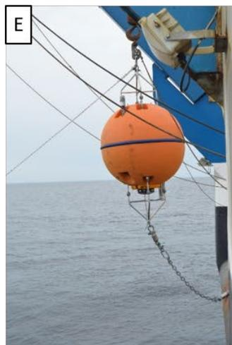
**Figure 8.21:** Mooring deployment. A) and E) ADCP and acoustic releases and lifted, and B) placed in the water. C) Wire is let out, and ADCP buoy and acoustic release trail behind the boat. D) When boat is nearly on target, the anchor is deployed into the water. When the boat is on target the anchor is released. The determination of targets also takes into account cross currents.
