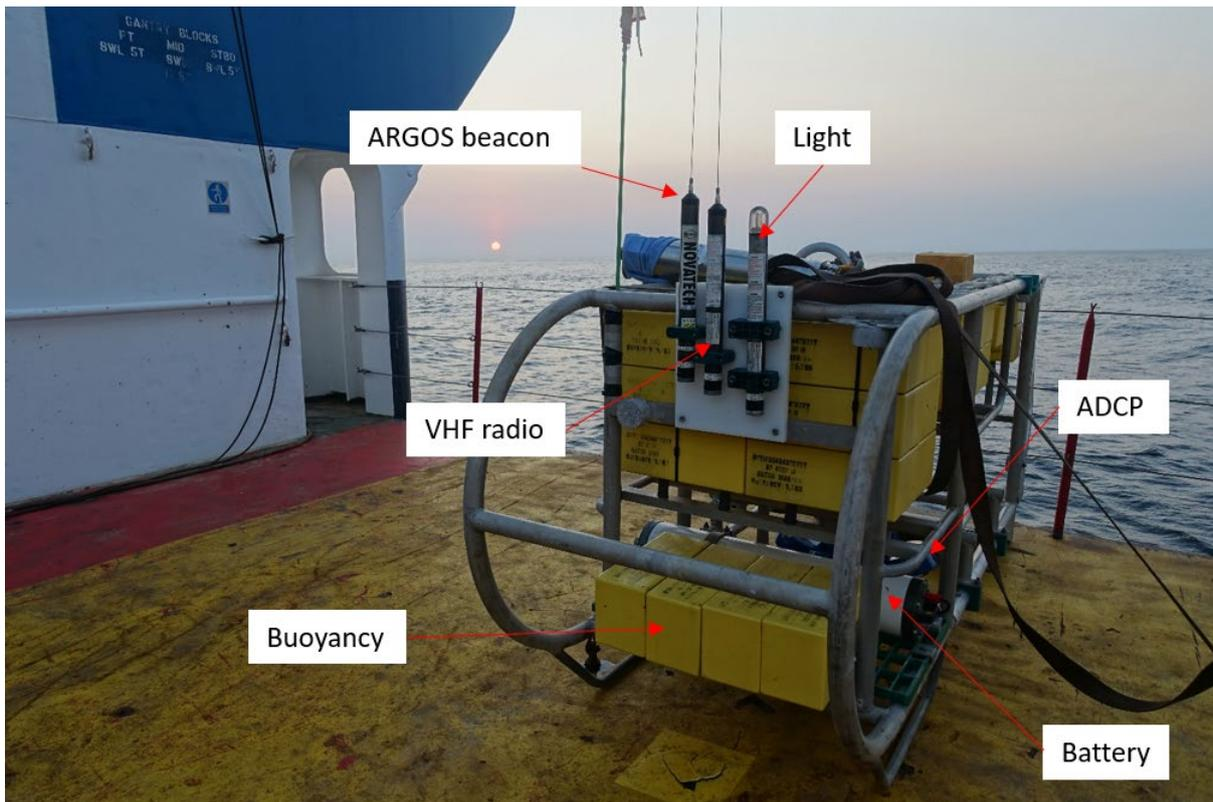
**Figure 8.24.** Main upper part of the Anitra mooring comprising ADCP, battery, buoyancy etc.
