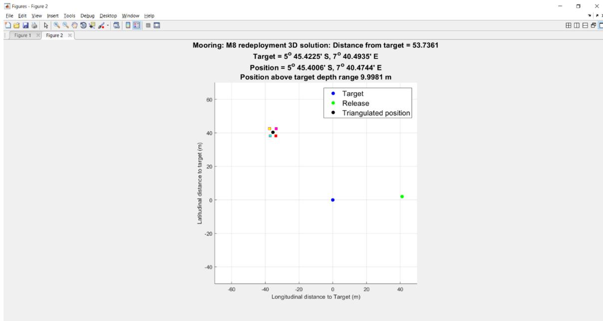
**Figure 8.64.** Target, release, triangulated position and distance from target of the NERC Mooring M8 determined by averaging the four direct trigonometric solutions (squares).
