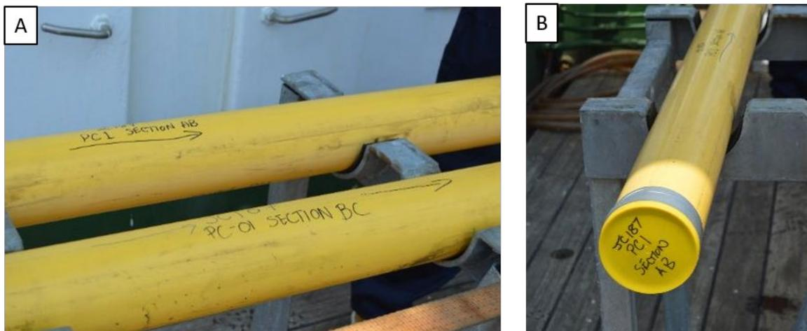
**Figure 8.75.** Labelling on each section (arrow pointing towards the top).
