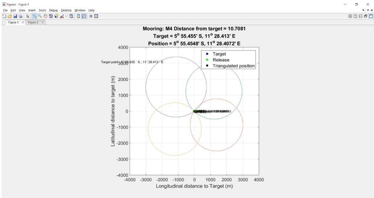
**Figure 8.42.** Zoom out of previous figure showing the full extent of the range circles from the four ranging positions.
