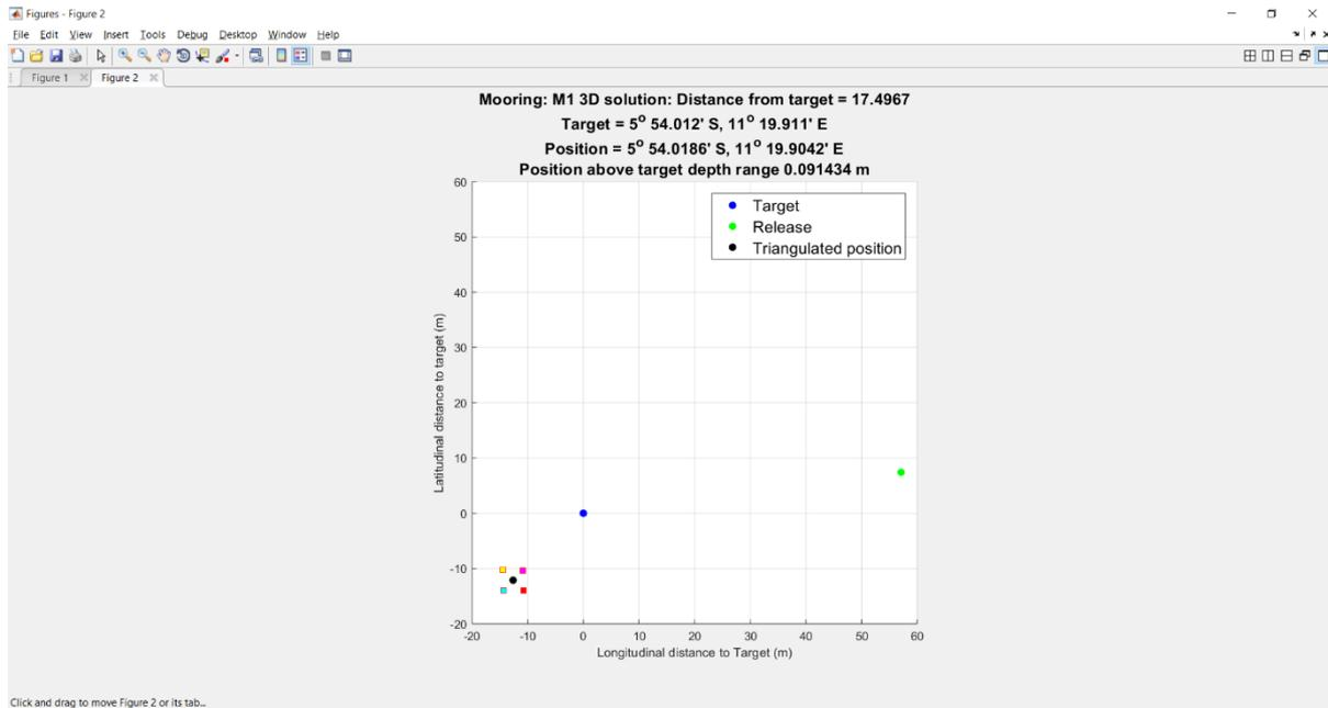
**Fig. 8.40.** Target, release, triangulated position and distance from target of the NERC Mooring M1 determined by averaging the four direct trigonometric solutions (squares).
