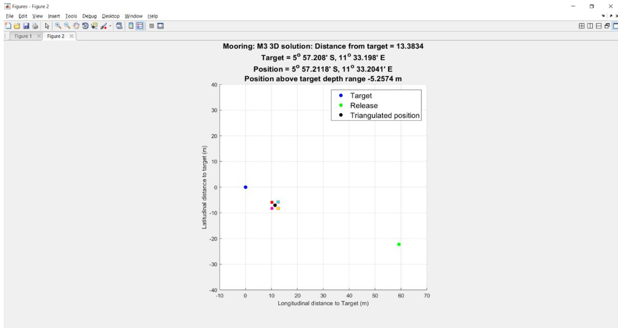
**Figure 8.46.** Target, release, triangulated position and distance from target of the NERC Mooring M3 determined by averaging the four direct trigonometric solutions (squares).
