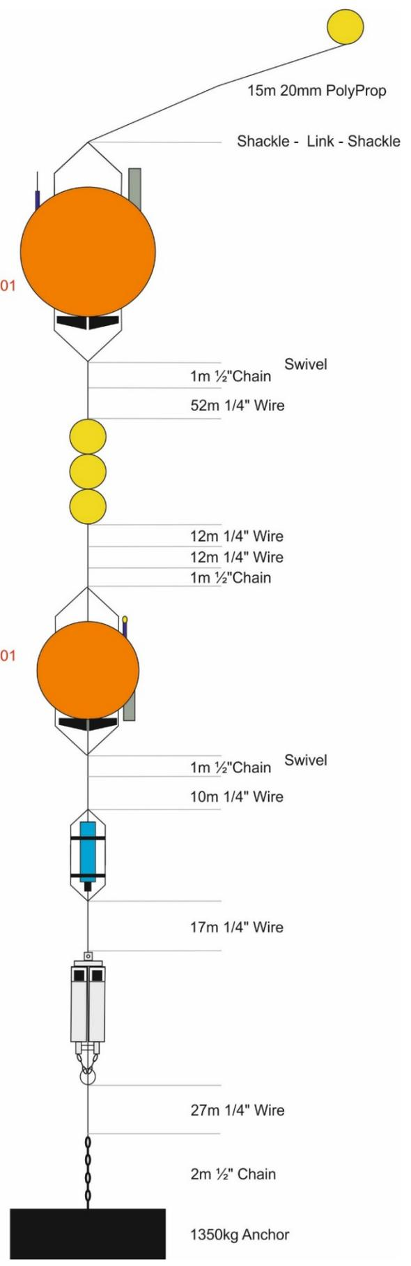
Figure 8.9. Diagram of NERC Mooring-2.
