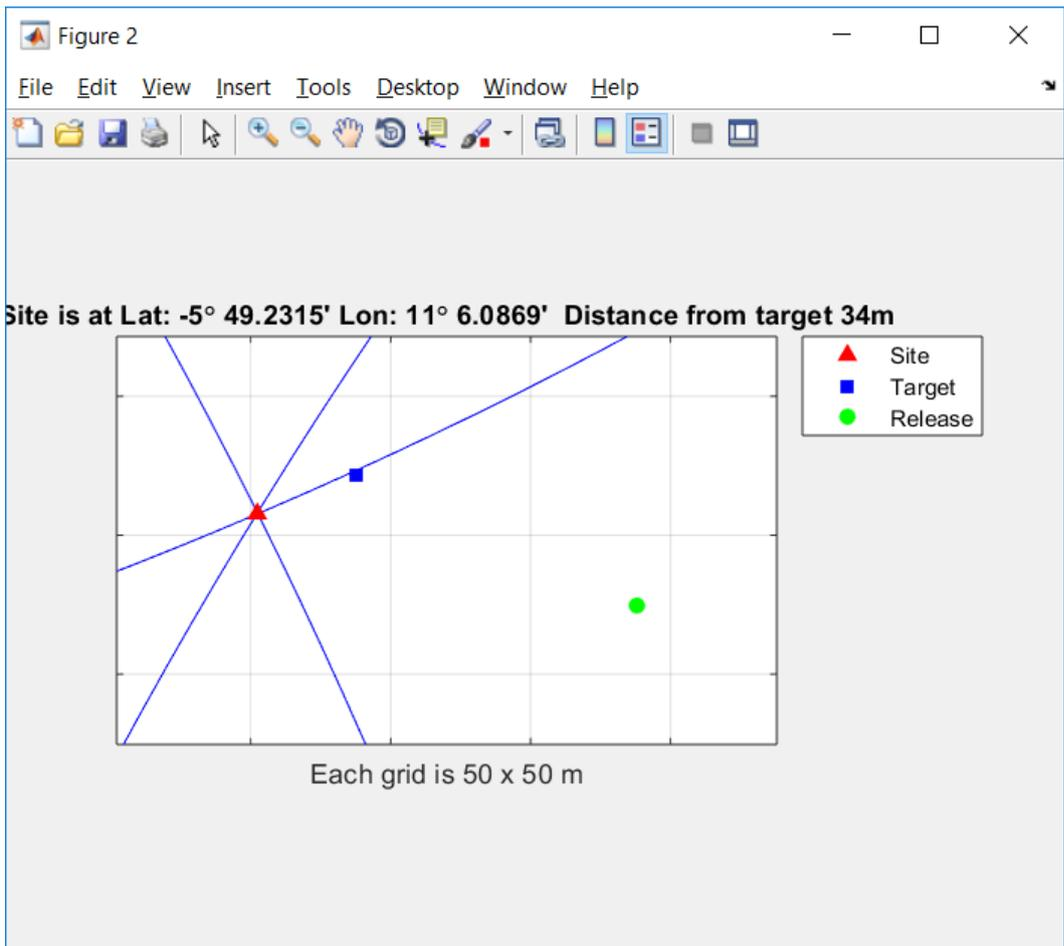
**Figure 8.33.** *Triangulation\_v6.m* output showing target position, release position and triangulated position of the hydrophone array experiment mooring.
