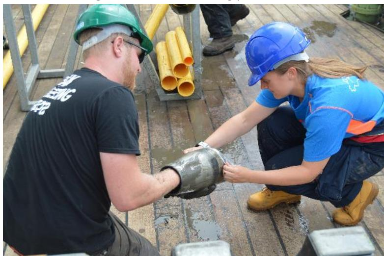
**Figure 8.71.** Collection of the core catcher sample into a plastic bag
