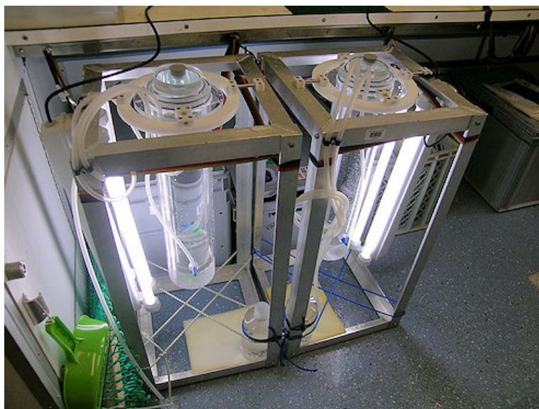
Paul his tubes to determine the settling velocity. The tubes have a cardanic suspension so they are not shaken by the waves and the algae can settle. The TL-lights are there to make the algae grow under controlled light conditions.
