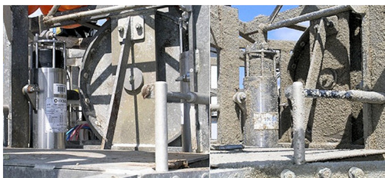
Left: Detail of the clean lander we deployed near the coast at 10 metres water depth. Right: The same detail of the recovered lander that had been under water at this site for 3 weeks. It is completely overgrown with barnacles.
