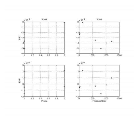
Fig. 5.1.1.1: in-situ salinity calibration. SRC (upper panel) is pre-calibration correction; SDIF (lower panel) is the final error SDIF between bottle (reference) and calbrated CTD salinity after applying a linear correction to conductivity (Müller, 1998); the overall standard deviation of SDIF is less 0.002 on the ISS78 scale.
