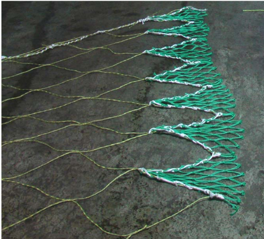
Figure 2: The “shark’s teeth” constructed from 160mm netting.
