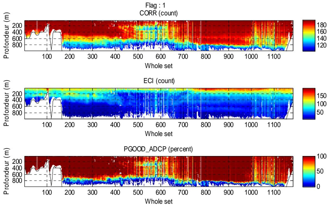
Fig. 21 Correlation, echo intensity and percent good of the processed VMADCP data during the thirty third track between Melchior I. and Cape Horn - Nueva I. in Drake Passage (23-26 March 2013). Noisy data in the middle are due to rough seas.
