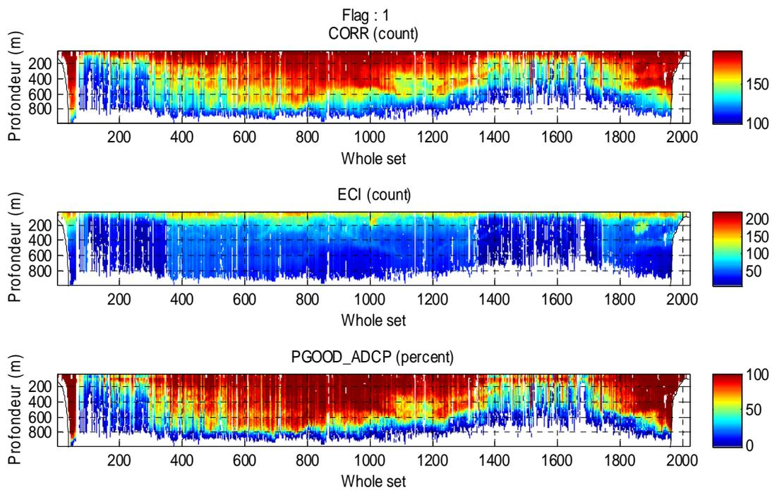
Fig. 15 Correlation, echo intensity and percent good of the processed VMADCP data during the seventeenth track between Nueva I. and Nelson St. in Drake Passage (28-30 January 2013). Noisy and shorter range data are due to rough seas.
