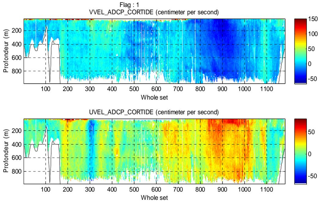
Fig. 22 Processed U and V components of the ADCP during the thirty third track between Melchior I. and Cape Horn - Nueva I. in Drake Passage (23-26 March 2013). Noisy data in the middle are due to rough seas.
