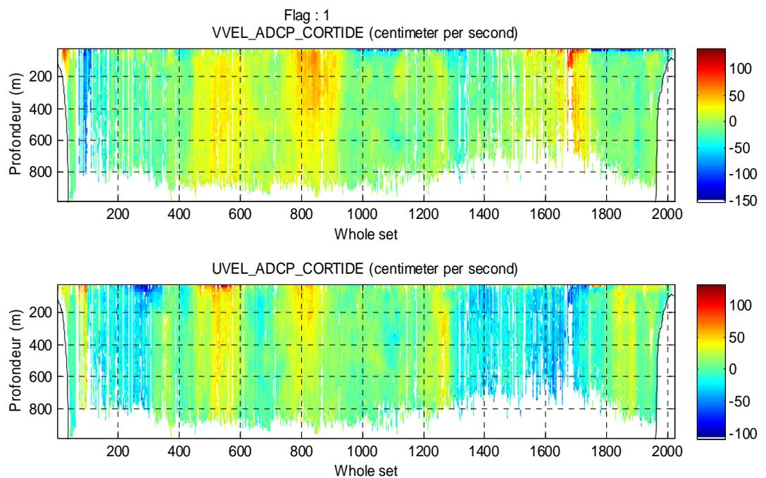
Fig. 16 Processed U and V components of the ADCP during the seventeenth track between Nueva I. and Nelson St. in Drake Passage (28-30 January 2013). Noisy and shorter range data are due to rough seas.
