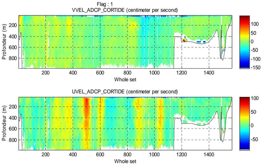
Fig. 20 Processed U and V components of the ADCP during the twenty eighth track between Nueva I. and Argentine I. in Drake Passage (07-09 March 2013).
