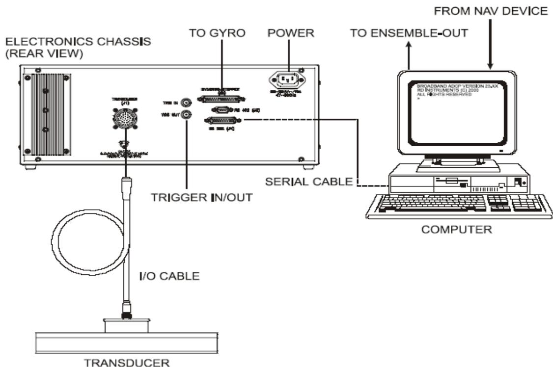
Figure 6 Ocean Surveyor 75 kHz Interface Cable Layout.
