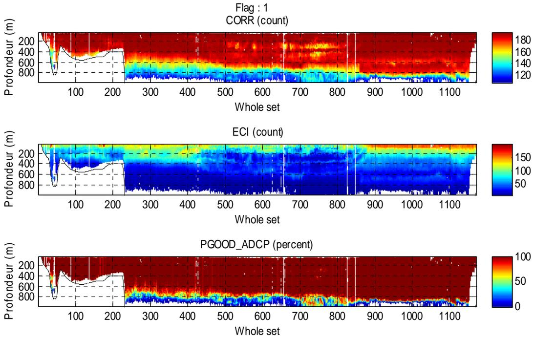
Fig. 17 Correlation, echo intensity and percent good of the processed VMADCP data during the twenty fourth track between Argentine I. and Cape Horn - Nueva I. in Drake Passage (21-24 February 2013).
