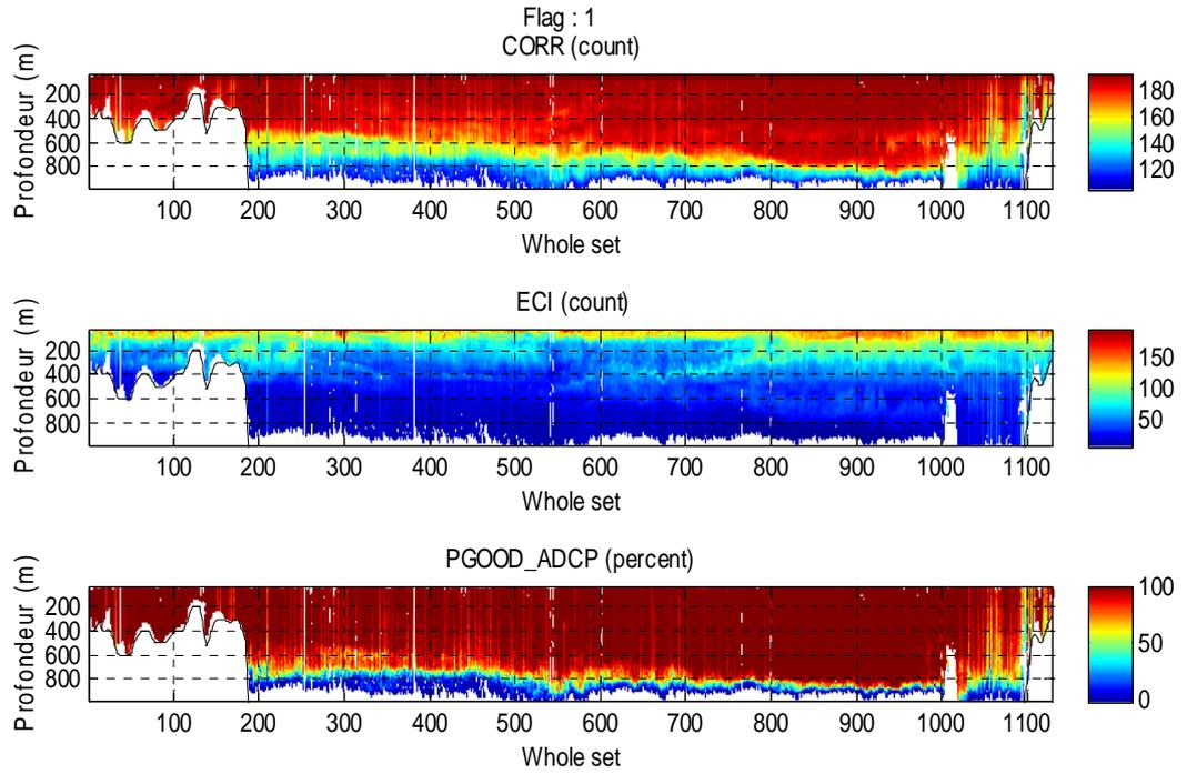
Fig. 13 Correlation, echo intensity and percent good of the processed VMADCP data during the twelfth track between Melchior Is. and Cape Horn - Nueva Is. in Drake Passage (12-15 January 2013).
