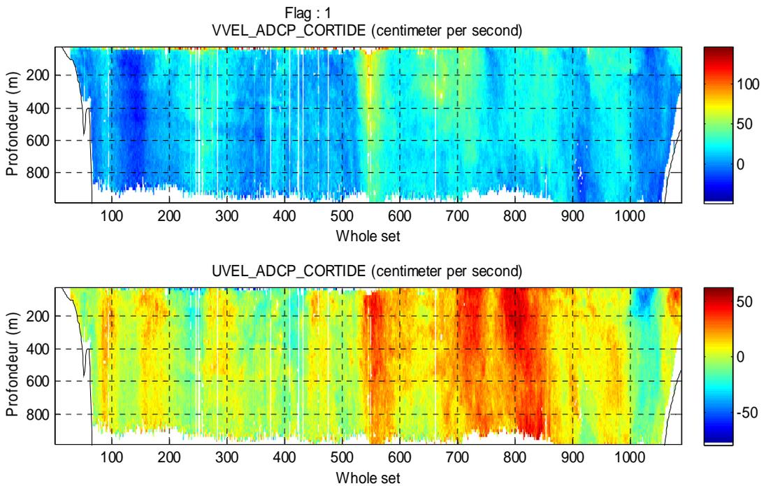
Fig. 12 Processed U and V components of the ADCP during the seventh track between English St. and Cape Horn - Nueva I. in Drake Passage (25-28 December 2012).
