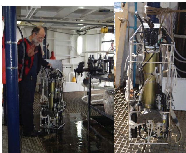
Figure 23. Installation of the CTD on its frame in the vertical position. No Rosette
