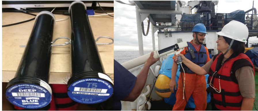
Figure 50. Deep Blue (left) XBT and T5 XBTs.
