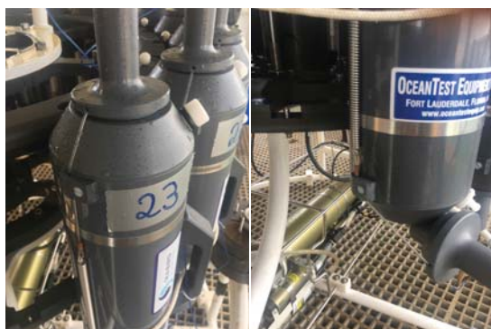
Figure 33. OTE 5l Niskin bottle with external spring mounted in the SBE Rosette.
