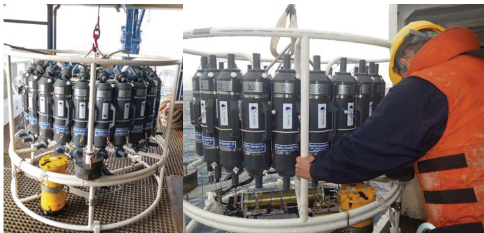
Figure 25. LADCP (the yellow cylinder) mounted in the Rosette.
