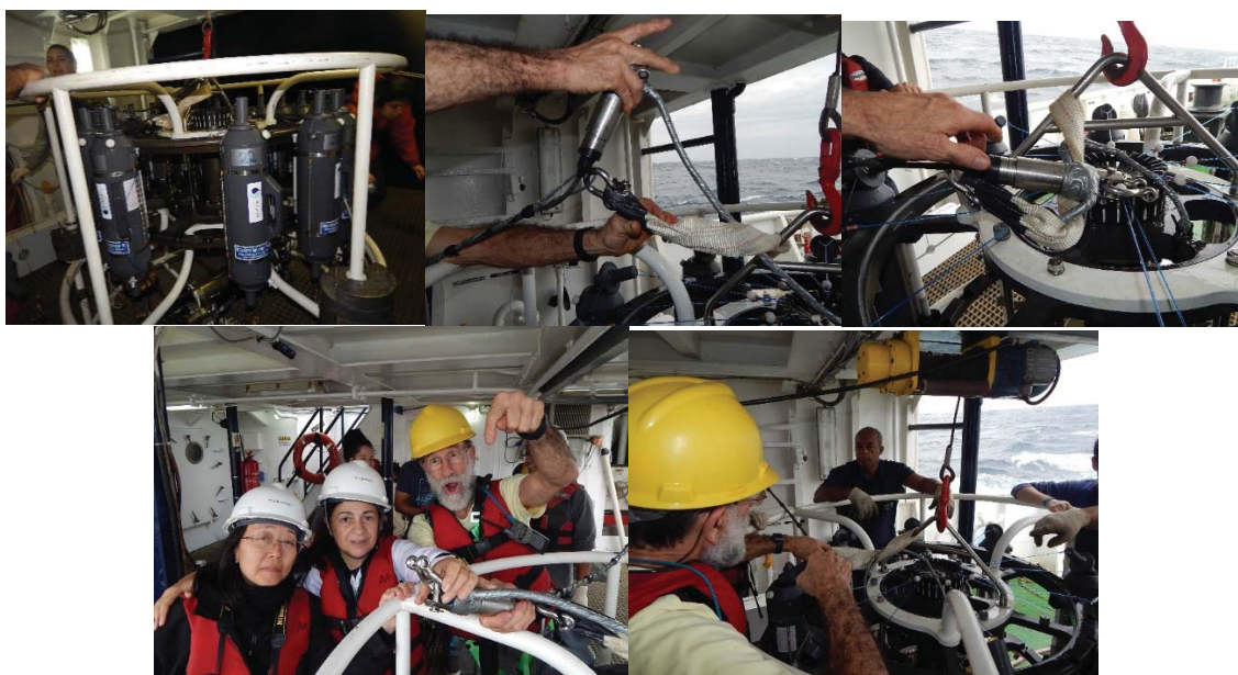
Figure 22. The rosette with 8 bottles and the security belt that maintained the equipment from being lost (the action-shackle opened).
