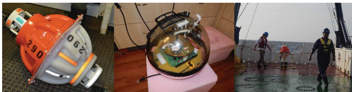
Figure 19. C-PIES SN290 recovered at the site AA (left) and serviced (center). Right: The C-PIES SN409 just before deployment as the new C-PIES AA..
