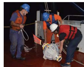
Figure 18. Deployment of PIES SN 187 at site A with the help of Vicentini, Miguel and Pegoraro.
