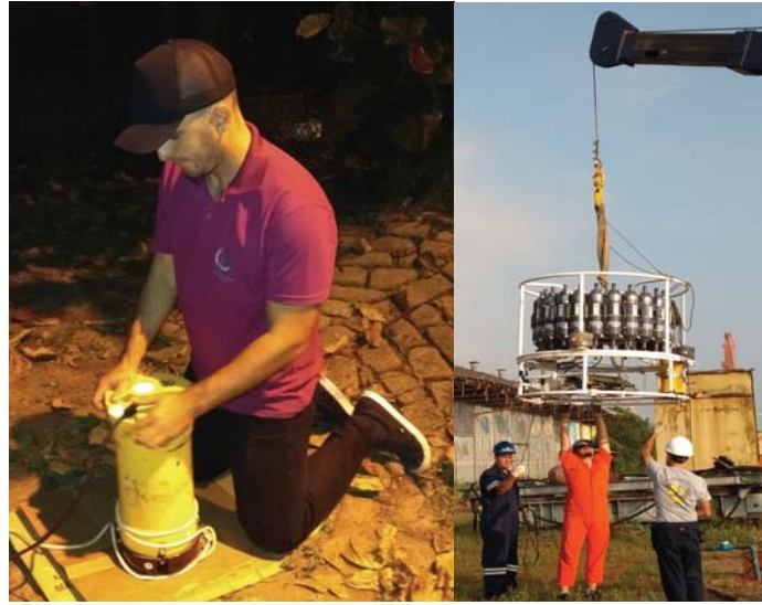
Figure 26: Pre-cruise LADCP gyro test. a) test on deck, before mounting in the CTD frame. b) test after mounting.
