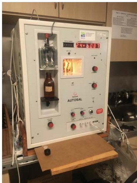
Figure 35. Autosol Guildline 8400B bench salinometer used for on board salinity analysis.
