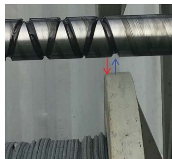
Figure 55. (Top) spooling of the drum showing a smooth of the very first wraps (around 1000 m of cable in). (lower) left and right flange misalignment of the screw groove ends.
