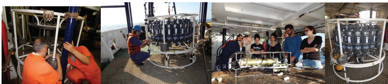
Figure 11. Preparing the rosette and CTD-LADCP to the first test.
