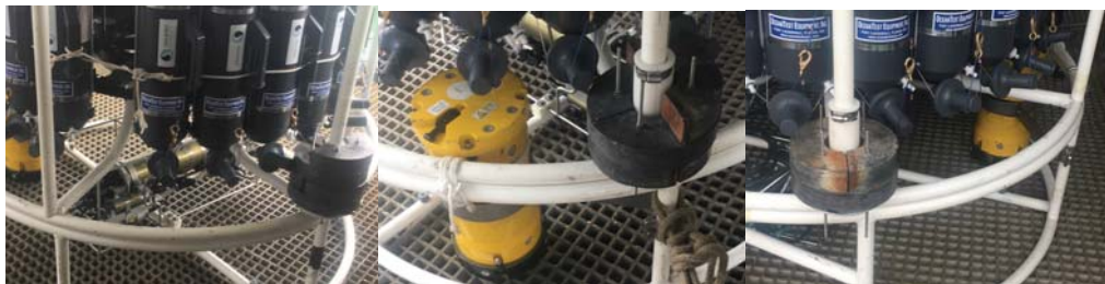
Figure 32. Distribution of weight around the Rosette frame to ballast the CTD/LADCP/Rosette package.
