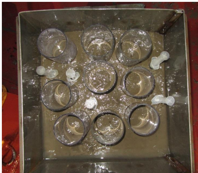
Figure 5.2.5.1. Box core deployment and sediment cores sampling.
