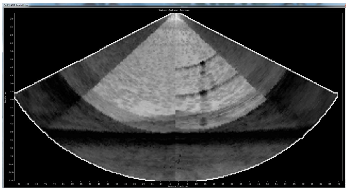
Figure 12. Multibeam imagery identifying orientation and instrument depths (screenshot courtesy of ArcticNet multibeam processing team)
