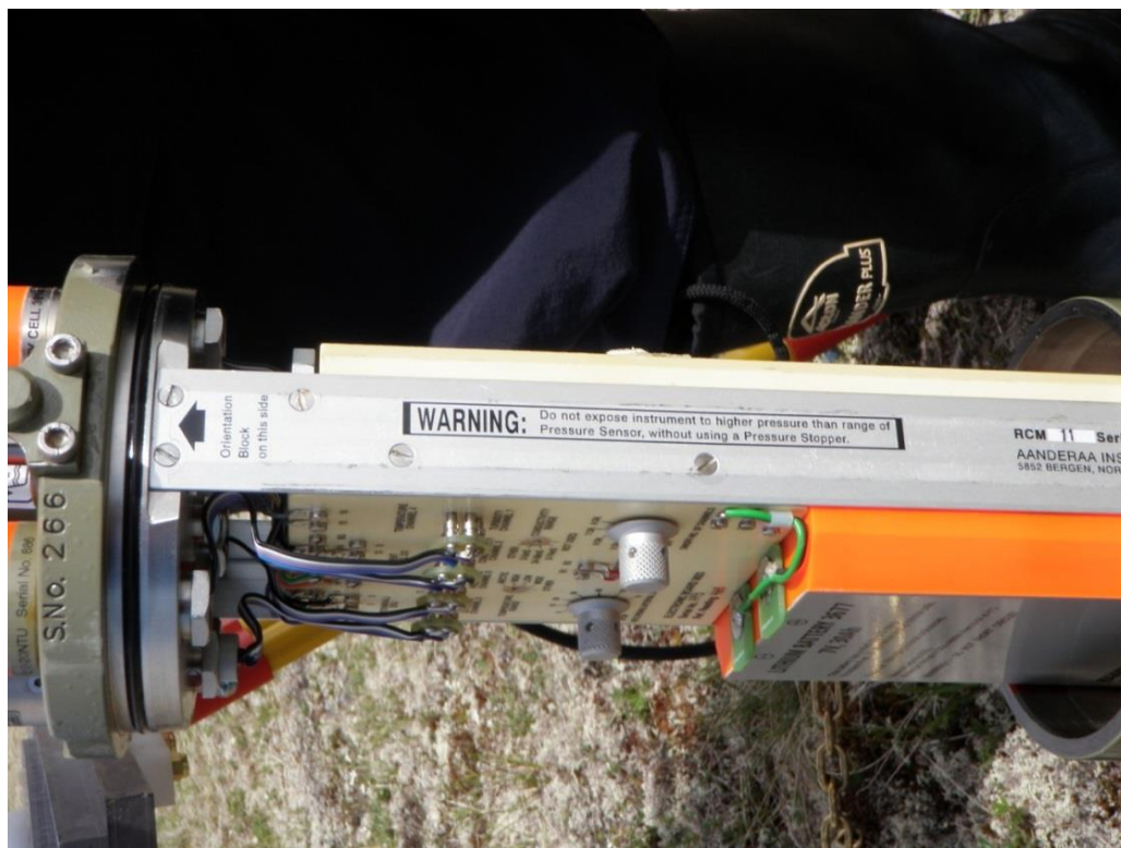
Figure 4. Indicating arrow inside an RCM11 points to the unit’s zero heading (beside serial number) (2010)
