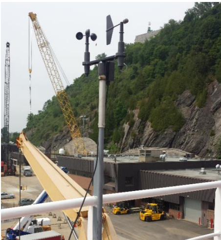
Figure 5.1.10.2: The anemometer, which is attached to the aerosol sampler through CR10 datalogger.
