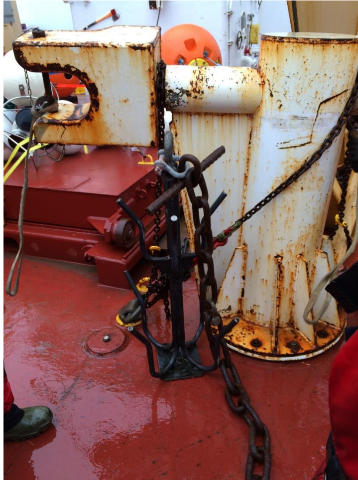
Figure 9. ArcticNet Drugging Anchor for BS1-14
