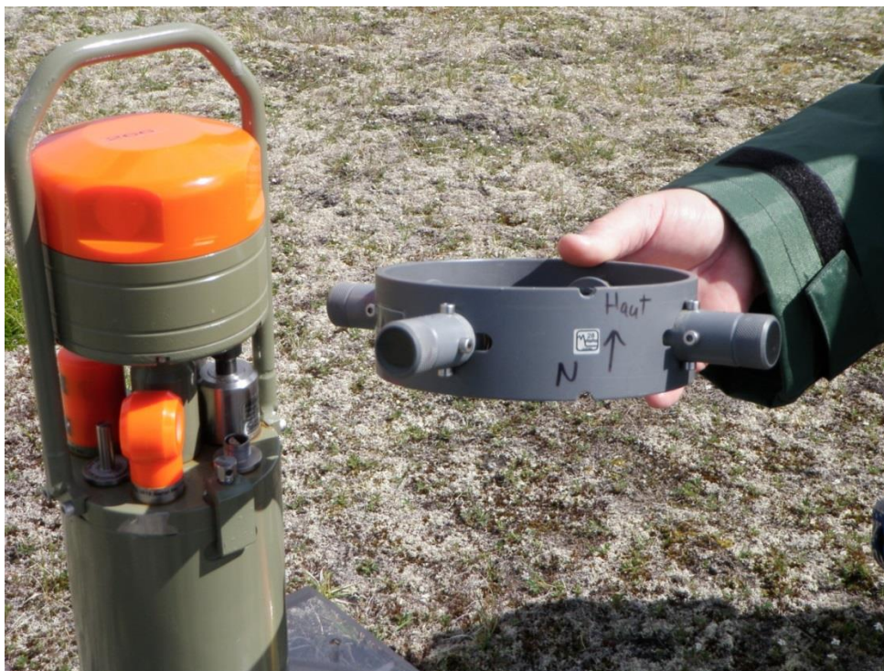
Figure 6. Aanderaa RCM current simulator transducers cover for instrument sensor testing purposes (2010)
