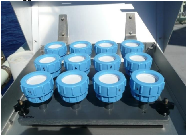
Figure 5.1.10.3: The PVC adapter plate that holds 12 – 47mm filter holders (courtesy of Bill Landing)
