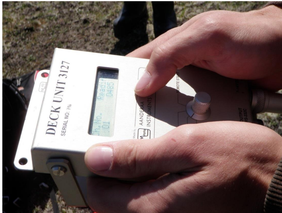
Figure 5. Aanderaa RCM Deck Unit 3127 for communicating to the RCM7/11 in real-time (2010)
