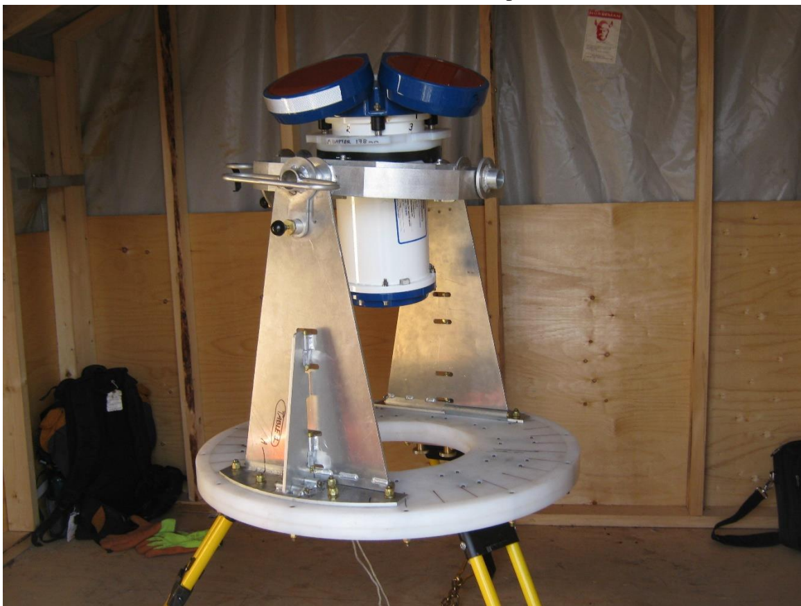
Figure 3. Tilt and rotate calibration jig / table as utilized in Inuvik, NWT
