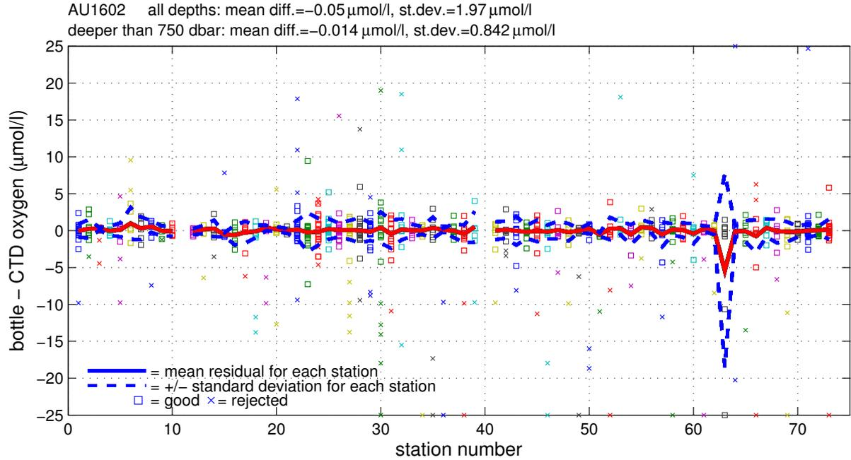
**Figure 5:** Dissolved oxygen residual ( $o_{\text{btl}} - o_{\text{cal}}$ ) versus station number for cruise au1602. The solid line follows the mean residual for each station; the broken lines are  $\pm$  the standard deviation of the residuals for each station.  $o_{\text{cal}}$ =calibrated downcast CTD dissolved oxygen;  $o_{\text{btl}}$ =Niskin bottle dissolved oxygen value.
