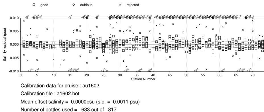
**Figure 3:** Salinity residual ( $s_{btl} - s_{cal}$ ) versus station number for cruise au1602. The solid line is the mean of all the residuals; the broken lines are  $\pm$  the standard deviation of all the residuals.  $s_{cal}$  = calibrated CTD salinity;  $s_{btl}$  = Niskin bottle salinity value.
