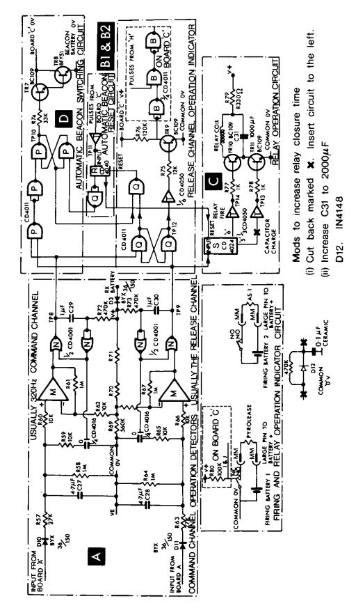
Fig 3: RL81 RELAY BOARD (MODIFIED) 12/11/84
