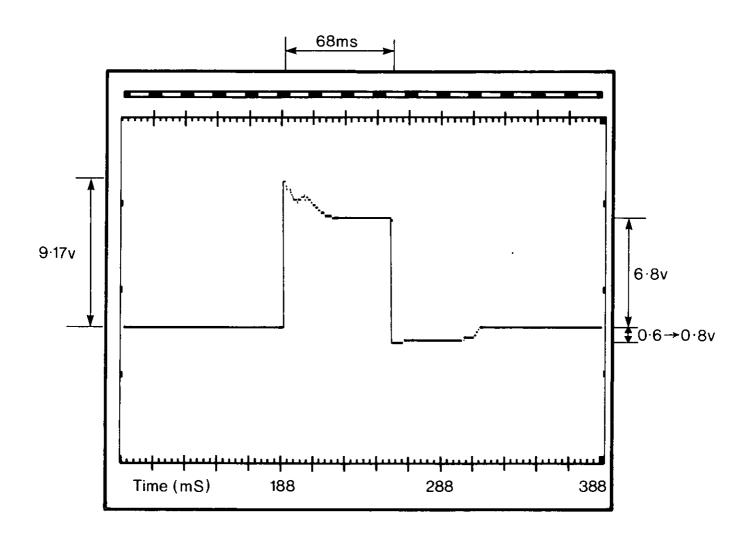
Fig 2: AUTO-RETRACTOR TYPICAL FIRING CURVE
