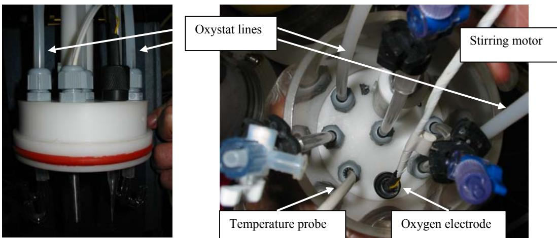
**Figure 2.** Core top seal, side view.
