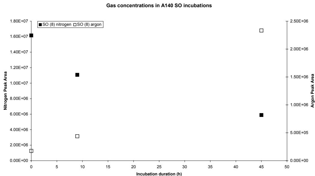
**Figure 3:** Nitrogen and argon peak areas vs time (h) during a shipboard sediment incubation at site A140.
