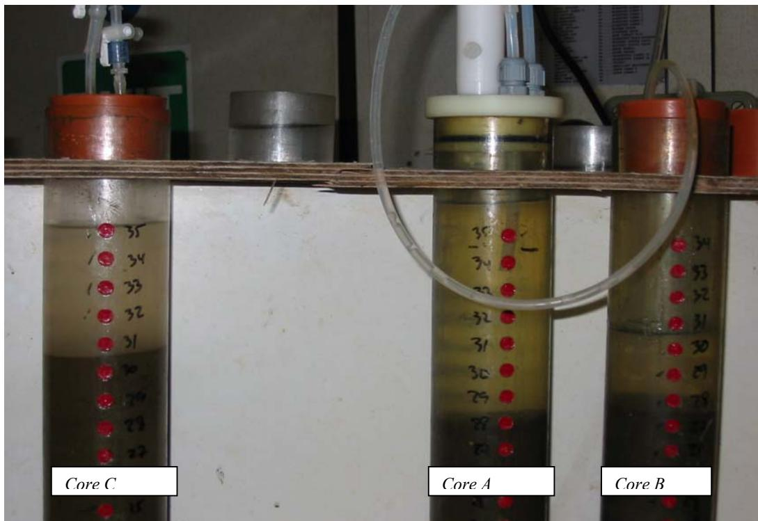
**Figure 2.** Acetylene block cores
