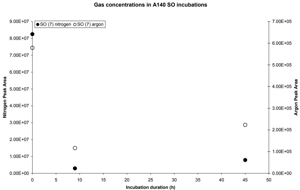
**Figure 2:** Nitrogen and argon peak areas vs time (h) during a shipboard sediment incubation at site A140.
