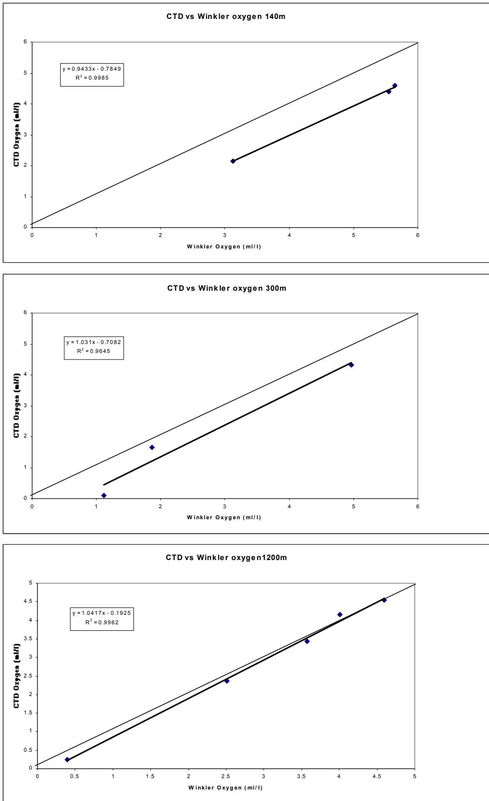
**Figure 1:** Comparison of CTD probe and Winkler titration oxygen results for CD146 water column profiles.
