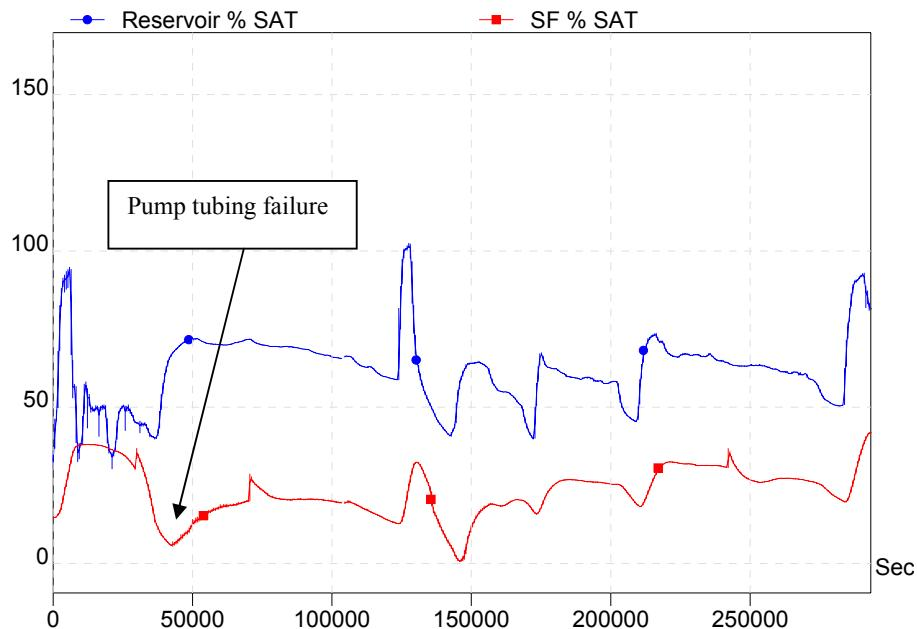
**Figure 6. CD146 A300 Benthic Flux Incubation.** Note marked decrease in dissolved oxygen due to pump tubing failure at point indicated in figure.
