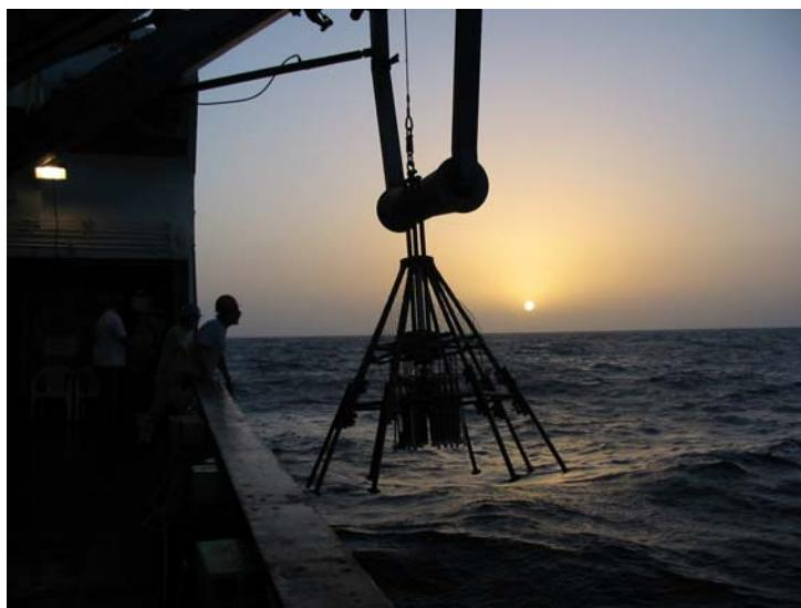
**Fig. 1.** Multicorer deployment from the starboard gantry at sunset.
