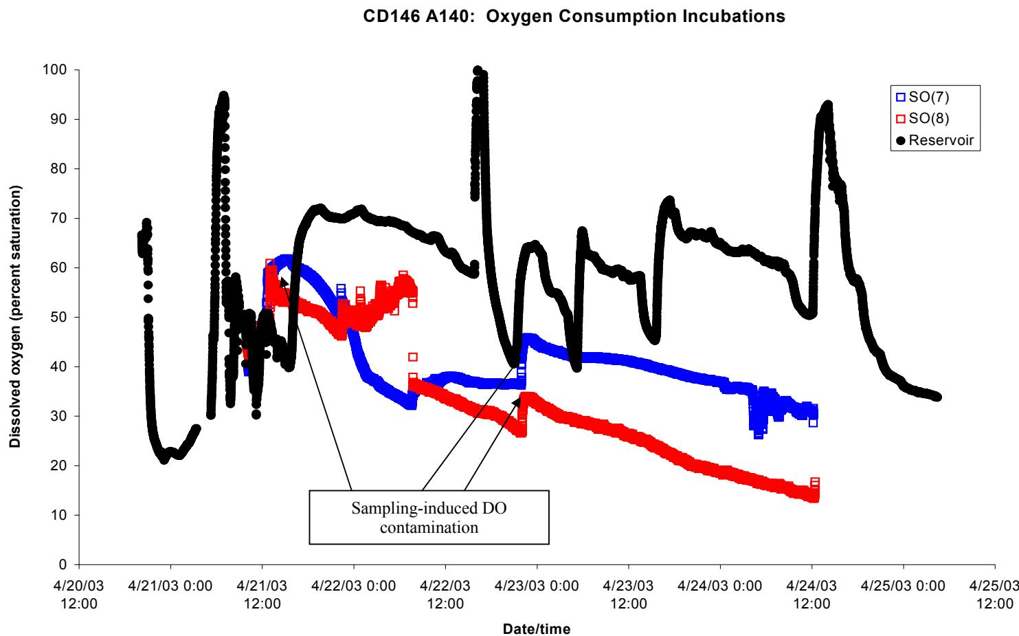
**Figure 4.** CD146 Oxygen Consumption Incubations. General decrease in incubation DO is interrupted by sampling-induced contamination, resulting from replacing sampled volume with water that is equilibrated with atmospheric oxygen.
