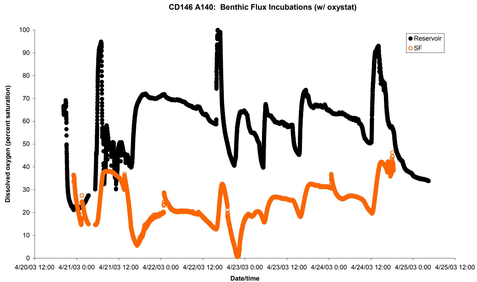
**Figure 3. CD146 A140 Benthic Flux Incubations. Note that SF incubation tracks the changes in dissolved oxygen in the oxystat reservoir.**
