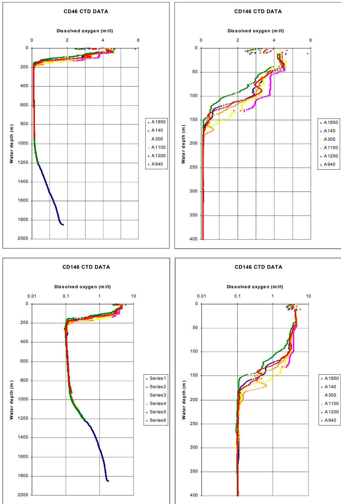
**Figure 4.** CD146 CTD dissolved oxygen concentration profiles (linear and logarithmic scales).
