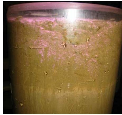
Figure 2. Smearing of beads during sectioning of a 940m megacore/
