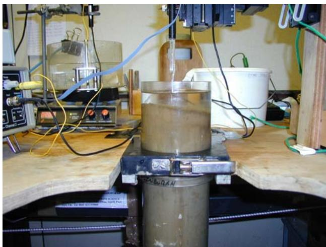
**Figure 1:** Microelectrode profiling of a megacore in the controlled temperature laboratory.
