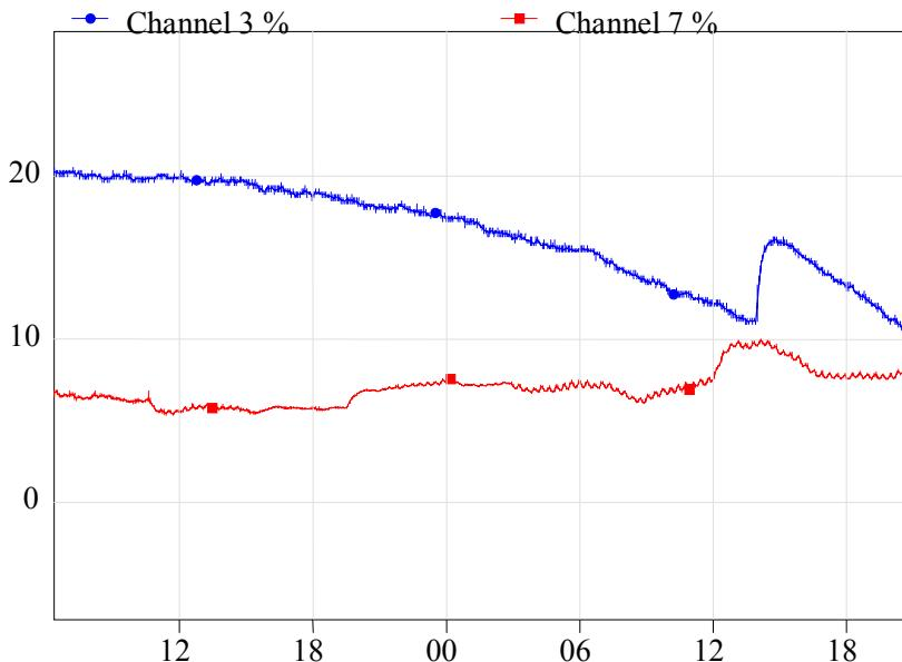
**Figure 5. CD146 A900 Benthic flux (SF) incubation.** Note: dissolved O<sub>2</sub> in SF incubation (Channel 3) remained above oxystat reservoir dissolved O<sub>2</sub> level for first 30 hours of incubation. This was due to coretop comtamination and pump tubing failure.
