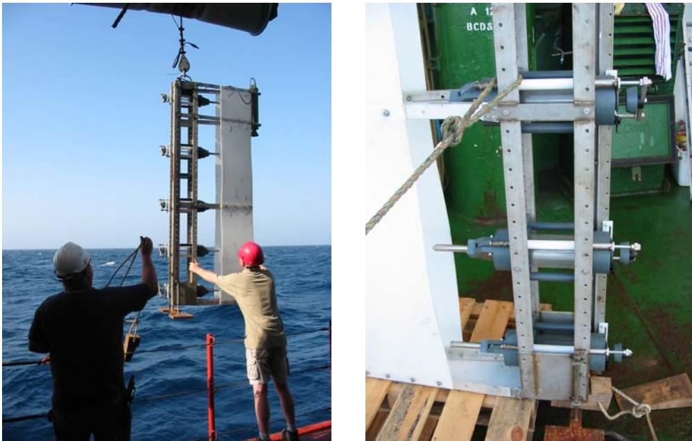
Figure 1: a) BBLS being deployed, showing frame, and b) detail of sample bottles.
