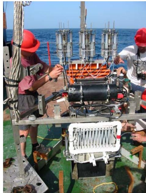
Figure. 3. Elinor system showing (from bottom) the box core and chamber, and the oxystat and syringe sampling systems.
