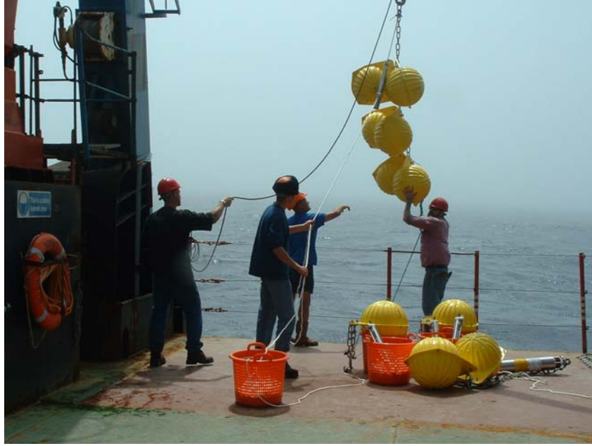
Plates 4 and 5: Deployment of a UKORS mooring.
