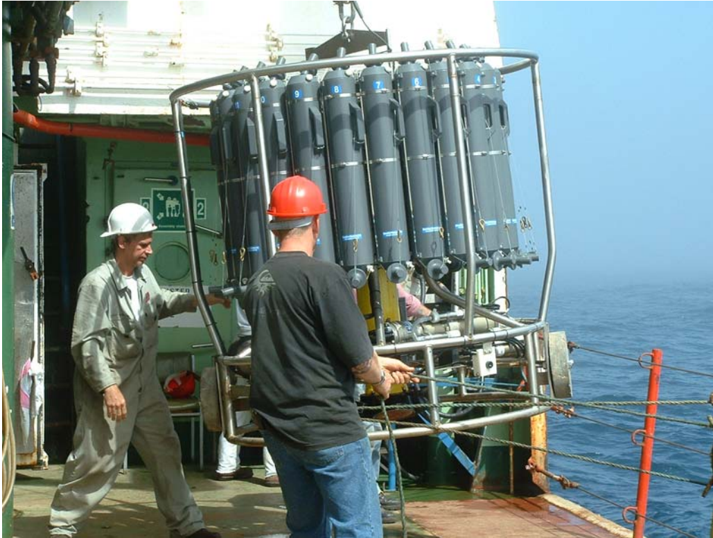
Plates 6 & 7: Deployment of the CTD/LADCP package
