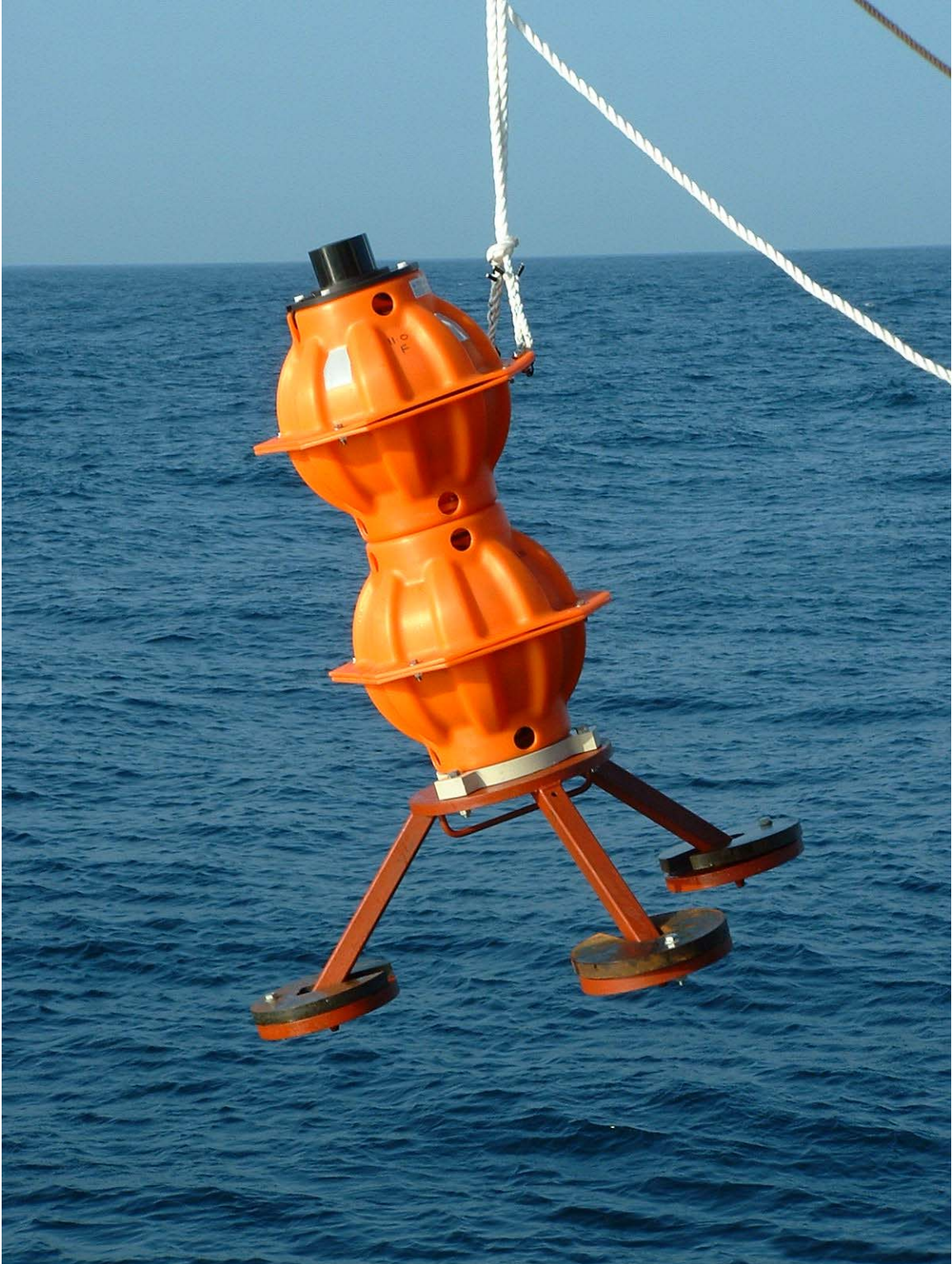
Plate 3: A POL RapidLander BPR being deployed.
