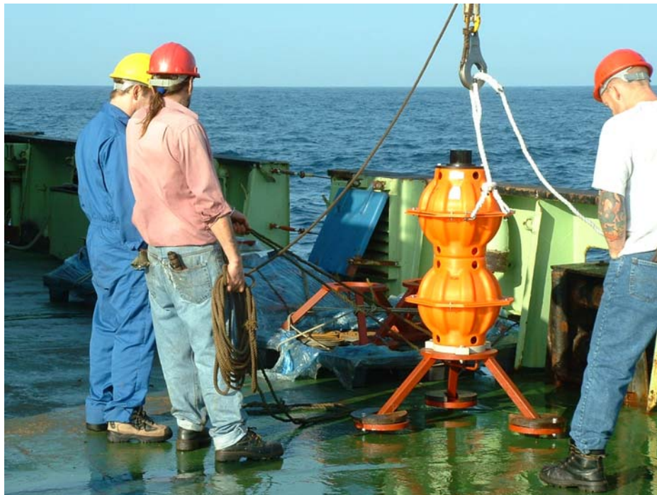
Plate 2: A POL RapidLander BPR being readied for deployment.
