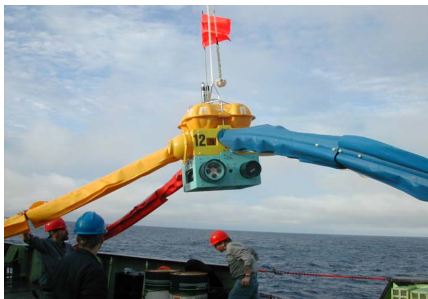
Figure 2.3. Recovering an LC-2000EM. The concrete bottom weight has been jettisoned and left on the sea bed. The electrodes are housed in the ends of the flexible arms.
