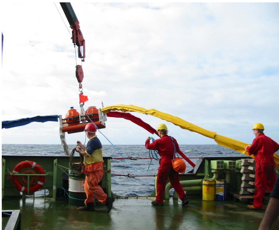
Figure 2.2. Deploying a LEMUR. The sensor electrodes are housed in the ends of the flexible arms. The bottom weight can be seen underneath the instrument frame.
