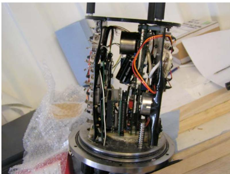
Photograph C.16: MAR4 MMP internal electronics chassis badly distorted, with electronic components broken off boards
