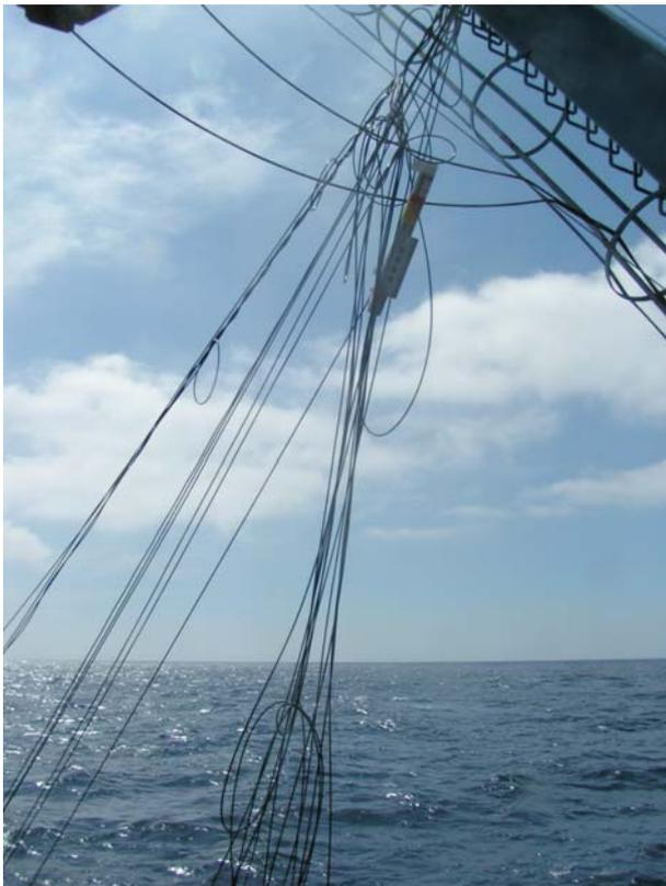
Photograph C.13: Wire wuzzle during EB3 recovery
