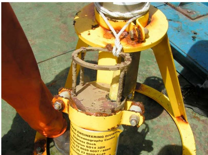
Photograph C.10: Fouling on EBH4 tripod and BPR
