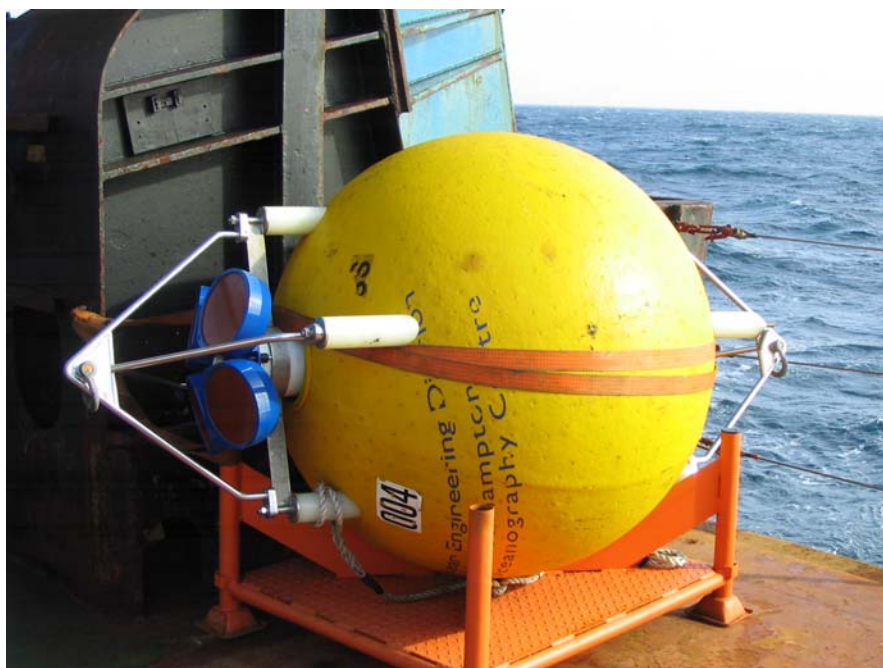
Fig. 10.1 The ADCP located in its buoy.
