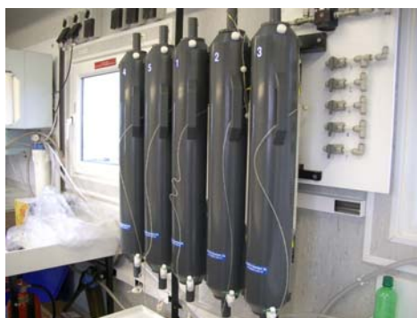
Fig. 15.4: Modified OTE bottles for trace metal work
