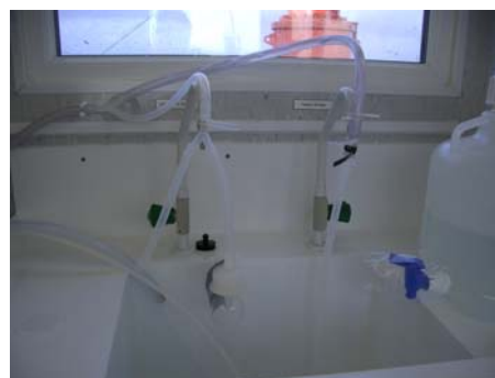
Fig. 15.3: Underway manifold in the clean container
