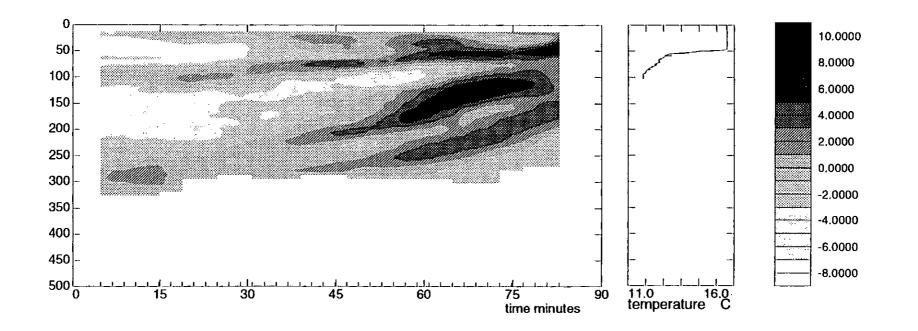
Figure 4. RRS Charles Darwin cruise 72: relative acoustic backscatter from the ADCP showing layers of diel migration in the vicinity of the thermocline.
