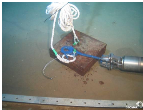
Fig. 4.4.3.1h: Hook-wire-construction for recovering ADCP and anchor weights.
