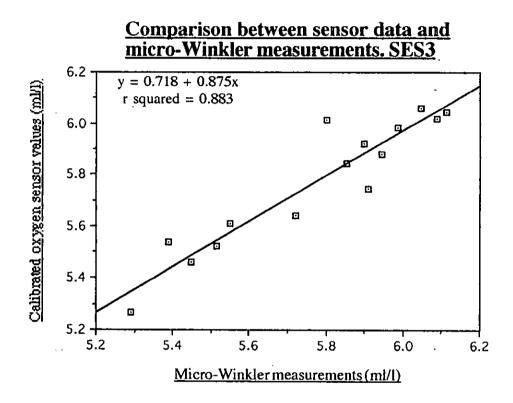
Figure 8. Comparison between sensor data and micro-Winkler measurements. SES3.
